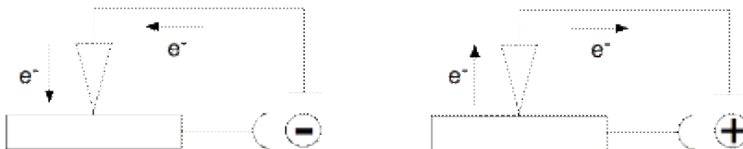
Figure 3-18: Setup used for CSAFM mode. A conductive AFM tip is biased to the sample. For a negative bias (left scheme), the higher is the current signal the lower is the resistivity of the sample. For a positive bias (right scheme) the dependence is opposite.
