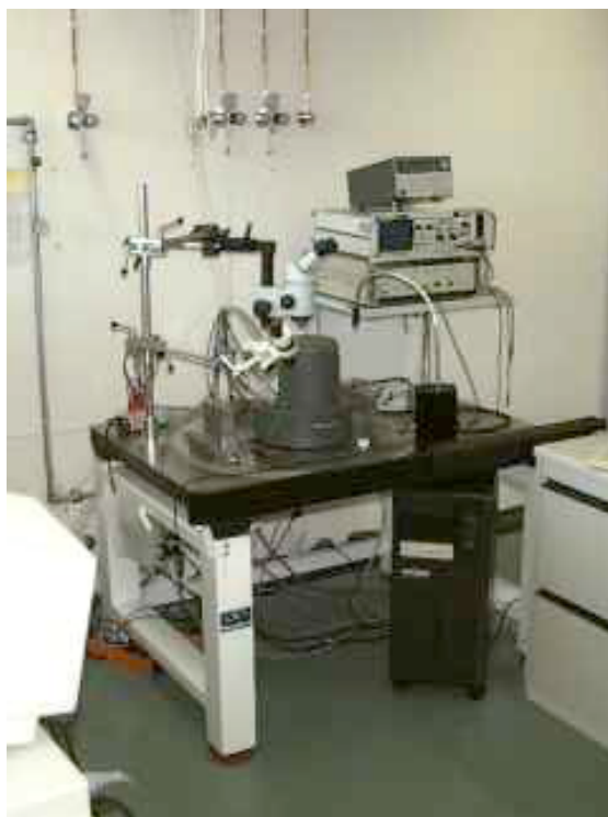
Figure 3-8: Autoprobe CP system (Thermomicroscopes Corp.). A base module, which houses the probe and the scanning unit, sits on a vibration isolated table. The base is connected to the AEM electronic module, the acquisition computer and the potentiostat.
