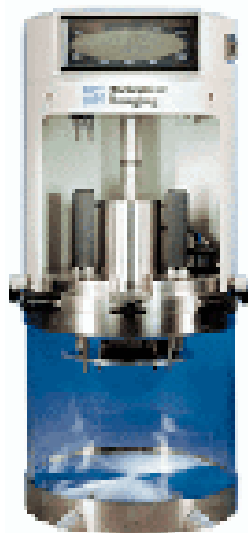
Figure 3-9: PicoSPM scanning unit. The in situ SPM cell is housed in a Pyrex cylinder. Two gaslets, which are visible in the front of the cylinder, enable exchange of the atmosphere. A piezo scanner provides the movement of the probes from the top of the cell.
