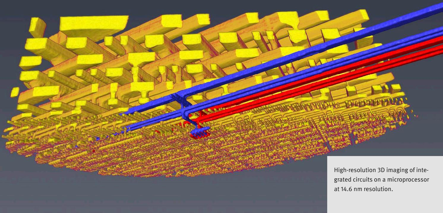
High-resolution 3D imaging of integrated circuits on a microprocessor at 14.6 nm resolution.
