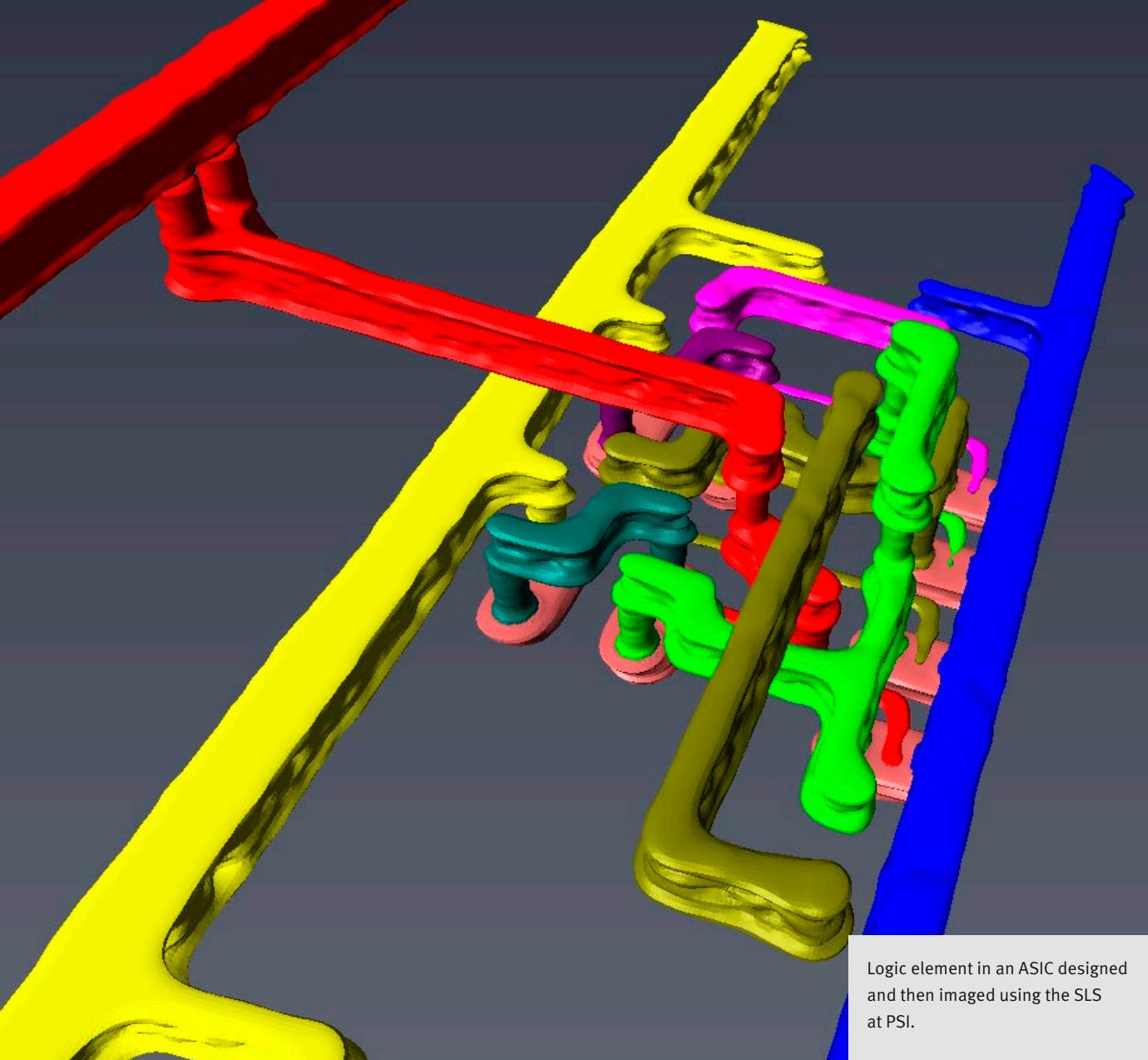
Logic element in an ASIC designed and then imaged using the SLS at PSI.
