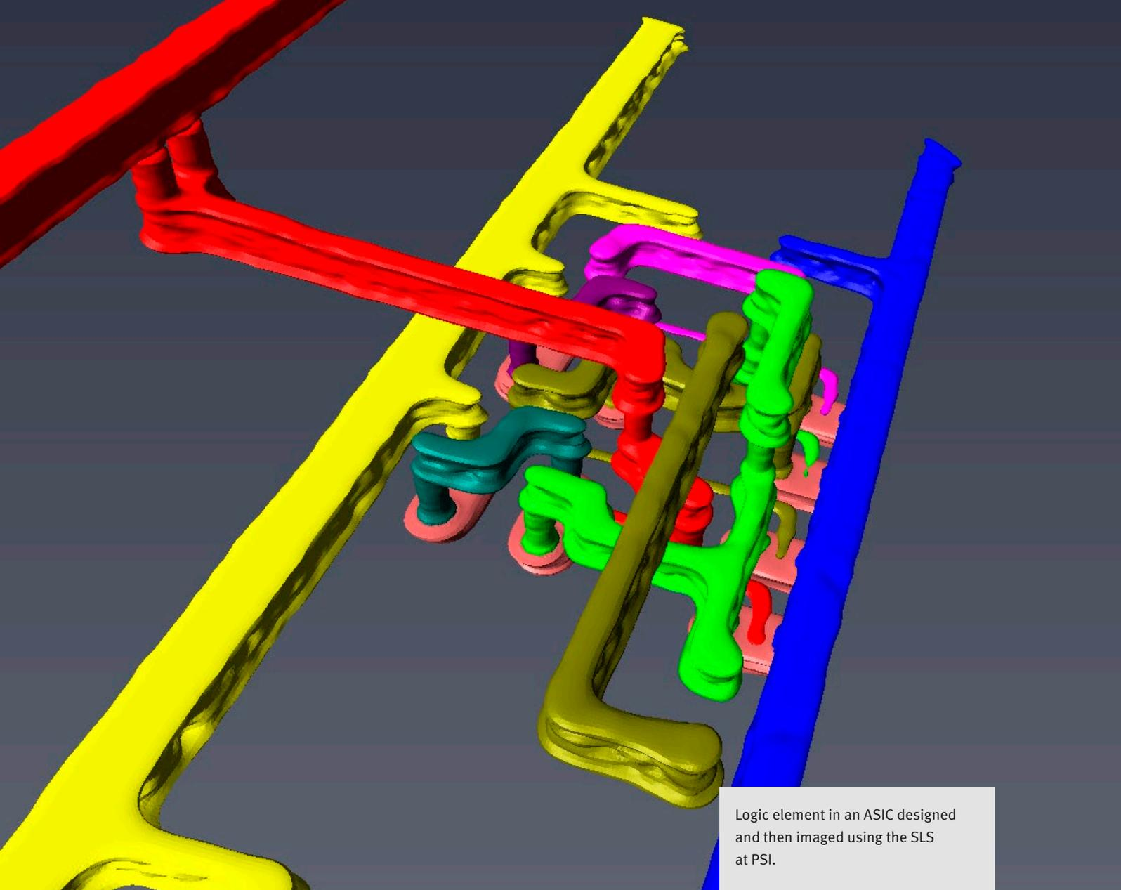
Logic element in an ASIC designed and then imaged using the SLS at PSI.
