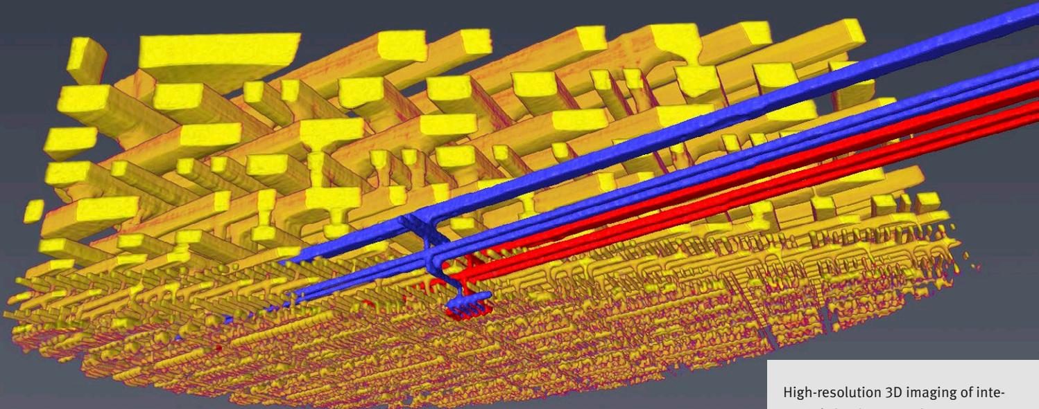
High-resolution 3D imaging of integrated circuits on a microprocessor at 14.6 nm resolution.
