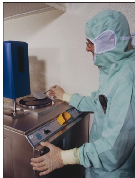
Plasma enhanced chemical vapor deposition system for nitrides and oxides.
