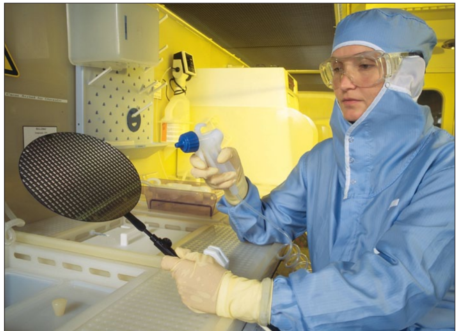
PSI clean room equipped for handling and processing of 200 mm diameter wafers.
