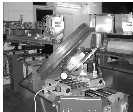
In-situ loading on POLDI, measuring the deformation mechanics of bainitic steels.
