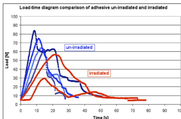
Figure 2: Comparison of unirradiated and irradiated adhesive bonds.
