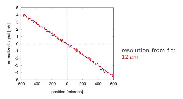
⇒ resolution is good, however, out of phase component shifts measured center position (see also 9P.86)
