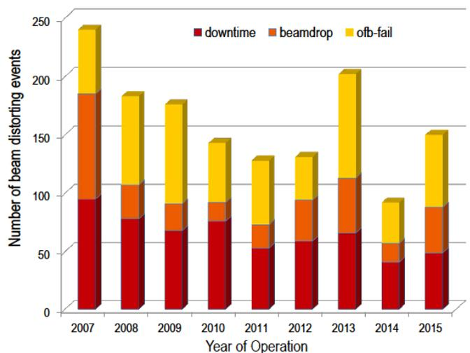
**Figure 5:** Number of beam distorting events of the past years
