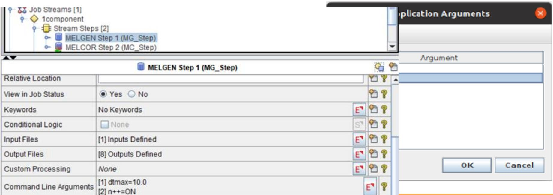
The screenshot displays the MELCOR software interface. On the left, a tree view shows the job structure: Job Streams [1] containing 1 component, which contains Stream Steps [2]. The selected step is MELGEN Step 1 (MG\_Step), with MELCOR Step 2 (MC\_Step) listed below it. The main panel shows the configuration for MELGEN Step 1 (MG\_Step). The 'Command Line Arguments' field is populated with the following text:
