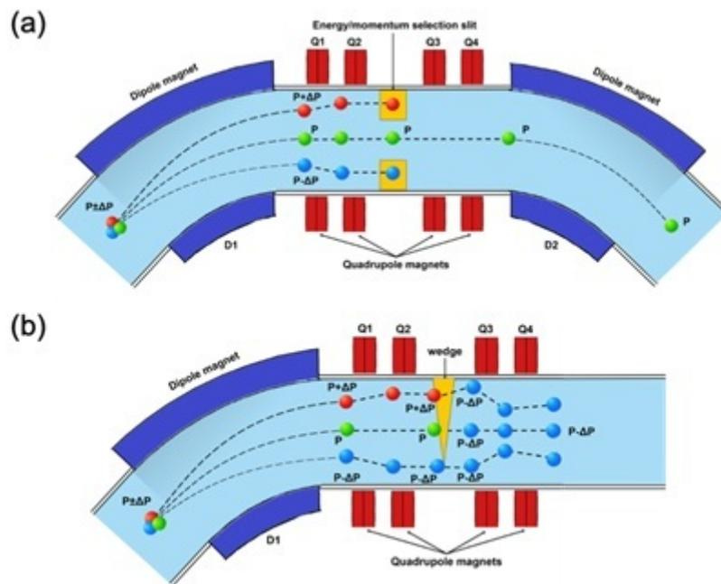
(a) The conventional layout of an ESS features a cross-sectional bending plane with an energy/momentum selection slit
