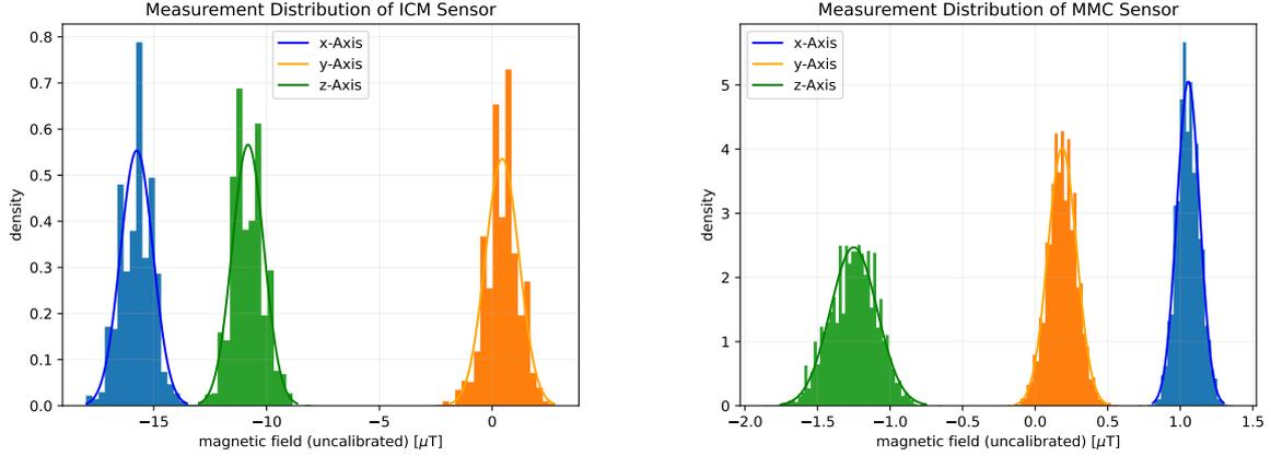
**Figure 9:** Distribution of data during a 30 s measurement in a stable external magnetic field for two randomly chosen sensors together with a Gaussian fit. All six histograms are individually normalized such that the area under the histogram yields 1. The sensors have not been calibrated. *Left:* ICM sensor, 1473 data points, *Right:* MMC sensor, 6572 data points.
