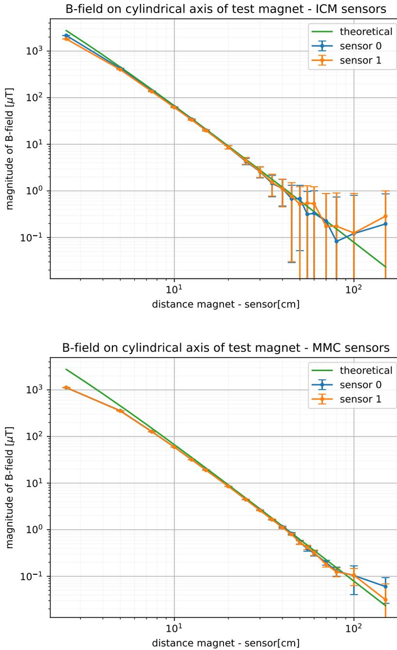
**Figure 8:** These plots show the magnetic field magnitude of the test magnet measured at various distances with the setup depicted in Figure 6 on the right. The errors on the magnitude are calculated from the standard deviation of the 7s reference and raw measurements along each axis using Gaussian error propagation. *Top:* Results for the ICM sensors. *Bottom:* Results for the MMC sensors
