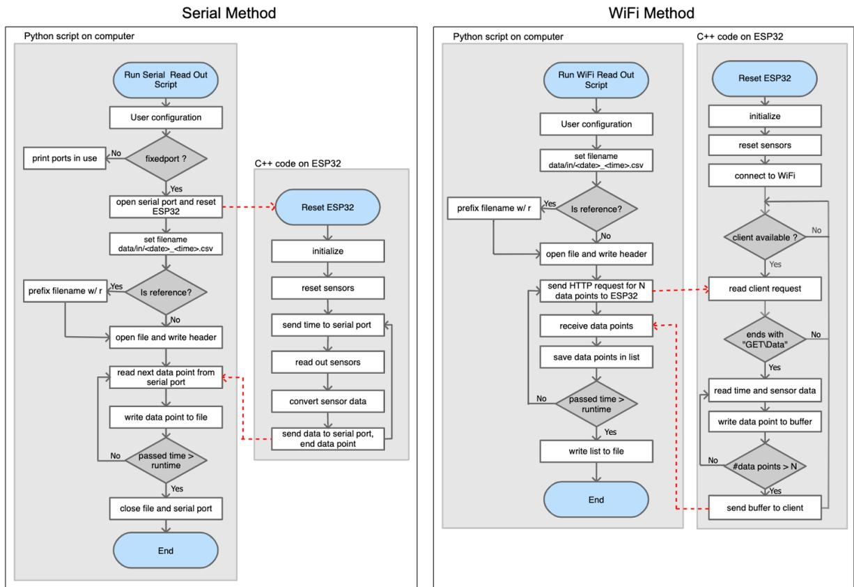
**Figure 4:** Flowcharts of the C++ code (ESP32) and the Python script (external computer) for both communication methods. When running an experiment one can choose between either method but first one has to upload the corresponding code onto the microcontroller, as the ESP32 can only save one program at a time. The red lines indicate communication between the two devices.
