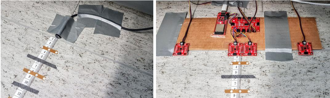
**Figure 6:** *Left:* Setup of the fluxmaster to measure the magnetic field of the test magnet along the black string at various distances. *Right:* Setup of four ICM sensors, the microcontroller and the Mux to test the sensor performance by placing the test magnet on the black string at various distances. The experiment was repeated with the MMC sensors.
