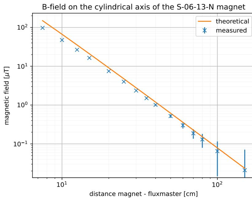
**Figure 7:** Comparison of the theoretical magnetic field along the cylindrical axis of the test magnet and the change in the magnetic field measured with the fluxmaster at various distances from the magnet. The errors are the result of the 0.5 % accuracy and  $< 5 \text{ nT}$  offset stated in the data sheet of the fluxmaster [15] and an uncertainty of  $50 \text{ nT}$  due to fluctuations in the readings during the experiment.
