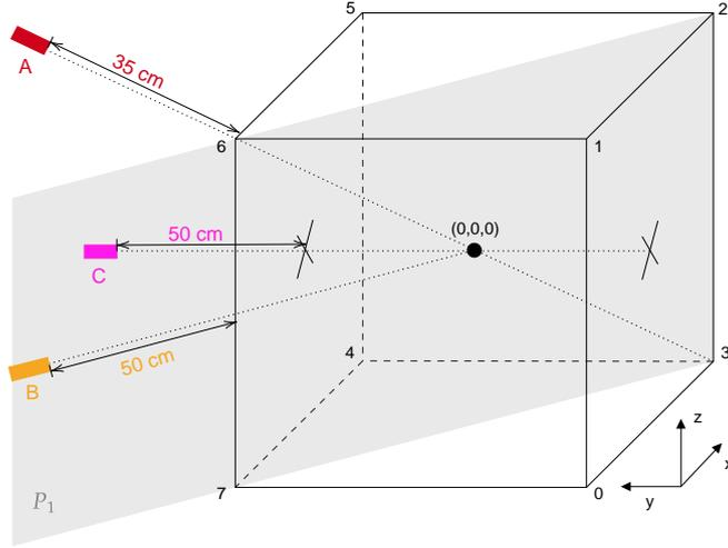
**Figure 11:** Sketch of the different magnet positions (A - C) tested in the experiment in section 6.1. Positions A and B lie on the plane  $P_1$ , whereas C is centered above a face of the Cube. The black numbers indicate the port number of the sensor placed at the corresponding position. The proportions in this sketch are not accurate.
