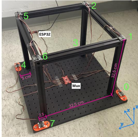
**Figure 3:** 3D setup of 8 MMC sensors (‘Cube’). The green numbers indicate which Mux port the respective sensor is connected to. Sensors 1, 2, 5 and 6 are fixed at the corners of the aluminium structure. The lower sensors 0, 3, 4 and 7 cannot be positioned exactly at the corners and therefore have been placed with an offset in x and y direction such that the positioning of the sensors is symmetric under  $90^\circ$  rotations around the z-axis.
