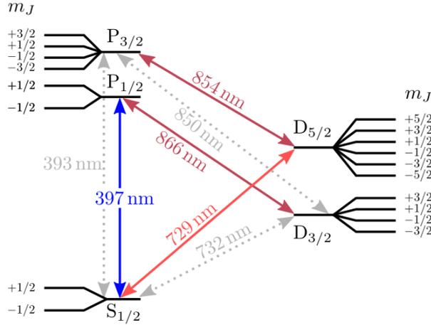
**Figure 1:** Energy level scheme of the  $\text{Ca}^+$  ion. The 729 nm laser drives the transition between  $|0\rangle$  (a Zeeman level of  $D_{5/2}$ ) and  $|1\rangle$  (a Zeeman level of  $S_{1/2}$ ). Note, that not all combinations are possible. Due to the selection rules for electric quadrupole transitions we must satisfy:  $\Delta m_j = 0, \pm 1, \pm 2$ . More information on the other indicated transitions can be found in the source of this illustration: [8]
