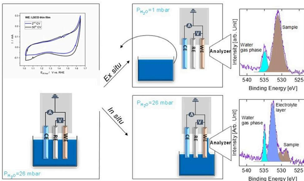
«dip and pull» method, a thin liquid electrolyte layer (10–30 nm thickness) is stabilized at the sample surface. This provides potential control of the working electrode while performing XPS measurements.
