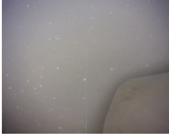
(a) Surface of the ice as seen by the endoscope. The temperature at the moment of the photograph was \simeq -85^\circ\text{C}
