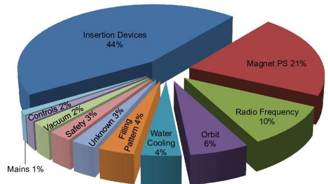
**Figure 7:** Beam outages per failure category at the SLS
