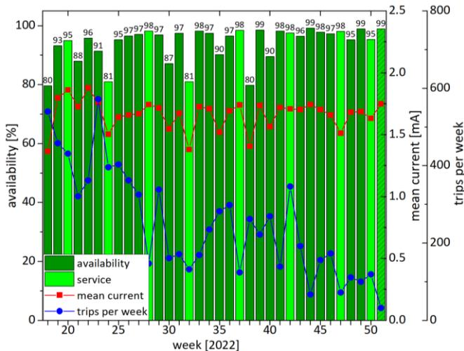
**Figure 1:** Weekly availability of the High Intensity Proton Accelerator Facility in 2022. Due to the energy limitation, the facility was shut down on 19 December, 5 days earlier than scheduled (dashed lines represent last week of operation with only 3 days).
