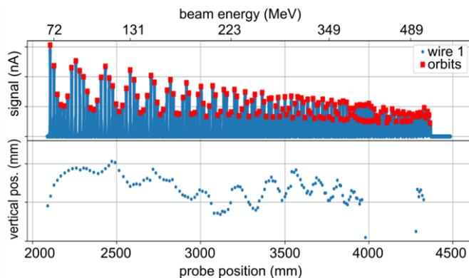
**Figure 3:** Measurement of the radial beam profile (upper plot) in sector two with the new probe RRL. The probe is equipped with 3 wires. One wire is positioned vertically; the other 2 are rotated by 90° against each other. With this setup, the vertical position (lower plot) of the beam can be measured simultaneously.
