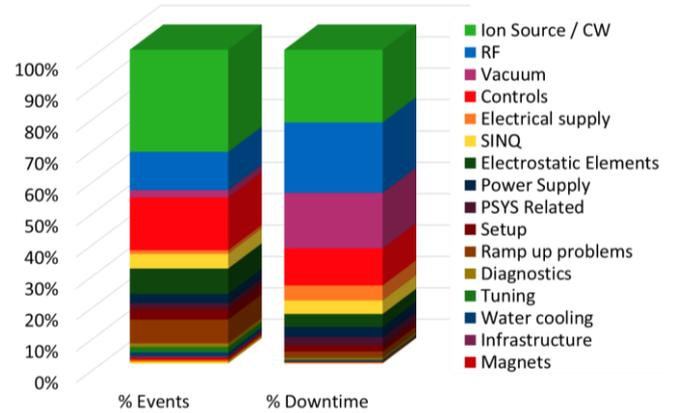
**Figure 2:** Beam outages per failure category at HIPA. The vast majority of failures on the ion source were due to interlocks induced by high voltage instabilities of the electron trap.
