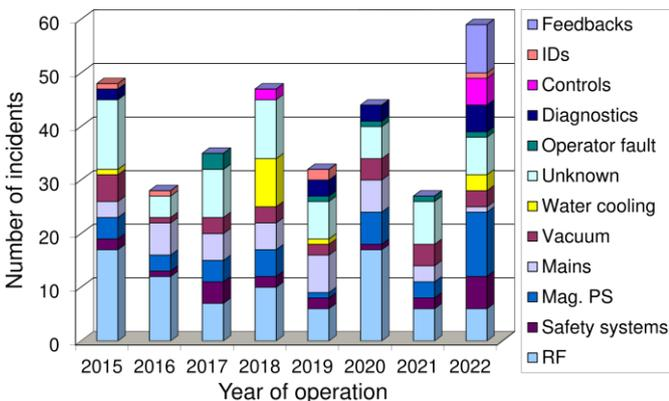
**Figure 5:** Beam outage count per system for the SLS
