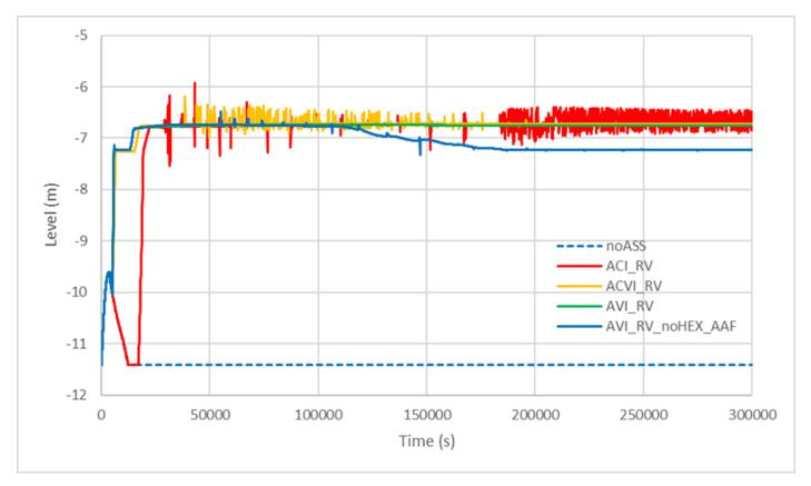
In scenario ACI\_RV reactor cavity dries out for more than one hour before it is flooded again
