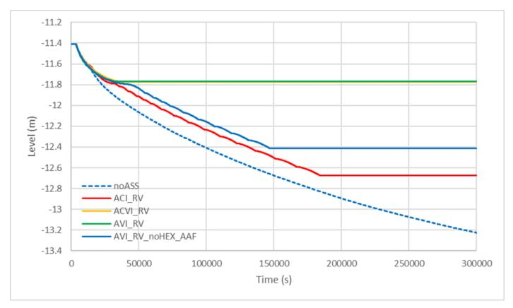
Small differences in flooding conditions influence characteristics of molten core concrete mixture, which influence the MCCI. Consequently, MCCI is very sensitive on flooding conditions.
