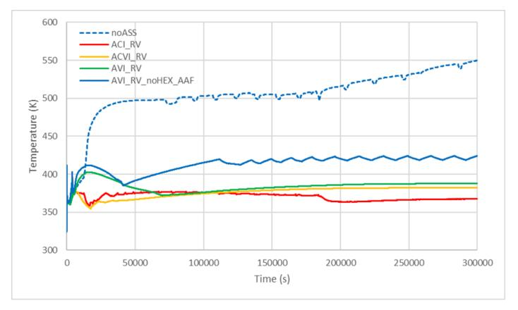
Heat transfer through containment walls not sufficient to extract the entire residual heat from the molten core (noASS)
