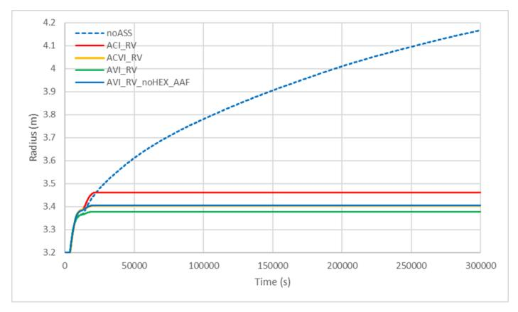
In scenario ACI\_RV, where the molten core dries out for more than one hour before it is flooded again, the extend of the MCCI is significantly larger
