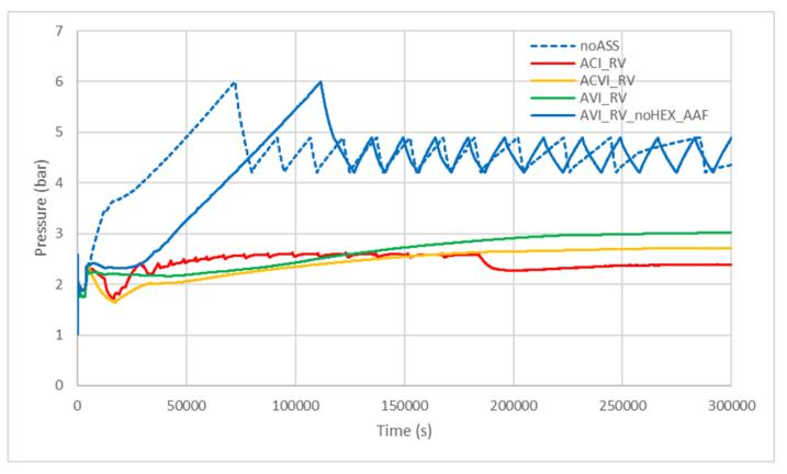
Cooling through steam generators by natural circulation of atmosphere in failed RCS is not sufficient to stabilize severe accident (AVI\_RV\_noHEX\_AAF)
