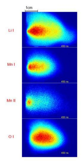
Fig.: Element-selective plasma imaging of the PLD thin film growth of LiMn<sub>2</sub>O<sub>4</sub>
