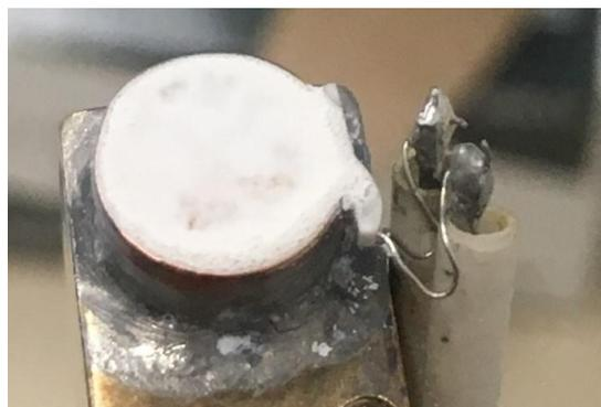
Figure S 4-6. K-feldspar powder sample coated on the sample cryo-holder surface.
