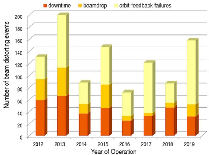
**Figure 5:** Number of beam distortions at the SLS.
