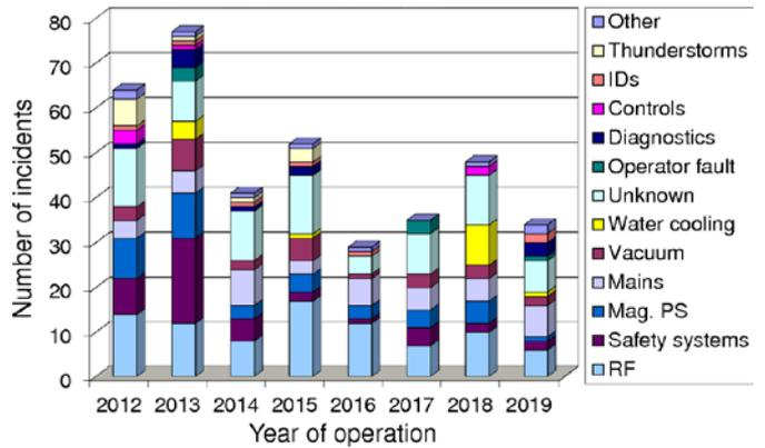
**Figure 4:** Beam outage count per system for the SLS.
