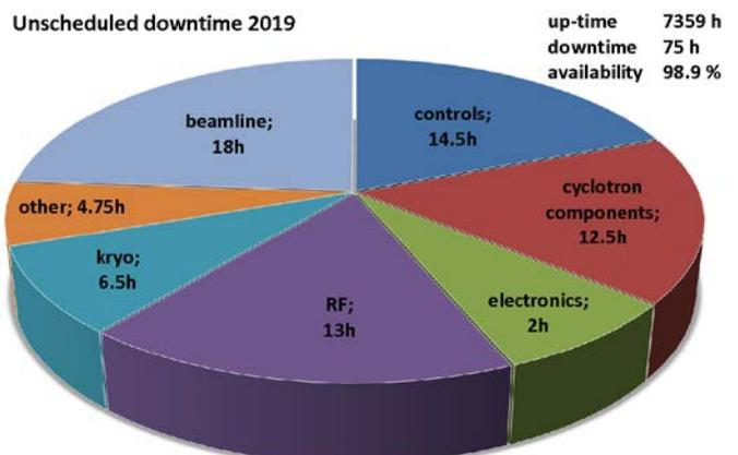
Figure 8: Beam outages per failure category for PROSCAN.
