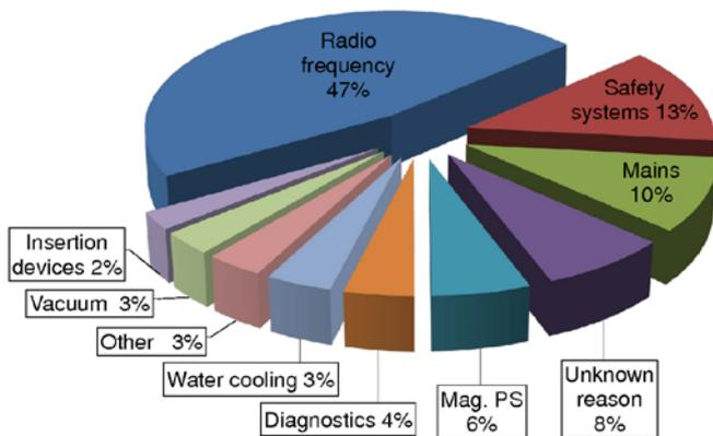
Figure 6: Beam outages per failure category for the SLS.
