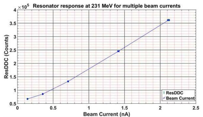
**Figure 11:** Measured response of the non-interceptive beam Intensity monitor.
