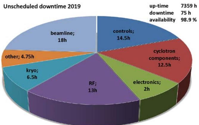
Figure 8: Beam outages per failure category for PROSCAN.
