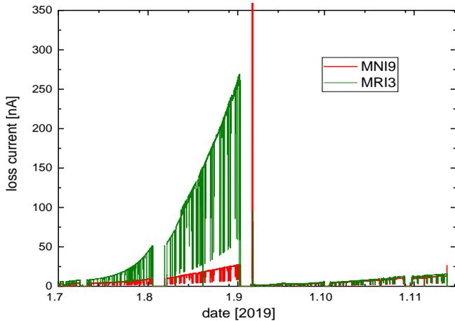
**Figure 3:** Röntgen radiation detected by the loss monitors MN19 (red) and MRI13 (green) in the Ring cyclotron. After the treatment with AQUADAG the radiation level clearly diminished.
