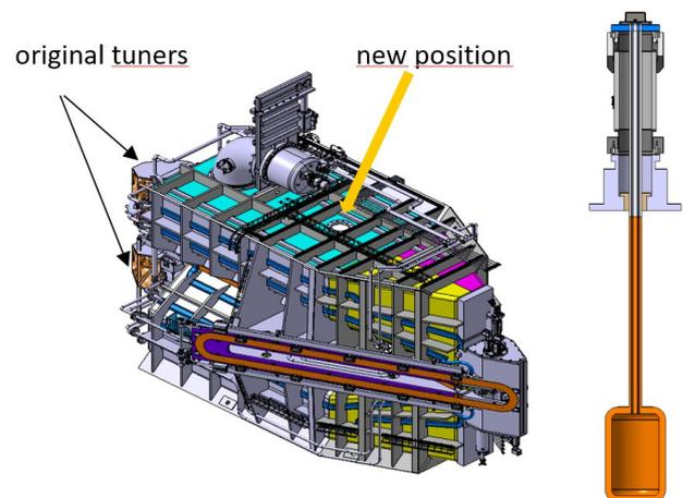
**Figure 3:** right, draft design of a new tuner without finger contacts. The movable displacer will extend 1 m into the resonator to tune the resonance frequency within a range of 200 kHz. It will be installed in a new position in addition to the original tuners.
