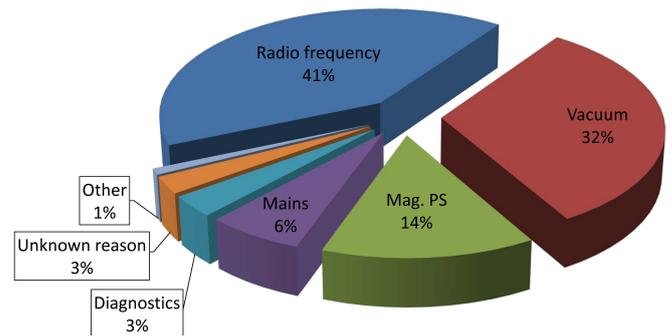
**Figure 5:** Beam outages per failure category at the SLS
