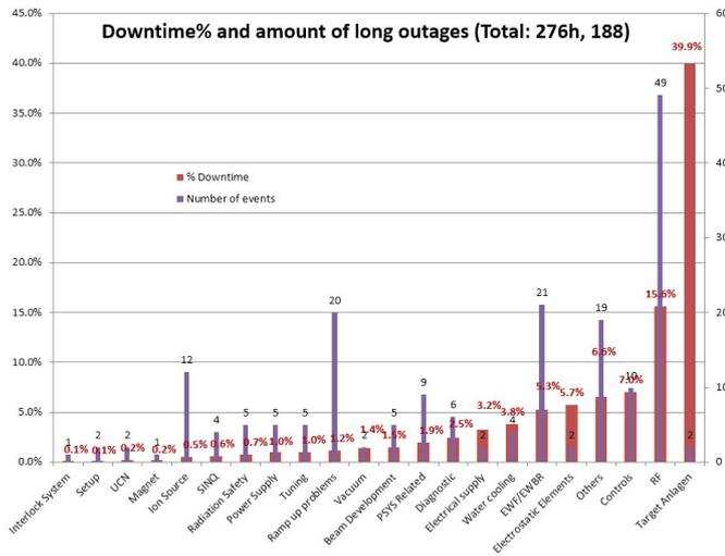
**Figure 2:** long outage (>5m) characteristics of the High Intensity Proton Accelerator facility in 2020
