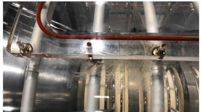
**Figure 1:** Acrylic glass tube surrounding the acceleration section of the Cockcroft-Walton. The visible brownish "bloom", formed a conductive layer of 100 M $\Omega$  instead of the required 50 G $\Omega$ .
