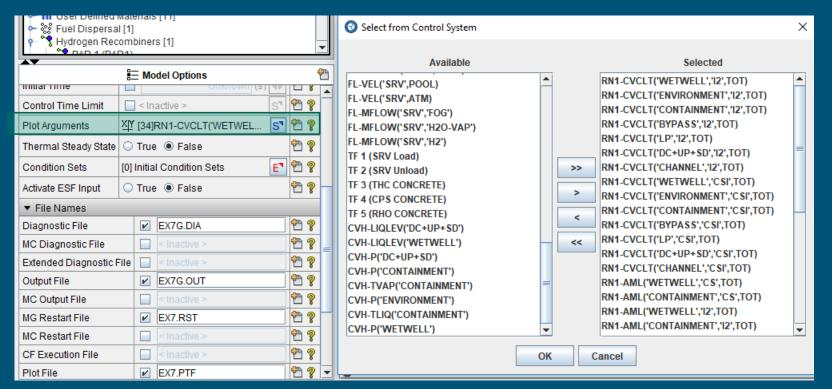
Note that a CF argument must be added to Control System Database before it can be assigned to a plot variable
