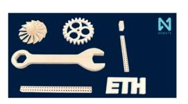
Fully functional LCP objects fabricated with the nematic 3D printing technology.
