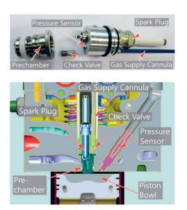
Concept of the novel turbocharged pre-chamber gas engine.
