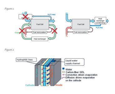
Figure 1: Left: Simplified scheme of a conventionally cooled fuel cell system with humidification of the process air; Right: The novel evaporative cooled system with direct injection of water.
