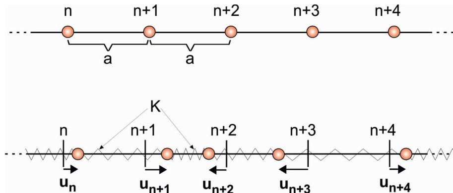
**Figure 1:** Schematic representation of an infinite monatomic 1D linear spring-chain with lattice constant (average interatomic distance)  $a$ . Here  $u_n$  is the displacement of the  $n$ :th atom and  $K$  is the elastic spring constant.
