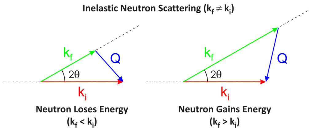
**Figure 3:** Scattering triangles for inelastic neutron scattering (INS) in which the neutron either loses energy ( $\mathbf{k}_f < \mathbf{k}_i$ ) or gains energy ( $\mathbf{k}_f > \mathbf{k}_i$ ) during the interaction with the sample. In both elastic and inelastic scattering events, the neutron is scattered through the angle  $2\theta$ , and the scattering vector is given by the vector relationship  $\mathbf{Q} = \mathbf{k}_i - \mathbf{k}_f$ .
