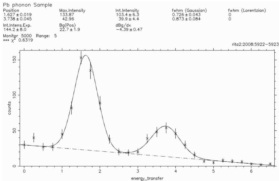
**Figure 6:** Screenshot from the FIT program showing how a constant- $q$  scan is fitted by two Gaussian functions. The positions (energy transfer) showed in the top left corner together with the  $q$ -point at which the scan was performed will yield two unique ( $E, q$ ) points of the phonon dispersion curves [see Fig. 7(a) below]. Remember to also record the error-bars of the position!
