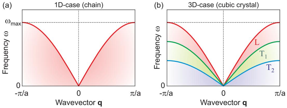
**Figure 2:** (a) Schematic dispersion curve for a monatomic linear chain with only nearest-neighbor interactions. Note that the frequency is linear for small  $q$  and that  $\partial\omega/\partial q$  vanishes at the zone-boundaries (i.e.  $q = \pm\pi/a$ ). (b)
