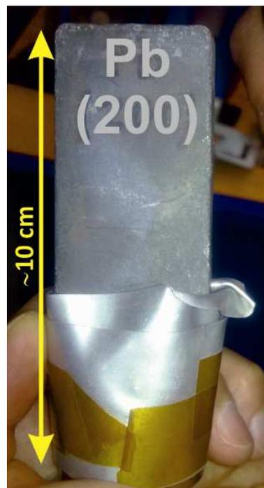
When the Pb crystal is aligned, you will acquire a series of either constant-q or constant-energy scans (or a combination) in order to map out the phonon-dispersion ( $h\nu$  as a function of  $q$ ) along a selected high-symmetry direction ( $h\ 0\ 0$ ). How to perform a scan will be shown to you by the local contact. However, just as an example, the two scans shown above in **Fig. X** are at the TASP instrument performed by running the following two text commands in the SIX-prompt:
