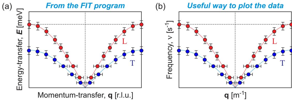
**Figure 7:** (a) Schematic view of how the extracted points obtained from fits of the data are plotted as phonon dispersion. (b) Useful way to plot the data from the viewpoint of extracting further properties in a straightforward manner (units!).
