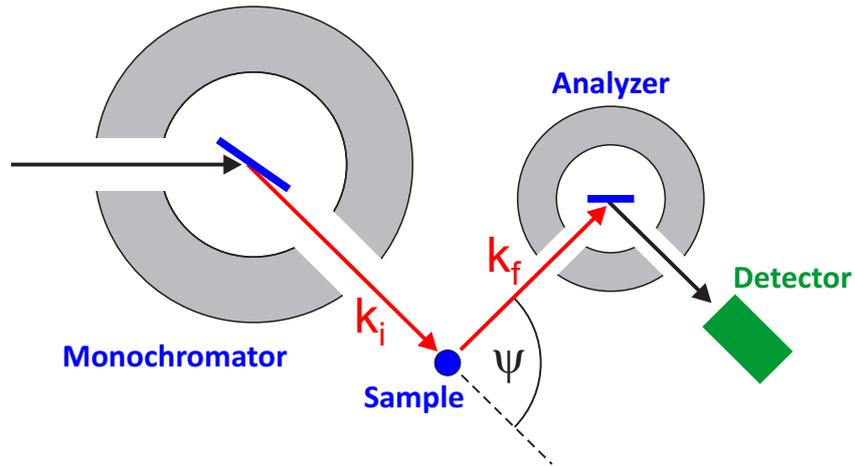
**Figure 4:** Schematic layout of a neutron triple-axis spectrometer.
