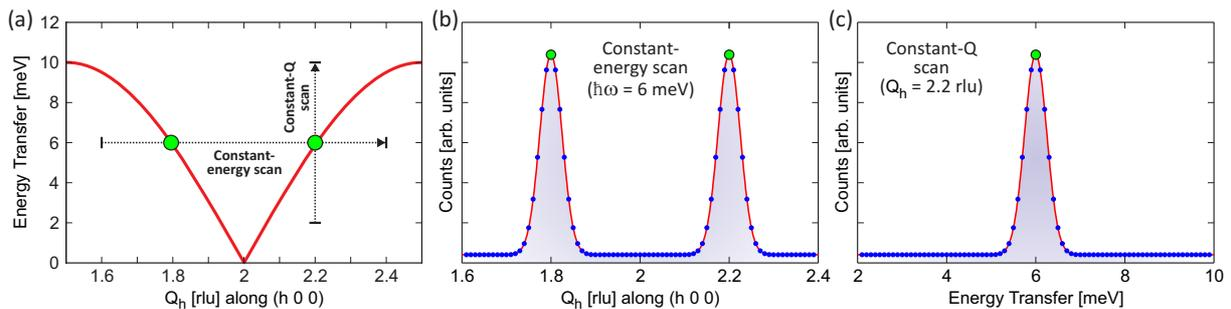
**Figure 5:** (a) Schematic view of how two points of the phonon dispersion curve can be measured using either (b) constant-energy scan or (c) constant- $Q$  scan. By performing multiple scans it is possible to map out the complete dispersion (see below).
