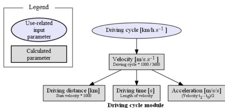
Figure 1 Parameters calculated from the driving cycle
