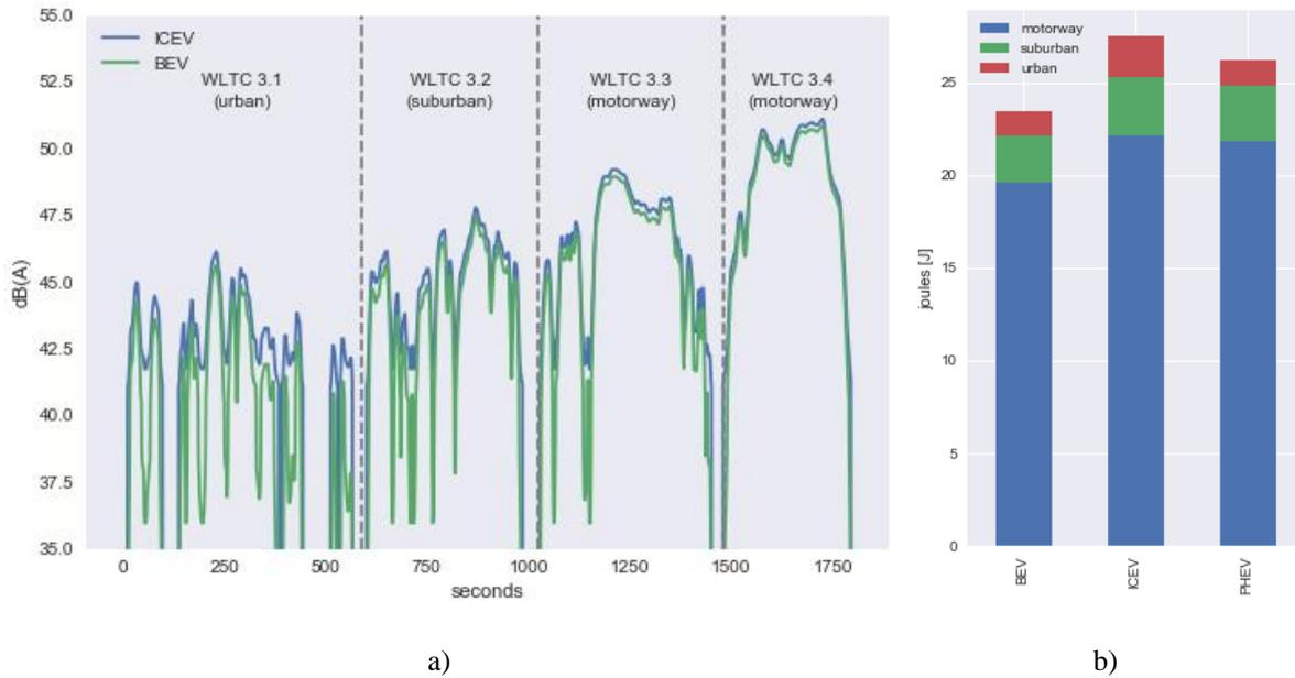
Figure 5 a) Noise emission level comparison between ICEV and BEV, based on the driving cycle WLTC. b) – Summed sound energy comparison between ICEV, BEV and PHEV, over the duration of the WLTC driving cycle.
