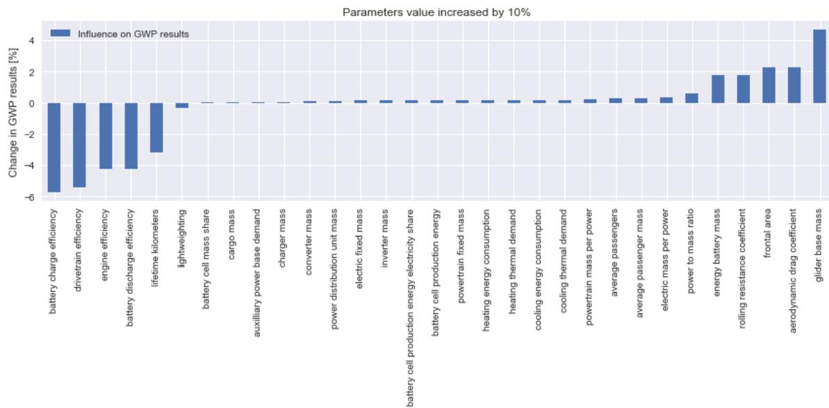
Figure 12 Sensitivity of GWP results in regard to parameters for BEV
