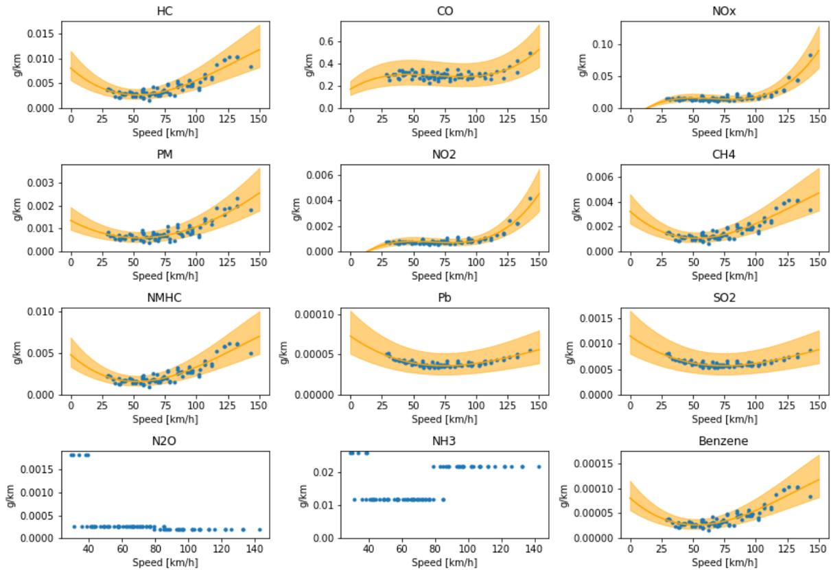
Figure 3 Relation between speed level and exhaust emissions for a gasoline-fueled vehicle. Blue dots: emission values modelled by HBEFA 4.1. Orange line: linear regression used by *calculator* as best-guess value. Yellow shaded area: minimum-maximum value range used for error propagation analyses. Data source: HBEFA 4.1
