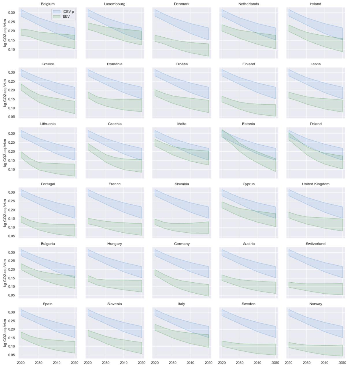
Figure 9 Life cycle GHG emissions of ICEV-p and BEV in EU-27, Norway, Switzerland and the United Kingdom, including error propagation analysis. Lower interval boundary: 25<sup>th</sup> percentile of Monte Carlo distribution using the “SSP2-PkBudg1100” REMIND energy scenario in the background inventory database. Upper interval boundary: 75<sup>th</sup> percentile of Monte Carlo distribution using the “SSP2-Baseline” REMIND energy scenario in the background inventory database.
