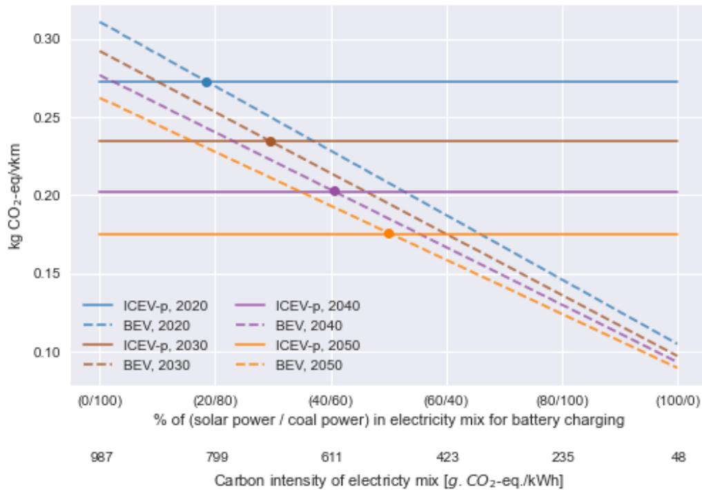
Figure 10 Effect of increasing the share of solar power at the expense of coal-based power in the electricity mix used for battery charging on the GHG emissions of a medium-size BEV
