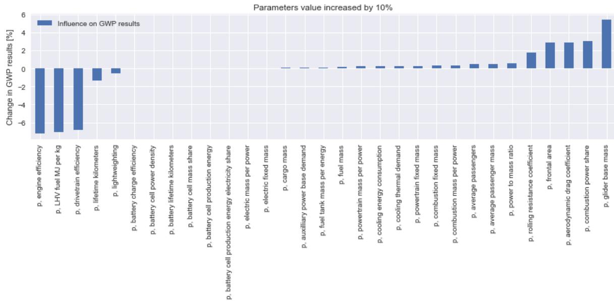
Figure 11 Sensitivity of GWP results in regard to parameters for ICEV-p
