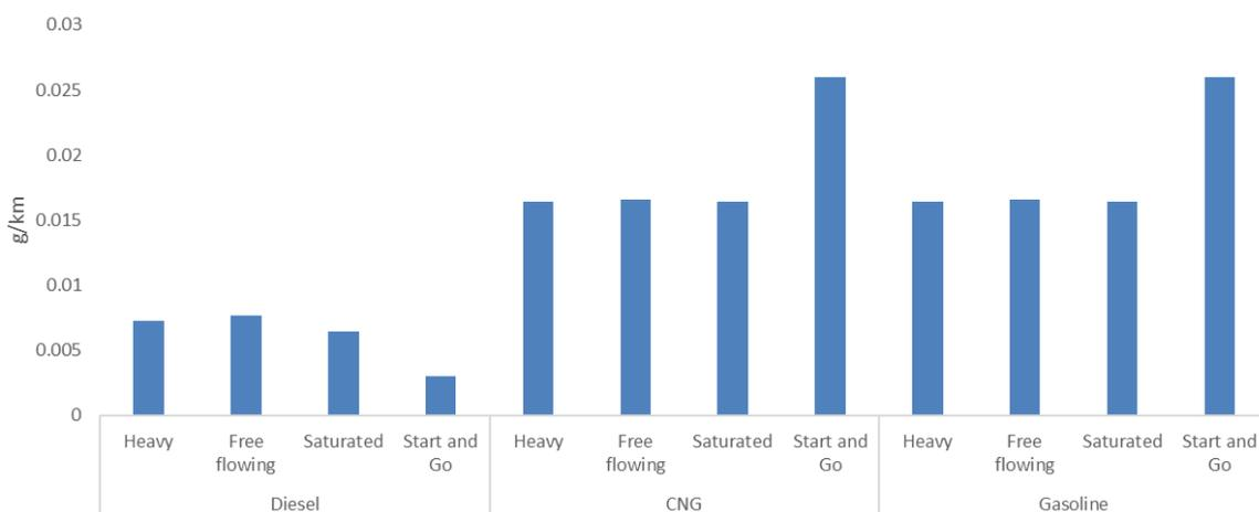
Figure 4 Relation between ammonia ( $\text{NH}_3$ ) emissions and traffic situations for EURO 6d diesel, gas and gasoline-fueled vehicles. Data source: HBEFA 4.1 [49]
