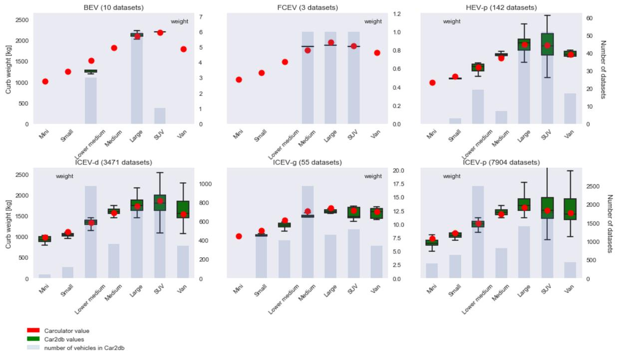
Figure 7 Validation of the curb mass against the datasets from the passenger vehicles database Car2db. Horizontal lines within the green boxes represent the median value. The green boxes represent 50% of the distribution (25<sup>th</sup>-75<sup>th</sup> percentiles). The whiskers represent 90% of the distribution (5<sup>th</sup>-95<sup>th</sup> percentiles). Outliers are not shown. Source for vehicle datasets: [56]
