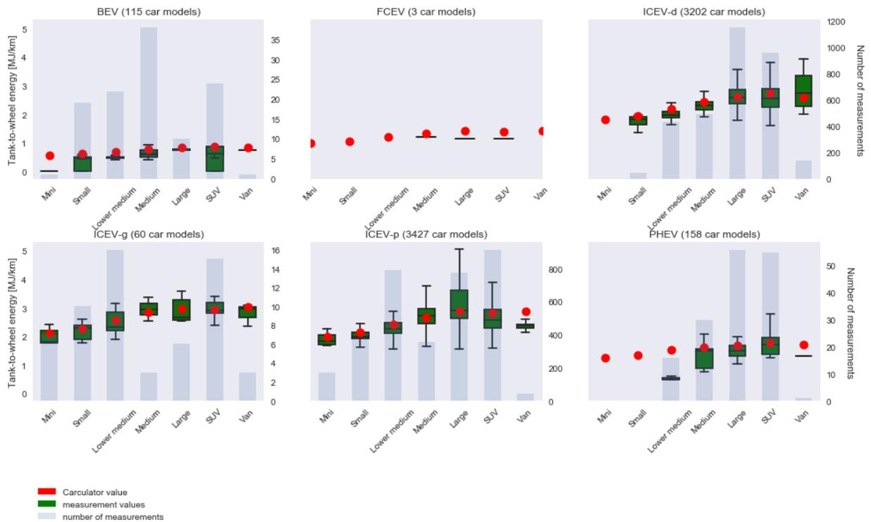
Figure 8 Validation of Tank-to-wheel energy requirement against the monitoring program for passenger vehicle emissions database. Horizontal lines within the green boxes represent the median value. The green boxes represent 50% of the distribution (25<sup>th</sup>-75<sup>th</sup> percentiles). The whiskers represent 90% of the distribution (5<sup>th</sup>-95<sup>th</sup> percentiles). Outliers are not shown. Source for vehicle tank-to-wheel energy consumption measurements: [57]
