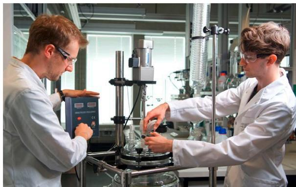
Setting up a new grafting reactor for the scaled-up production of Amphion™ membranes for vanadium redox flow batteries.
