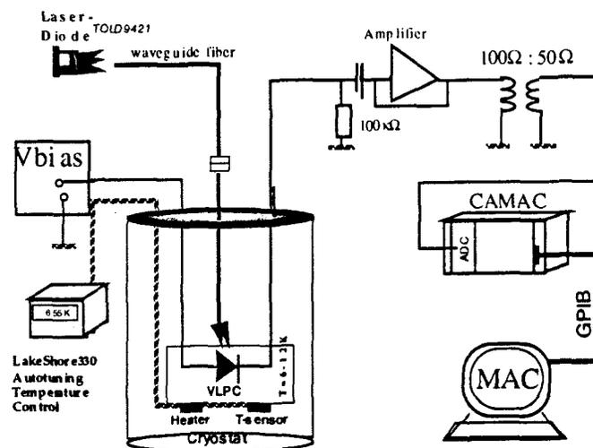
Figure 7: Signal flow diagram for the VLPC test-station.
