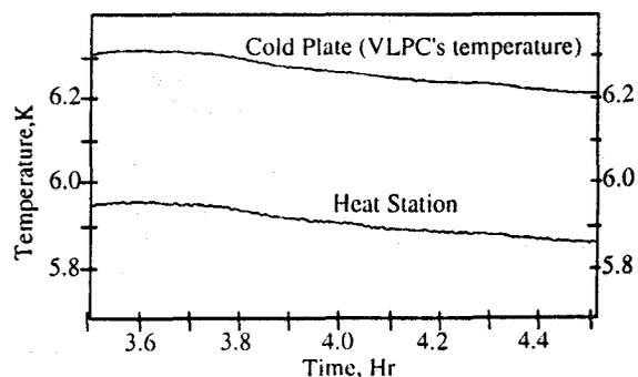
Figure 2: Temperatures of Cold Plate and First Heat Station during 1 hour period.
