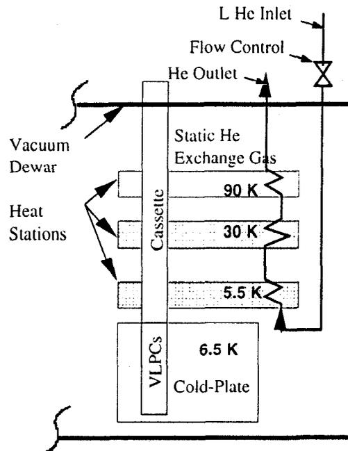
Figure 1: The compact VLPC transducer cryostat concept.
