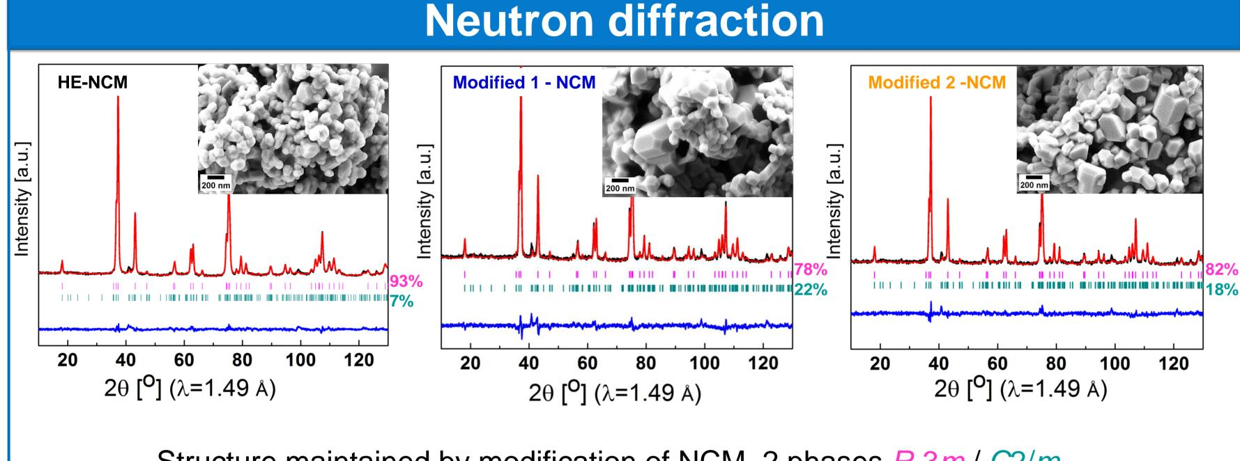
Structure maintained by modification of NCM, 2 phases R-3m / C2/m Increase of lattice volume when NCM is modified
