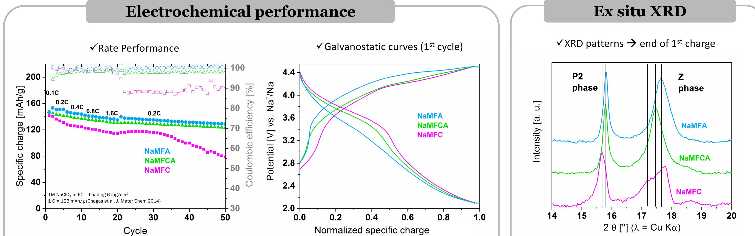
Higher performance with Al containing materials Loss of~300 mV in discharge potential for NaMFA
