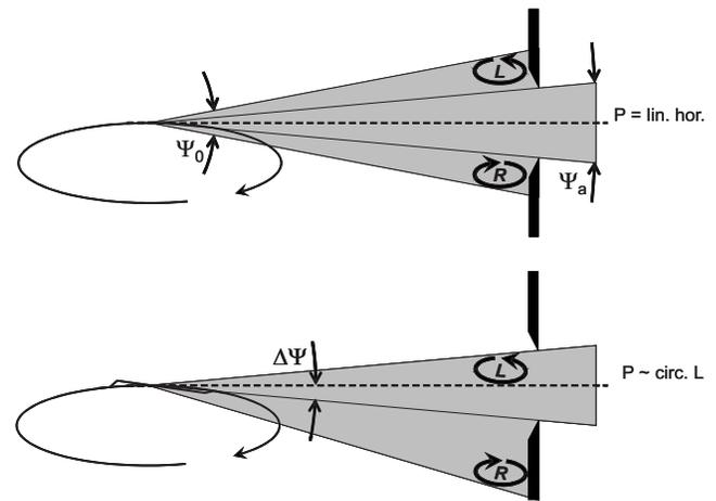
FIG. 6. Scheme showing how circularly polarized light is obtained from a bending magnet by tilting the storage ring orbit relative to the optical axis of the beamline. The beamline acceptance is  $\psi_A$ ; the tilt angle of the orbit is  $\Delta\psi$  ( $\leq \pm 300 \mu\text{rad}$ ).
