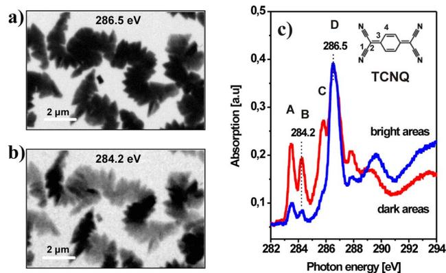
FIG. 10. (Color online) STXM transmission images at (a) 286.5 eV and (b) 284.2 eV of 200 nm thick TCNQ film grown on top of a 5 nm silver film; (c)  $C K$ -edge NEXAFS spectra extracted from line scans taken across bright and dark microcrystallites shown in (b). The line scans were performed with 0.02 eV energy step from 280 to 295 eV with 40 ms dwell time per pixel.
