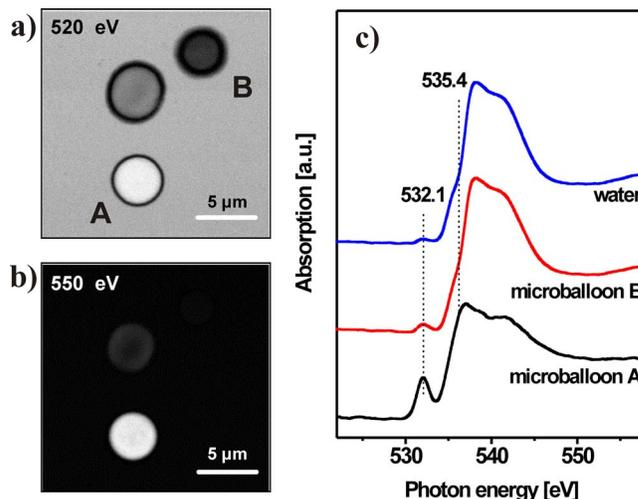
FIG. 13. (Color online) STXM transmission images of microballoons in water environment recorded at (a) 520 eV and (b) 550 eV. (c) Oxygen *K*-edge NEXAFS spectra of the surrounding water and the interior parts of microballoons A and B.
