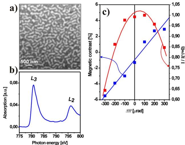
FIG. 9. (Color online) Magnetic imaging of a CoPt/IrMn multilayer sample (total Co thickness=6 nm). The well known worm domains of about 200 nm width are shown in (a), a spectrum taken at the Co  $L$  edge in (b), and the magnetic contrast and relative intensity as a function of bump angle  $\Delta\psi$  in (c).
