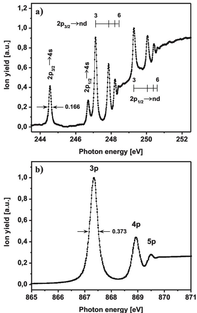
FIG. 4. (a) Argon  $L_{2,3}$  photoion yield measurement for 300 lines/mm grating and 10  $\mu\text{m}$  exit slit setting. (b) Measured  $1s$ - $np$  transition series of neon with 600 lines/mm grating.
