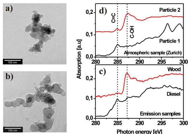
FIG. 12. (Color online) TEM bright field micrograph of (a) soot particle from wood combustion and (b) diesel soot. Both consist of chains of primary particles. C  $K$ -edge NEXAFS spectra of (c) single soot particles from wood and diesel combustion and (d) from two particles in an atmospheric sample, collected along an arterial road in Zurich.
