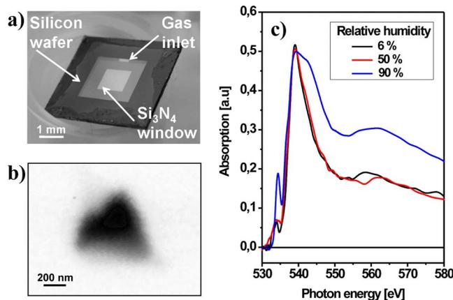
FIG. 11. (Color online) Climate cell (a) consisting of two silicon wafers with  $\text{Si}_3\text{N}_4$  windows ( $t=100$  nm) and a gas inlet and outlet (not visible). STXM transmission image taken at 540 eV of an individual particle composed of ammonium sulfate and adipic acid is shown in (b). The dependence of the oxygen  $K$ -edge spectrum of an ammonium sulfate/adipic acid film on the humidity is shown in (c). See text for details.
