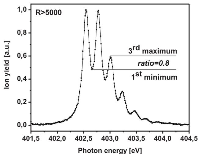
FIG. 2. Measured photoion yield at the nitrogen  $1s \rightarrow \pi^*$  transition using the gas cell located between exit slit and FZP of the PolLux beamline (300 lines/mm grating, 10  $\mu\text{m}$  slits). The intensity ratio of the first minimum to the third maximum (0.8) indicates an energy resolution in excess of  $E/\Delta E \sim 5000$  (Ref. 23).
