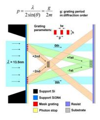
Figure 1. Schematic of EUV-IL. The mask gratings diffract the incident light into beams which interfere, with periodicity, p, given by the equation
