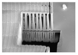
**Figure 2:** FIB cross section of a double-sided blazed zone plate. The coarse structures are on the front and the dense are on the back side.
