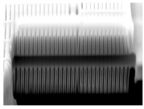
**Figure 1:** FIB cross section of a double-sided line-doubled zone plate with 30 nm zone width and 1.1 µm combined structure height.
