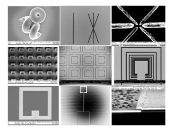
Fig. 1 Collage of different THz antennas featuring with nanometer sized gaps.
