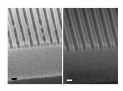
Figure 2. Cross-sectional SEM images of silicon nanowires etched into silicon-on-insulator substrate using RIE-ICP. Scale bar is 20 nm. Left: 14 nm half-pitch. Right: 16 nm half-pitch.
