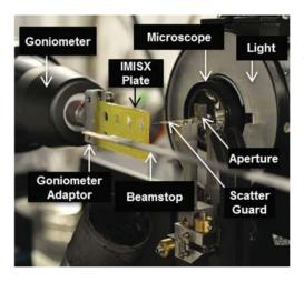
Figure 1: A view of a section of an IMISX plate in the goniometer positioned for SX data collection on beamline PXII (X10SA) at SLS.
