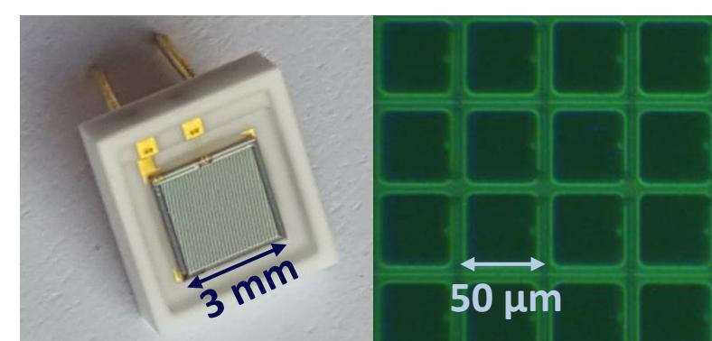
Array of Avalanche Photodiodes in Geiger mode allows for photon counting measurements.
