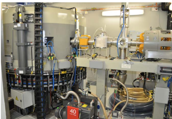
Fig. 1: The Bern cyclotron with its characteristic beam transport line.
