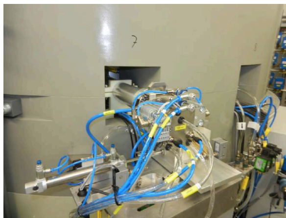
Fig. 3: The solid target station for the production of radionuclides.
