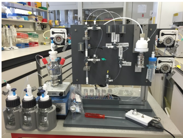
Fig. 1: ^{64}\text{Cu} chemical separation apparatus for hot cell production.
