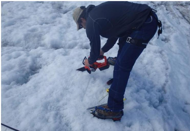
**Figure 12** Cutting of the ice blocks samples using an electrical chainsaw.
