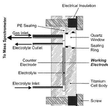
**Fig. 1:** Schematic view of the new DEMS cell.
