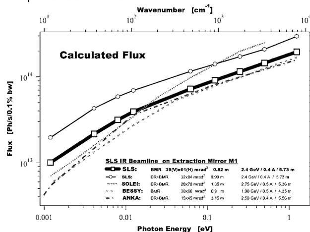
**Fig. 2:** Extracted IR radiation flux from the SLS ring by sole BM Radiation (squares) and ER+BM Radiation (circles) for several photon energies. The values were calculated on the position of the extraction mirror M1. For comparison the extracted flux from other beamlines are displayed (dashed lines).
