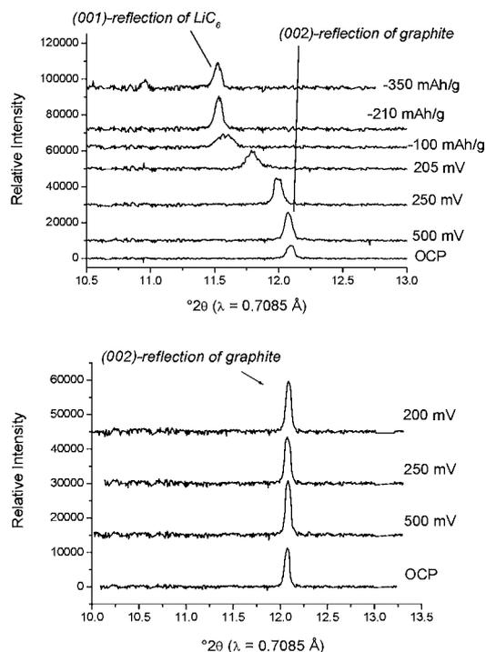
**Fig. 1:** *In situ* synchrotron x-ray diffraction patterns of Graphite A (top) and SLX50-HT (bottom). Electrolyte: EC:DMC (1:1), 1M  $\text{LiPF}_6$ .
