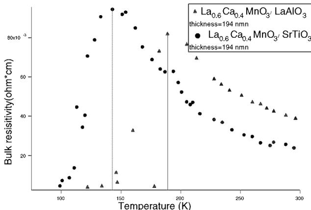
**Fig. 1:** Temperature dependences of the resistivity for LCMO thin films deposited on  $\text{SrTiO}_3$  (left) and  $\text{LaAlO}_3$  (right).
