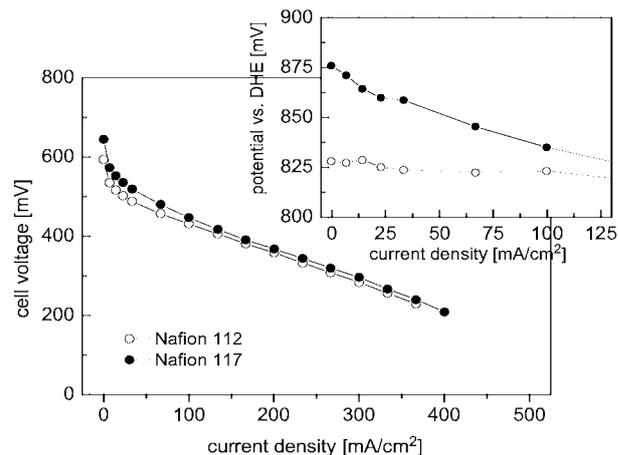
Fig. 2: Polarisation curves for DMFC with Nafion 112 and 117 at 60°C 1bar(a); oxidant is air; inset shows cathodic polarisation at low current densities.
