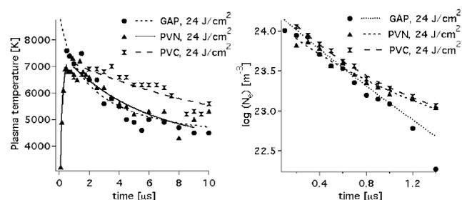
**Fig. 4:** The decay of the plasma temperature (a) and the electron density (b).
