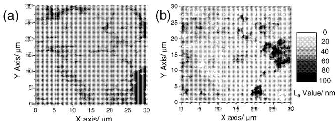
**Fig. 1:** *Ex situ* Raman mapping of graphite surface showing the comparison of (a) the optical picture of the surface of graphite and (b) the high number point  $L_a$  map; 50 x 50 points; 2500 spectra.
