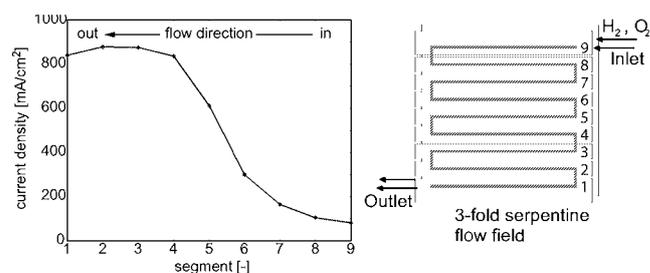
**Fig. 3:** Current density distribution in co-flow mode of the reactant gases (r.h. 50%).
