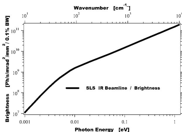
**Fig. 6:** The expected brightness calculated for the SLS IR beamline [1].
