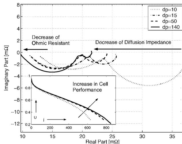
**Fig. 1:** Selected impedance measurements at various pressure differences between cathode and anode. The inset shows the polarisation curves at corresponding pressure differences.
