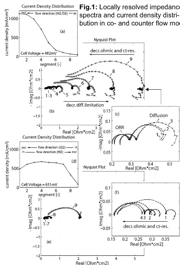
**Fig.1:** Locally resolved impedance spectra and current density distribution in co- and counter flow mode.
