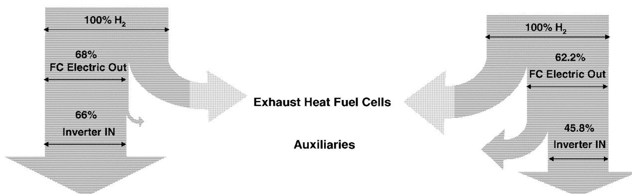
**Fig. 3:** Tank to electric power efficiencies of automotive fuel cell power trains. Left: HY-LIGHT  $H_2/O_2$  32 kW peak power system for average power of 7 kW, data obtained on the road in arbitrary driving cycle. Right  $H_2$ /air, 55 kW peak power system, for average power of 12 kW, data obtained for NEFZ [1].
