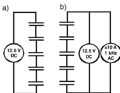
**Fig. 1:** Sketch of the test circuit for the two capacitor strings. a) reference, b) with ripple current.
