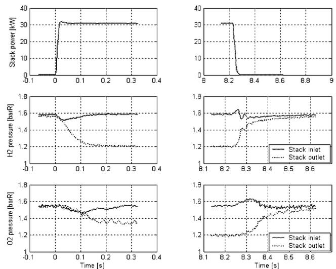
**Fig. 2:** Pressure response of gases to positive power step (left) and negative power step (right).
