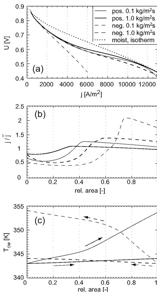
**Fig. 2:** Polarisation curves for co flowing reactants and different cooling flow arrangements (a), the normalized local current densities (b), and coolant temperatures (c) at 6000 A/m<sup>2</sup>. The reactants flow from left to right.
