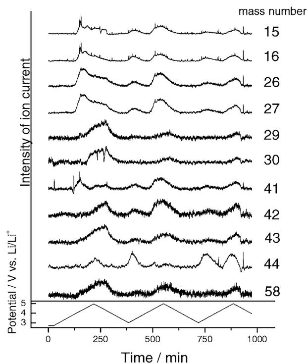
**Fig. 5:** Intensity of the ion currents at the investigated mass numbers in dependence on the applied potential. For a better illustration strong signals (e.g. 44) were scaled.
