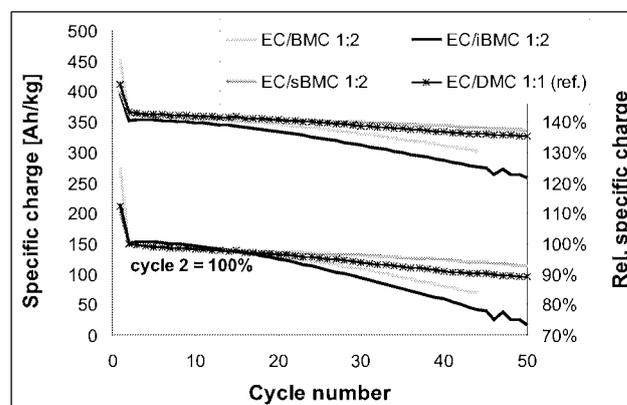
Fig. 2: Relative (bottom) and absolute (top) cycling behaviour (Li intercalation) in SLP30 half cells vs. met. Li with isomeric BMC electrolytes containing 1M LiPF<sub>6</sub>.
