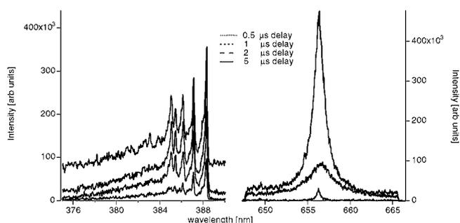
**Fig. 3:** Time dependent decay of the emission peaks of CN Violet (left) and H-Balmer- $\alpha$  (right).
