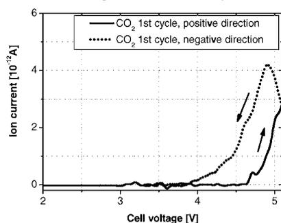
**Fig. 3:** DEMS measurement on  $\text{LiCoO}_2$ , electrolyte EC/DMC 1:1 + 2% VC, 1M  $\text{LiPF}_6$ .
