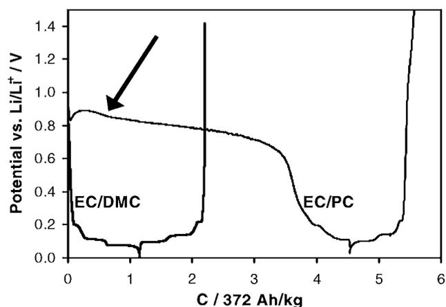
**Fig. 1:** First electrochemical intercalation/deintercalation of lithium into/from TIMREX<sup>®</sup> SLX50 in 1 M LiPF<sub>6</sub>, EC/DMC 1/1 (w/w) and in 1 M LiPF<sub>6</sub>, EC/PC 1/1 (w/w) as electrolyte at a specific current of 10 mA/g.
