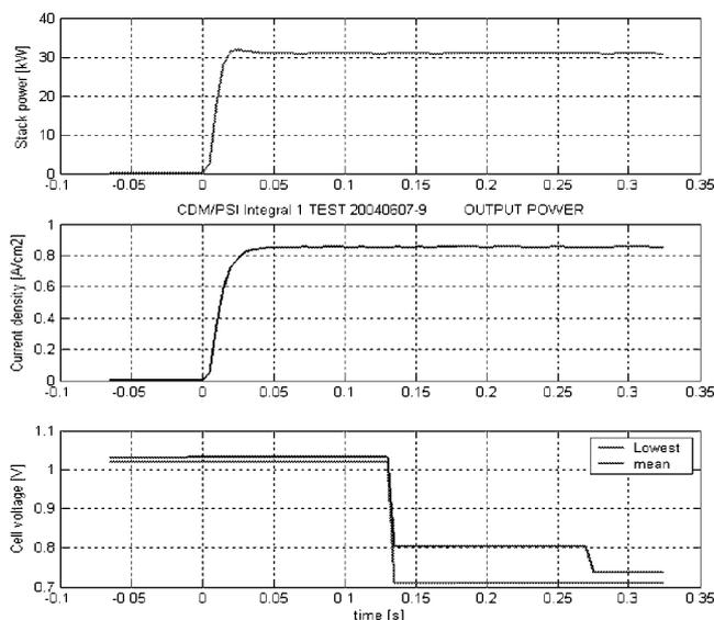
**Fig. 1:** Power, current density and cell voltages for 0 to 30 kW power step.
