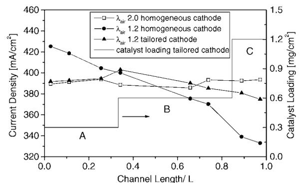
**Fig. 1:** Current density distribution as a function of the channel length.  $\lambda_{\text{air}} = 2.0$  and 1.2 for the homogeneous cathode and 1.2 for the tailored cathode.  $\lambda_{\text{H}_2} = 2.0$ ,  $T_{\text{cell}} = 70^\circ\text{C}$ , air and  $\text{H}_2$  dew point =  $70^\circ\text{C}$ , air and  $\text{H}_2$  pressure = 2.0 bara. Constant Current mode with avg. current density 400  $\text{mA}/\text{cm}^2$ . A, B and C see text.
