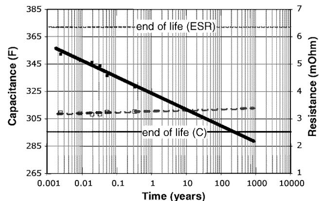
**Fig. 2:** Capacitance fading (full line) and ESR increase (dashed line) of an EDLC at 25 °C and 2.5 V.
