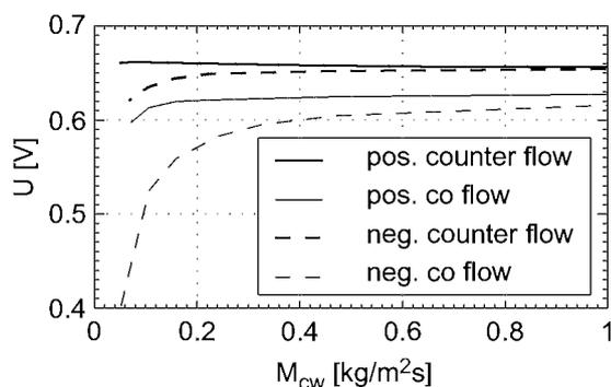
**Fig. 1:** The effect of coolant mass flow on the cell voltage at 5000 A/m<sup>2</sup> for different flow arrangements.
