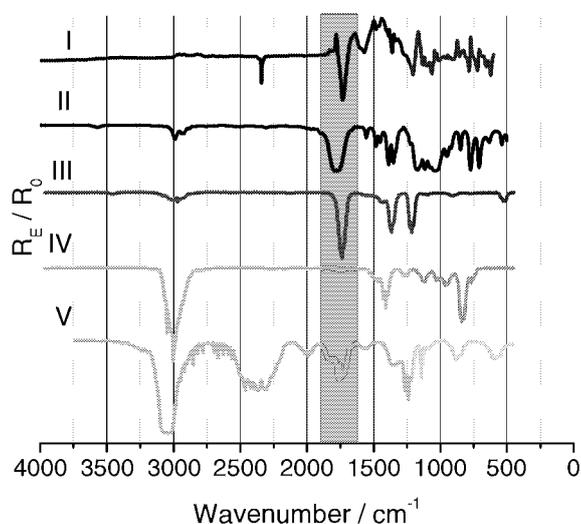
**Fig. 2:** SNIFTIR spectra measured on a polished nickel electrode in the electrolyte (I) 1 M LiClO<sub>4</sub> in PC at 5 V vs. Li/Li<sup>+</sup>, IR-spectra of PC (II), acetone (III), propylene oxide (IV) and propanal (V).
