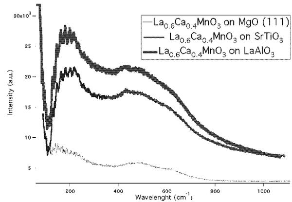
**Fig. 2:** Raman spectra of  $\text{La}_{0.6}\text{Co}_{0.4}\text{MnO}_3$  thin films on  $\text{LaAlO}_3$ ,  $\text{SrTiO}_3$  and MgO substrates. Active vibrations at  $425\text{ cm}^{-1}$  were recorded for the  $\text{LaAlO}_3$  substrate and  $437\text{ cm}^{-1}$  for the  $\text{SrTiO}_3$  substrate.
