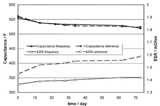
**Fig. 2:** Decay of capacitance and ESR for both capacitor strings with time. Full lines: Test string with ripple current (labelled 'frequency'), dashed lines: reference string. Full symbols: capacitance, open symbols: ESR @ 1 kHz.
