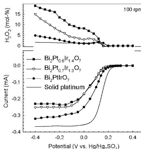
**Fig. 2:**  $\text{O}_2$  reduction and  $\text{H}_2\text{O}_2$  formation on  $\text{Bi}_2\text{Pt}_{2-y}\text{Ir}_y\text{O}_7$  ( $y = 1, 1.3, 1.4$ ) RDEs compared to a solid polycrystalline Pt RDE in  $\text{O}_2$ -saturated 0.5 M  $\text{H}_2\text{SO}_4$ . Scan rate = 5 mV/s.
