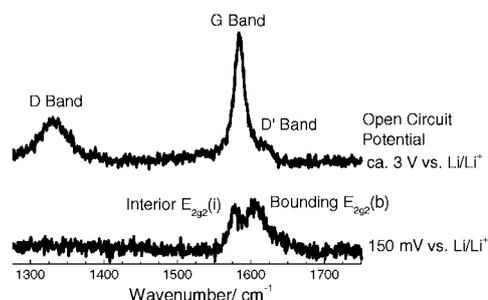
**Fig. 2:** The Raman spectra of graphite at OCP (ca. 3.0 V vs.  $\text{Li/Li}^+$ ) and at 150 mV vs.  $\text{Li/Li}^+$ .
