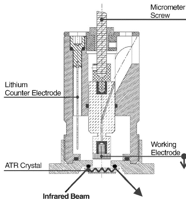
**Fig. 1:** Schematic of the ATR-SNIFTIRS cell used. The internal reflection element (ZnSe) allows up to six reflections.
