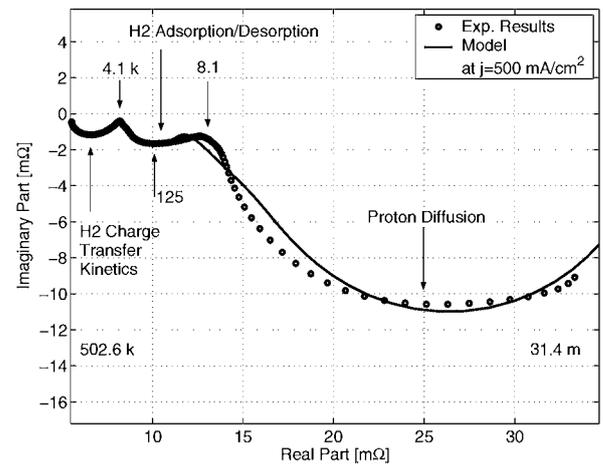
**Fig. 1:** Comparison between experimental and simulated results at current density of  $j = 500 \text{ mA/cm}^2$  for the HOR. Units of selected frequencies are  $\text{rads}^{-1}$ .
