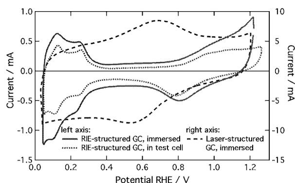
**Fig. 2:** CVs of micro structured and Pt-coated GC electrodes recorded at a scan rate of  $100 \text{ mV/s}$ .
