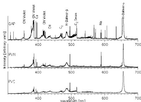
**Fig. 2:** Emission spectra of GAP, PVN and PVC, doped with carbon, 1  $\mu\text{s}$  after irradiation at 1064 nm.
