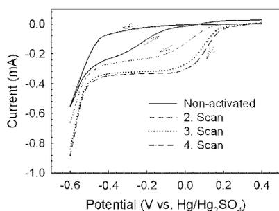
**Fig. 1:** The development of ORR activity of a fresh  $\text{Bi}_2\text{PtIrO}_7$  powder pellet in  $\text{O}_2$ -saturated 0.5 M  $\text{H}_2\text{SO}_4$  at 100 rpm. Scan rate = 5 mV/s. Cathodic scans are only shown for scans 2-4.
