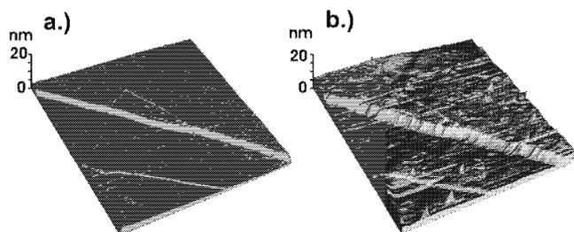
**Fig. 1:** *In situ* contact-AFM images ( $1.5 \mu m \times 1.5 \mu m$ ) of HOPG in PC with 1M  $(C_2H_5)_4NBF_4$  at the same location. a) At 3 V vs.  $Li/Li^+$ . b) At 1 V vs.  $Li/Li^+$ .
