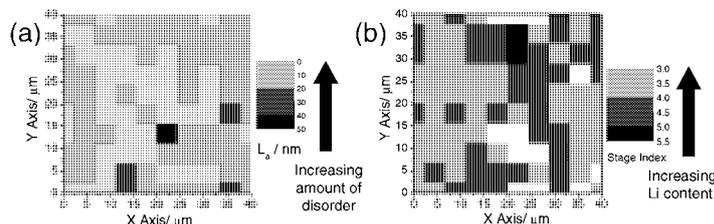
**Fig. 3:** (a)  $L_a$  map of graphite (OCP ca. 3.0 V vs.  $\text{Li/Li}^+$ ) and (b) lithium content map (150 mV vs.  $\text{Li/Li}^+$ ) 10 x 10 points; 100 spectra (bad points in white).
