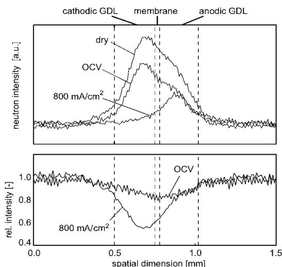
**Fig. 1:** Neutron intensities over the thickness of the MEA for different operating conditions.
