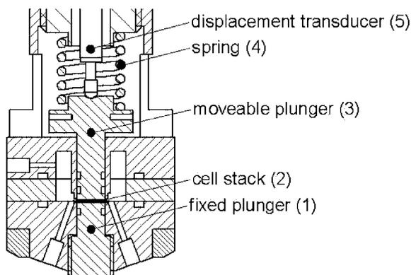
**Fig. 1:** Cross sectional view of the dilatometer. The cell stack (not shown in detail) is held between two plungers (1 and 3).
