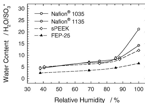
Fig. 1: Membrane hydration, expressed as molecules of water per sulfonic acid group, at room temperature.
