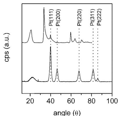
**Fig. 3:** XRD patterns of  $\text{PtO}_2$  before (top) and after controlled-potential electroreduction (bottom).
