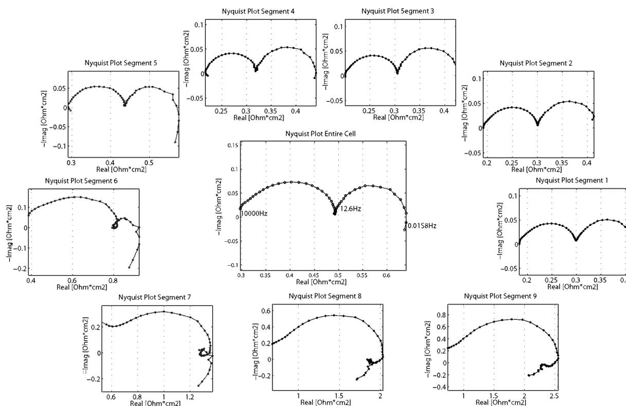
**Fig. 4:** Impedance spectra of segments 1-9 and calculated impedance spectrum of the entire cell.
