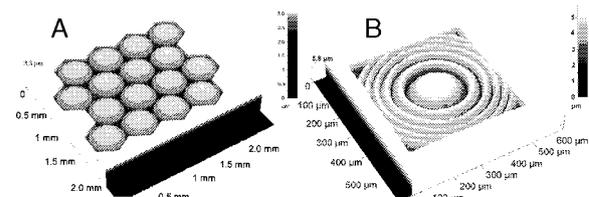
Fig. 2: Image of a plano-convex micro-lens array in quartz (A) and a Fresnel lens in BaF<sub>2</sub> (B)
