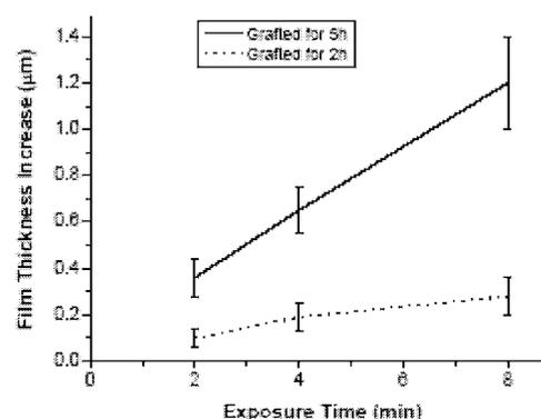
**Fig. 2:** Dependence of film thickness increase on exposure dose and grafting time measured by profilometer for styrene/DVB grafted FEP films.
