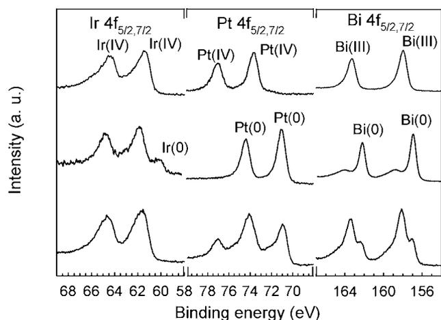
**Fig. 2:** High resolution XP-spectra of the Ir, Pt and Bi 4f electrons in  $\text{Bi}_2\text{PtIrO}_7$  as prepared (top), after electrolysis at -0.8 V (middle) and after CV between -0.6 and 0.6 V (bottom).
