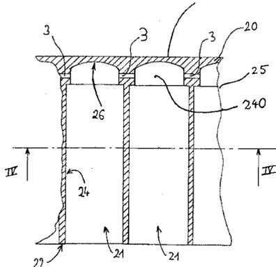
**Fig. 2:** Principle of the hydrogen storage which is an integral structure of the chassis.
