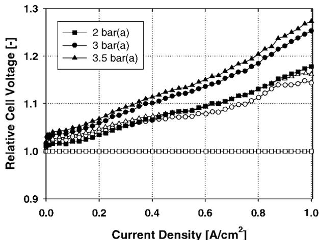
**Fig. 1:** Relative performance of cell of technical size for operation with H<sub>2</sub>/O<sub>2</sub> (■●▲) and H<sub>2</sub>/air (○△) relative to H<sub>2</sub>/air at 2 bar<sub>a</sub> (□) as the base case.
