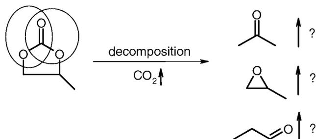
**Fig. 3:** Possible products of propylene carbonate decomposition.
