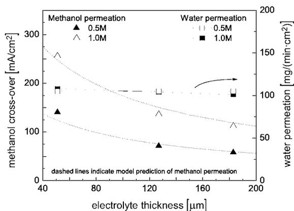
Fig. 1: Methanol and water permeation as a function of membrane thickness for Nafion membranes.
