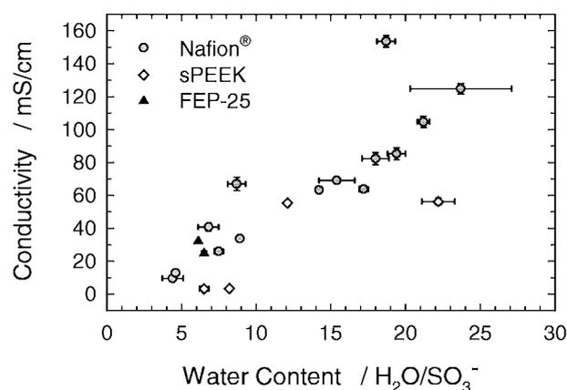
Fig. 2: Proton conductivity at room temperature as a function of water content. Nafion<sup>®</sup> data includes all Nafion<sup>®</sup> types investigated (cf. Experimental section).
