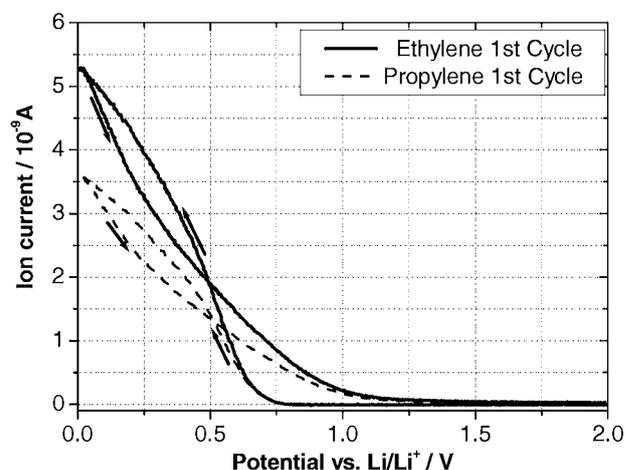
**Fig. 3:** DEMS measurements in TIMREX<sup>®</sup> SLX50 in 1 M  $\text{LiPF}_6$ , EC/PC 1/1 (w/w) electrolyte. Mass signals corresponding to ethylene ( $m/z=27$ ) and propylene ( $m/z=41$ ) are shown.
