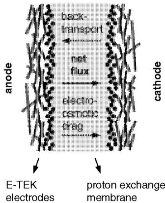
**Fig. 1:** Mechanisms for water transport in a fuel cell membrane:
