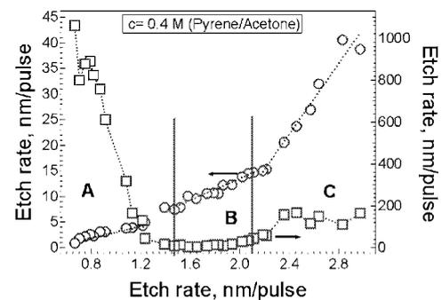
Fig. 1: Etch rate of quartz at different laser fluences.
