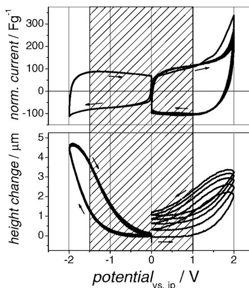
**Fig. 2:** CV (top) and simultaneous height change (bottom) of a 150  $\mu$ m thick supercap electrode. The SC operation window is indicated.
