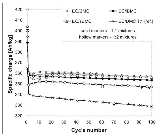
Fig. 1: Specific charge capacity (Li intercalation) in SFG44 half cells vs. metallic Li with isomeric BMC electrolytes containing 1M LiPF<sub>6</sub>.
