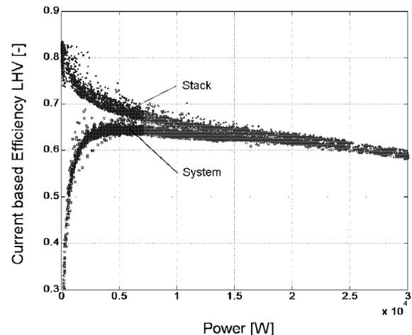
**Fig. 2:** Fuel cell stack and fuel cell system efficiency of the HY-LIGHT H<sub>2</sub>/O<sub>2</sub> fuel cell system as function of net power. Data obtained in car.
