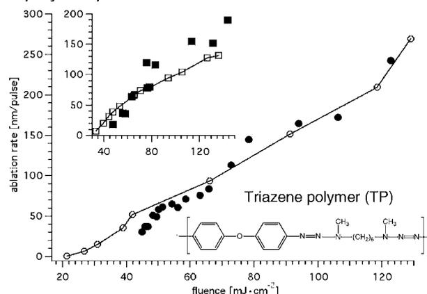
**Fig. 1:** Profilometric (●, ■) and gravimetric (○, □) measurement of the ablation rates of TP at irradiation wavelengths of 248 (■, □) and 308 nm (○, ●).
