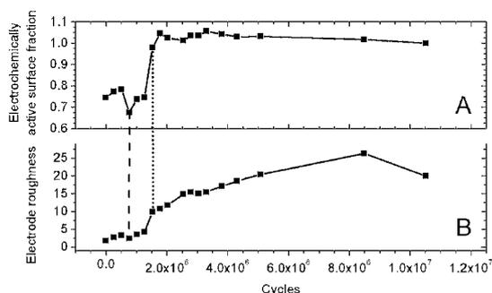
Fig. 1: Active surface fraction (A) and roughness (B).
