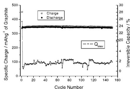
Fig. 1: Stable cycling of a SFG44 in EMI-TFSI – 1M  $LiPF_6$ – 5%VC.
