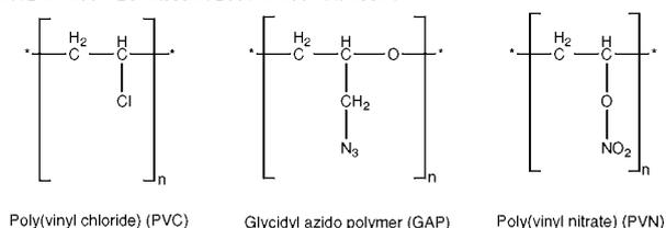
**Fig. 1:** Structure of PVC, GAP and PVN.
