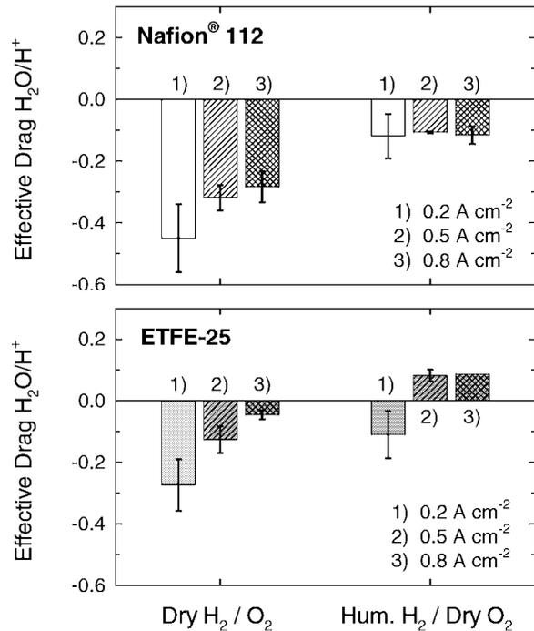
**Fig. 2:** Net water transport through 2 different fuel cell membranes. 30  $\text{cm}^2$  single cells with serpentine flow field, counter flow operation, 80  $^\circ\text{C}$  cell temperature,  $\text{H}_2/\text{O}_2$  gas flows 1.5 times stoichiometric, atmospheric pressure.
