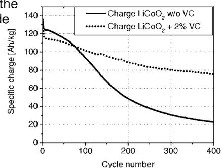
**Fig. 4:** Cycle stability of  $\text{LiCoO}_2$ , electrolyte EC/PC 1:1, 1M  $\text{LiPF}_6$  with and without additive.
