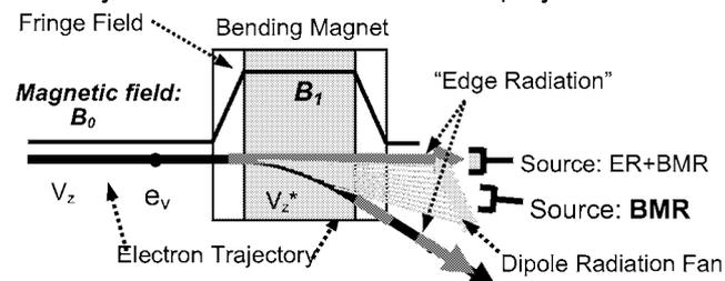
**Fig. 1:** Sketch of the two possible IR radiation sources: the bending magnet radiation (BMR) and the edge radiation (ER). The latter is always accompanied by some BMR.
