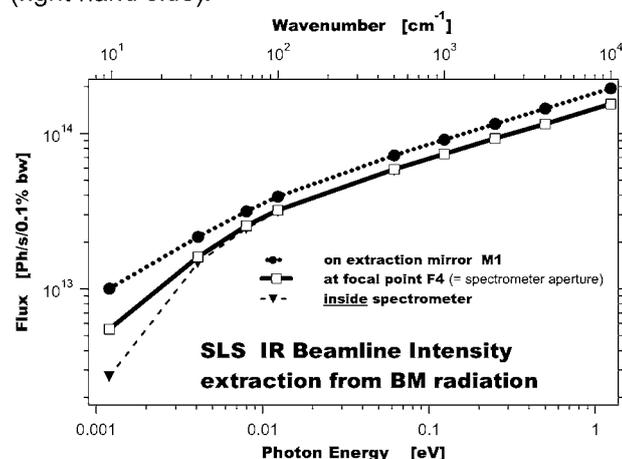
**Fig. 5:** Comparison of the extracted flux at the first mirror M1 (dots) with the propagated beam at last focal point F4 (squares) and with the flux inside the spectrometers (triangles).
