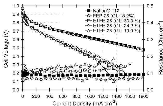
**Fig. 1:** Single cell performances of ETFE based membranes (carbon cloth electrodes) compared with Nafion® and FEP based membranes (carbon paper electrodes) (Pt loading of 0.6  $\text{mg cm}^{-2}$ ) at 80 $^{\circ}\text{C}$ .
