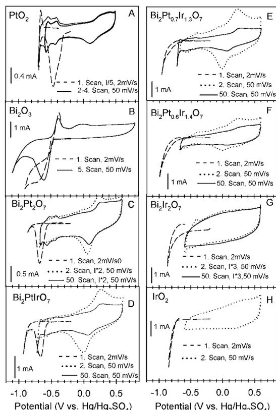
**Fig. 1:** CVs of metal oxide powders on graphite in Ar-saturated 0.5 M  $\text{H}_2\text{SO}_4$  at the indicated scan rates and current scales.
