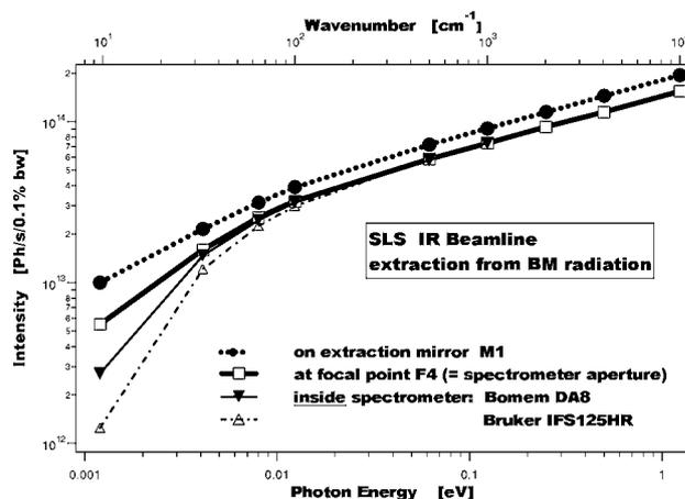
Fig. 1: Comparison of the extracted flux at the first mirror M1 (61(H) x 39(V)  $\text{mrad}^2$ ) with that at focal point F4 and with the flux inside different spectrometers.
