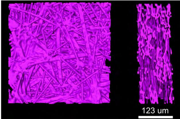
**Figure 2.** 3D surface of Toray TGP-H-060 without PTFE at a relative thickness of 0.62. The uncompressed thickness was 200  $\mu\text{m}$ . (All figures in color on-line)
