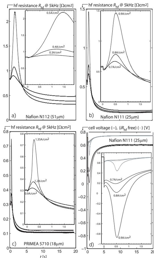
**Figure 1.** Integral transient response of the hf resistance (a-c) and cell voltage (d) (conditions as stated in Fig 1).
