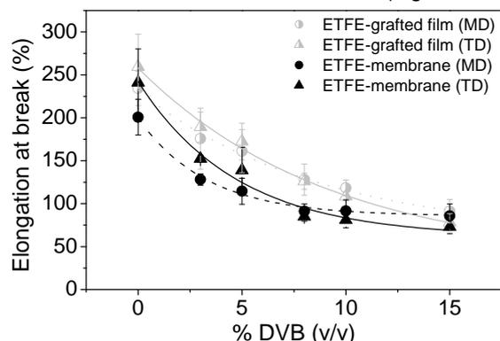
**Figure 1.** Elongation at break of the ETFE based grafted films and membranes in both directions (MD and TD) as function of the DVB concentration.
