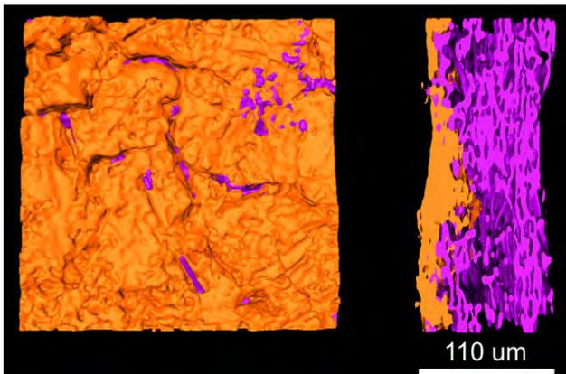
**Figure 4.** 3D surface of TGP-H-060 with 20% PTFE and MPL (orange phase) at a relative thickness of 0.48. The uncompressed thickness was 230  $\mu\text{m}$ .
