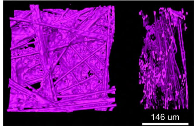
**Figure 5.** 3D surface of GDL24 from SGL without PTFE at a relative thickness of 0.85. The uncompressed thickness was 172  $\mu\text{m}$ .
