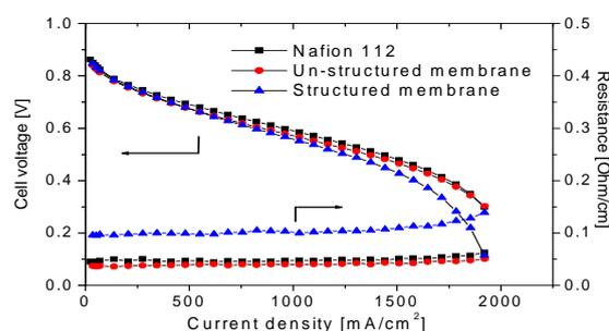
**Figure 2.** Single cell performance after 150 hours of a reference Nafion 112 membrane ■ and of a structured ▲ and an un-structured membrane •: 25  $\mu\text{m}$  ETFE exposed at ANKA and grafted with styrene/DVB achieving 35% of degree of grafting. Electrodes: E-TEK 0.6 mgPt cm<sup>-2</sup>, cell temperature: 80 °C, reactants: H<sub>2</sub>/O<sub>2</sub> at a stoichiometry of 1.5/1.5, gas pressure 1 bar, gases fully humidified.
