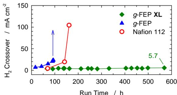
**Figure 1.** H<sub>2</sub> crossover, a measure for mechanical membrane integrity, is measured electrochemically in H<sub>2</sub> / N<sub>2</sub> mode.
