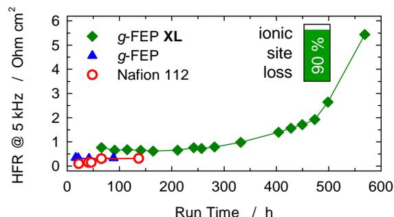
**Figure 2.** Chemical integrity of the membrane is measured via high frequency resistance (HFR).
