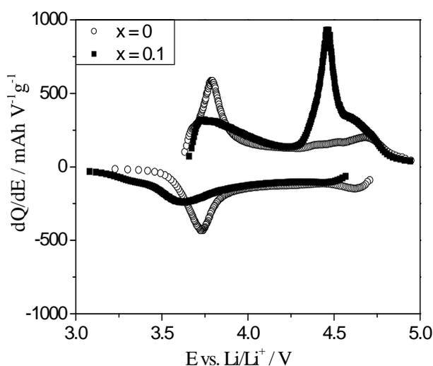
**Figure 2.** Differential plot for the  $\text{Li}_{1+x}(\text{Ni}_{1/3}\text{Mn}_{1/3}\text{Co}_{1/3})_{1-x}\text{O}_2$  ( $x = 0$  and  $x = 0.1$ , respectively) materials in the high voltage experiment in EC:DMC, 1 M  $\text{LiPF}_6$  (1<sup>st</sup> cycle).
