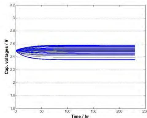
Figure 3. Evolution of single cell voltages in a SC module with 50 capacitors in series;  $C_i = 350 \pm 70$  F,  $R_i = 2500 \pm 500 \Omega$ .  $R_i$  is a function of the cell voltage. Same scale as Figure 2.
