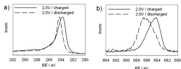
**Figure 2.** Comparison of the XP spectra obtained from the positive electrode in its charged and discharged state. a) C 1s signal  $\Delta E = 0.7$  eV; b) F 1s  $\Delta E = 2.0$  eV
