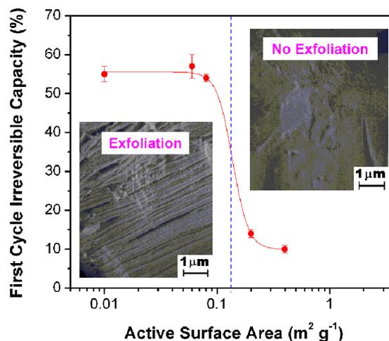
**Figure 1.** Irreversible capacities ( $C_{irr}$ ) for the first electrochemical Li<sup>+</sup> insertion into TIMREX<sup>®</sup> SLX50 negative electrodes as a function of the active surface area (ASA) measured at 10 mA g<sup>-1</sup> in a 1 M LiPF<sub>6</sub>, EC:DMC (1:1) electrolyte. Experimental data points and modified SEM images were obtained from Ref. [6].
