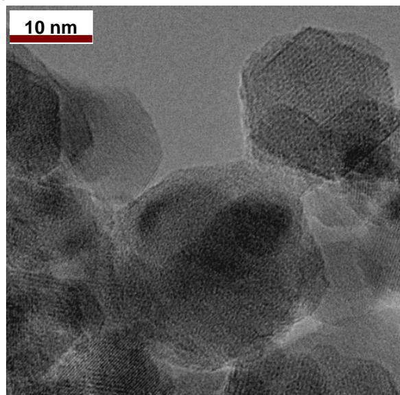
Figure 1. TEM of FSP-produced LiMn<sub>2</sub>O<sub>4</sub> nanoparticles.
