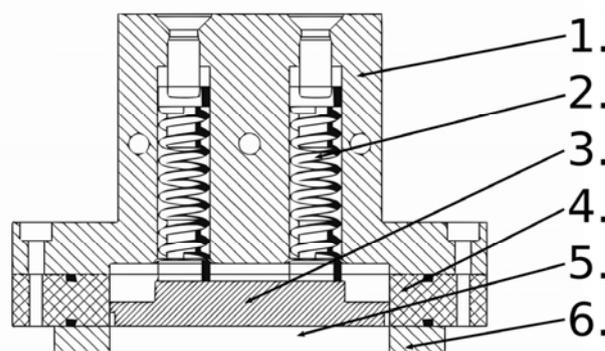
**Figure 1.** Schematic view of the *in situ* electrochemical cell. The elements of the device are: 1. Cell top, 2. Spring, 3. Negative current collector, 4. PEEK cell body, 5. Cavity for the electrode material, 6. Positive current collector.
