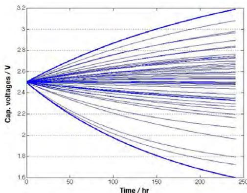
Figure 2. Evolution of single cell voltages in a SC module with 50 capacitors in series;  $C_i = 350 \pm 70$  F,  $R_i = 2500 \pm 500 \Omega$ .  $R_i$  is assumed to be constant.
