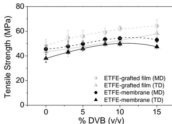
**Figure 2.** Tensile strength of ETFE-based grafted films and membranes in both directions (MD and TD) as function of the DVB concentration.
