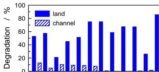
**Figure 2.** Local degradation analysis of an uncrosslinked PSI membrane operated at a current density of 2.25  $\text{A/cm}^2$  for 142 h.
