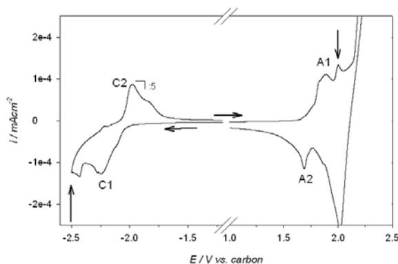
**Figure 1.** Current density potential curves of HOPG in 1M  $Et_4NBF_4/PC$ ;  $dE/dt = 10mV/s$ , anodic and cathodic scans were recorded separately, scan direction as indicated
