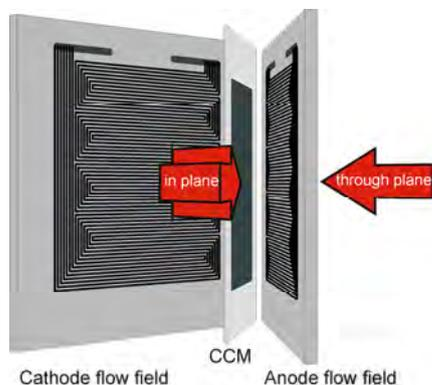
**Figure 1.** Two flow fields with a horizontal seven channel structure and a CCM in between. The arrows show the direction of the neutron beam.
