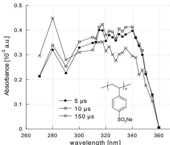
**Figure 1.** Time resolved absorption spectra of transients, normalized to 1 Gy, obtained from pulse irradiating 30  $\mu\text{M}$  poly(sodium styrene sulfonate) with polymerization degree  $n=6$ ,  $\text{N}_2\text{O}$ -saturated solution at pH 6.
