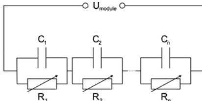
Figure 1. Sketch of a series connection of supercapacitors.
