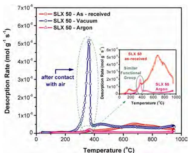
**Figure 2.** Desorption rate of CO gas as a function of temperature measured after oxygen chemisorption by temperature-programmed desorption (TPD) experiments for graphite samples of "SLX50 - As - received", "SLX50 - Vacuum", and "SLX50 - Argon". An enlarged plot of the circled dashed line is shown in the inset. A specific surface functional group is observed at 350 °C for all treated samples.
