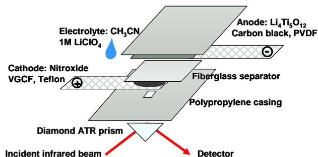
**Figure 2.** In-situ infrared cell on diamond ATR device.
