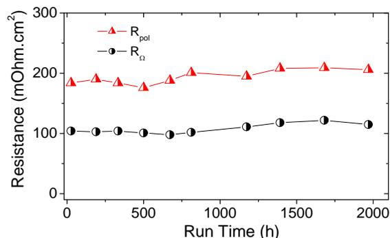
**Figure 2.** Extracted ohmic ( $R_{\Omega}$ ) and polarization resistance ( $R_{pol}$ ) from the EIS-spectra @500 $\text{mA}/\text{cm}^2$ .
