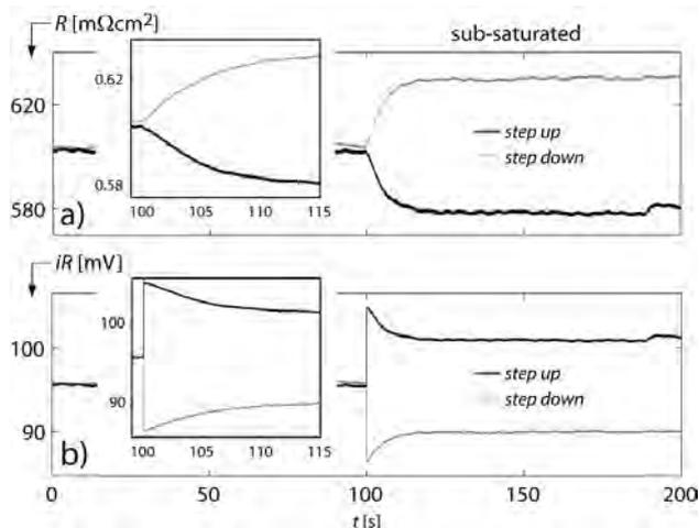
**Figure 2.** (a) Transient response of  $R$  and, (b) calculated  $iR$  drop (200pts/sec) for sub-saturated operation of the cell.
