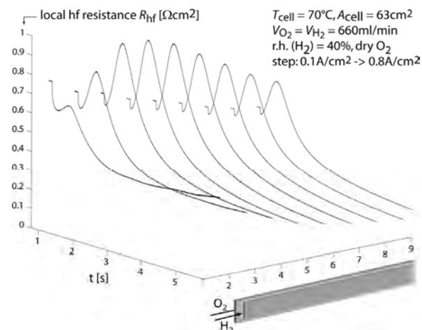
**Figure 1.** Local transient response of the hf resistance after a current step (MEA: Nafion 111, TKK 70%Pt/C).
