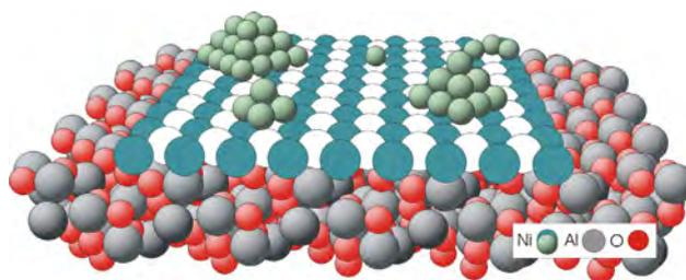
**Figure 2.** Suggested model of nickel deposition at the  $\gamma$ -Al<sub>2</sub>O<sub>3</sub> support with the “missing row” first layer
