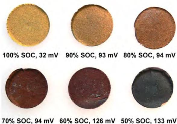
**Figure 1.** Graphite electrodes harvested from coin cells after intercalation of different amounts of lithium.
