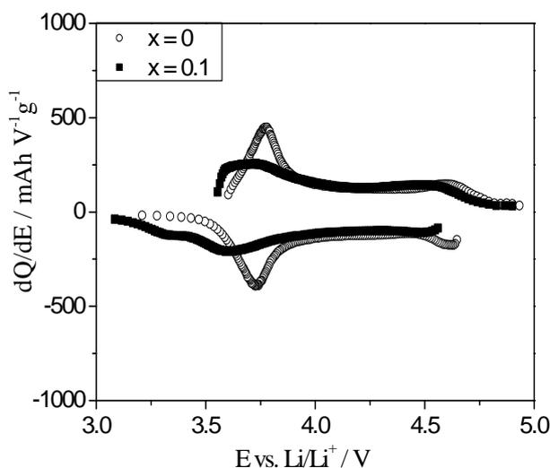
**Figure 3.** Differential plot for the  $\text{Li}_{1+x}(\text{Ni}_{1/3}\text{Mn}_{1/3}\text{Co}_{1/3})_{1-x}\text{O}_2$  ( $x = 0$  and  $x = 0.1$ , respectively) materials in the high voltage experiment in EC:DMC, 1 M  $\text{LiPF}_6$  (2<sup>nd</sup> cycle).
