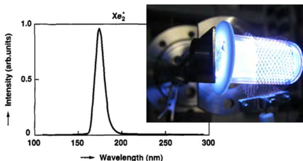
Figure 1. Emission spectrum and image of xenon excimer lamp
