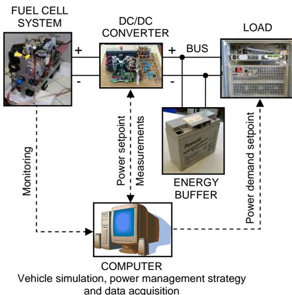
Figure 1. Experimental setup of the hardware in the loop test bench.
