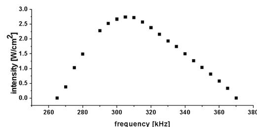
Figure 4. Lamp intensity versus frequency at 3 kV
