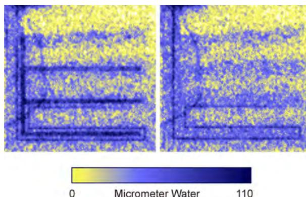
**Figure 2.** Radiograms (through plane) recorded at  $750 \text{ mA/cm}^2$  and a time difference of 12 minutes (left to right). The inner channel is completely filled with water (left), while it has been removed at once (right).
