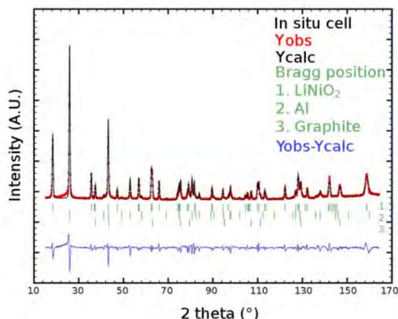
**Figure 4.** Neutron diffraction pattern of a  $\text{LiNiO}_2$  electrode measured in the in situ cell. The measurement was performed at a wavelength of 1.5 Å.
