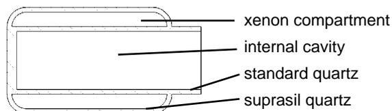
Figure 2. Cross section of excimer lamp tube
