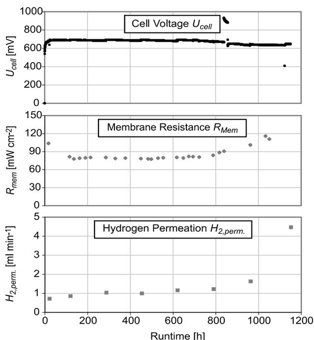
Figure 1. Measured cell voltage, membrane resistance, and hydrogen permeation as a function of time
