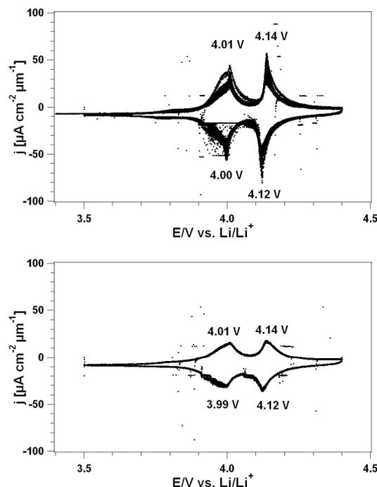
**Figure 1.** Typical cyclic voltammograms at  $0.05 \text{ mV s}^{-1}$  of thin films of  $\text{Li}_{0.87}\text{Mn}_2\text{O}_{3.47}$  after 20 (top) and 140 (bottom) cycles; 20 cycles are shown.
