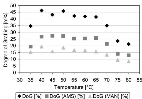
**Figure 2.** Dependency of the degrees of grafting, total, for AMS only, and MAN only, from the temperature after 48 h.
