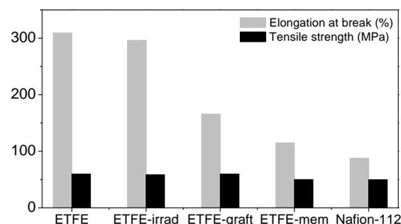
**Figure 3.** Comparison of the mechanical properties in MD of the ETFE base material with Nafion-112 based membrane during the overall process (irradiation, grafting and sulfonation).
