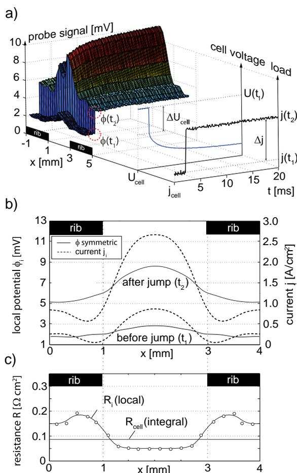
**Figure 1.** Principle of local resistance measurement: a) the channel-rib potential distribution is recorded during a perturbation of cell current, b) the distribution before and after the step is identified and the current is calculated, c) the resistance distribution  $R_i$  is obtained from  $\Delta U_{\text{cell}}$  and the local  $\Delta j_i$  during the step.
