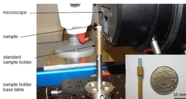
**Figure 1.** Endstation of X02DA TOMCAT beamline with sample holder, scintillator and CCD camera. The inset shows the specially designed sample holder.
