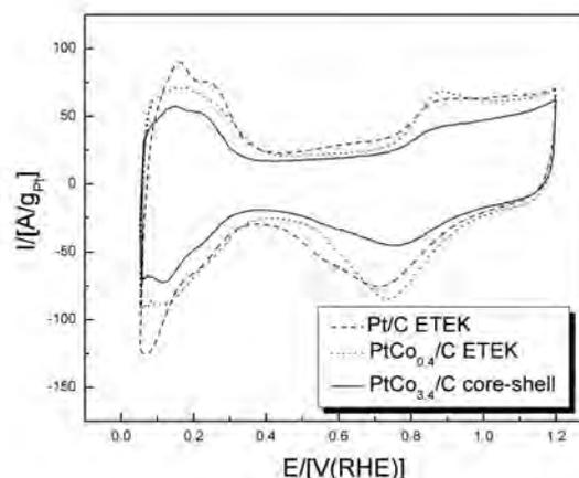
Figure 3. Cyclic voltammograms of commercial and PtCo<sub>3</sub>/C core-shell catalysts; Ar-saturated 0.1M HClO<sub>4</sub>, v=100mV/s, RT.
