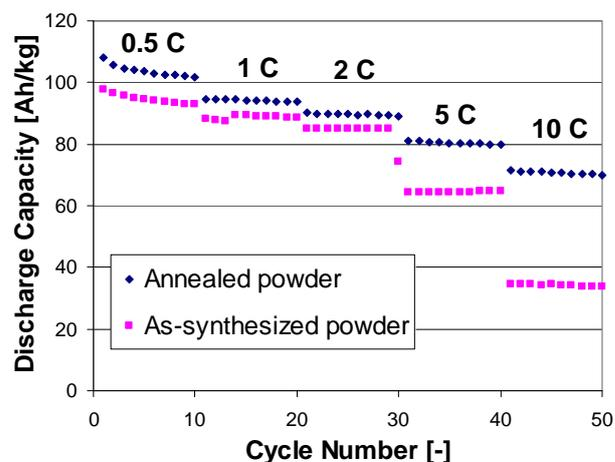
Figure 2. Galvanostatic cycling capacity of the FSP-produced LiMn<sub>2</sub>O<sub>4</sub> nanoparticles at various C-rates between 3.5 and 4.3 V vs Li. Capacity is expressed per kg of LiMn<sub>2</sub>O<sub>4</sub>. 1C = 148 A kg<sup>-1</sup>.
