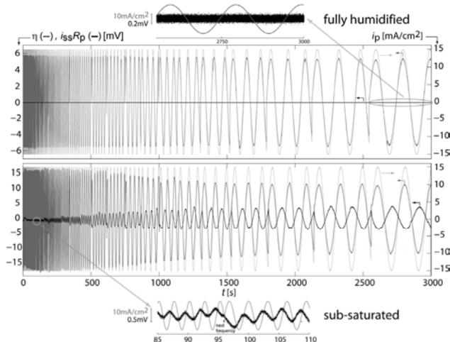
**Figure 3.** AC perturbation current  $i_p$ , ac cell voltage  $\eta$  and ac voltage  $i_{ss}R_p$  caused by variation of  $R$  ( $1\text{Hz} \leq f \leq 5\text{mHz}$ ).
