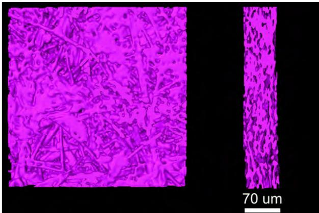
**Figure 3.** 3D surface of TGP-H-060 from Toray without PTFE at a relative thickness of 0.35. The uncompressed thickness was 200  $\mu\text{m}$ .
