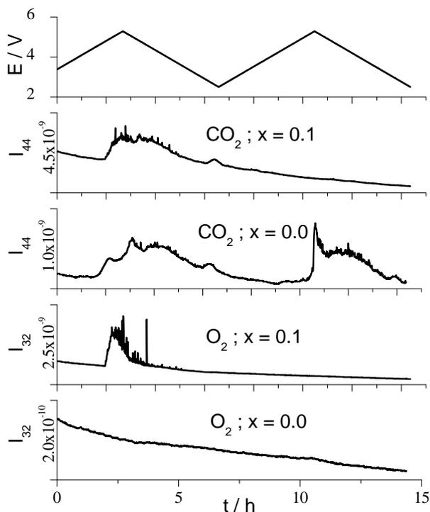
**Figure 4.** Plot of mass signal intensities  $I_{m/z}$  [ $A g^{-1}$ ] for  $Li_{1+x}(Ni_{1/3}Mn_{1/3}Co_{1/3})_{1-x}O_2$  ( $x=0$  and  $x=0.1$ , respectively) normalized in respect to the oxide mass;  $E$  is the potential vs.  $Li/Li^+$  [V].
