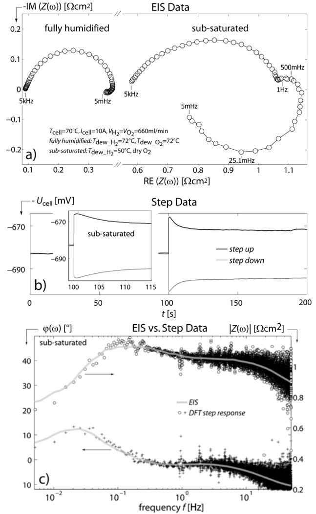
Figure 1. (a) EIS data ( $5\text{mHz} \leq f \leq 5\text{kHz}$ , 10pts/sec), (b) transient response cell voltage, (c) Fourier transformed step data vs EIS.
