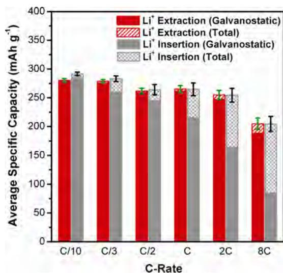
**Figure 3.** The average (over 10 cycles) specific capacities of the  $\text{Li}_4\text{V}_3\text{O}_8$  electrodes cycled between 2.0 and 4.0 V at different specific currents (C-rate). Note that 1C rate is assumed to be  $350 \text{ mA g}^{-1}$  in all cases.
