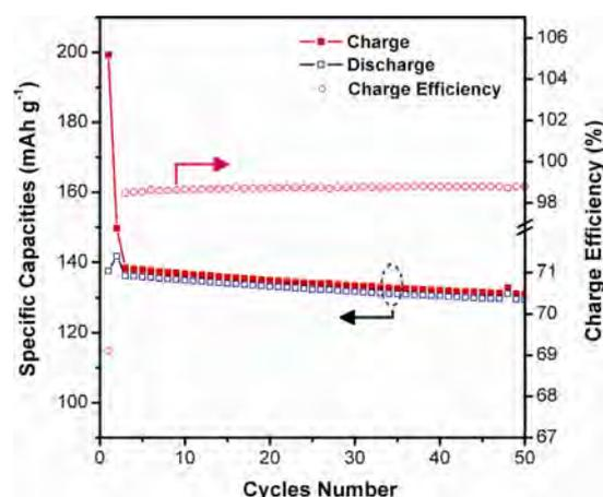
**Figure 4.** Cycle life behaviour of the  $\text{Li}_4\text{V}_3\text{O}_8$  cathode in a full cell (vs. graphite LBG1025), where cycling took place between 1.6 and 4.0 V at  $117 \text{ mA g}^{-1}$ .
