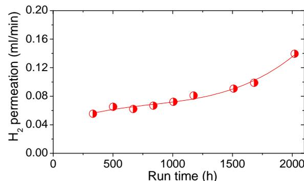
**Figure 3.** Hydrogen crossover measured in  $\text{H}_2/\text{N}_2$  mode.
