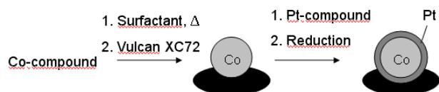
Figure 1. Preparation of core-shell PtCo<sub>3</sub>/C catalysts
