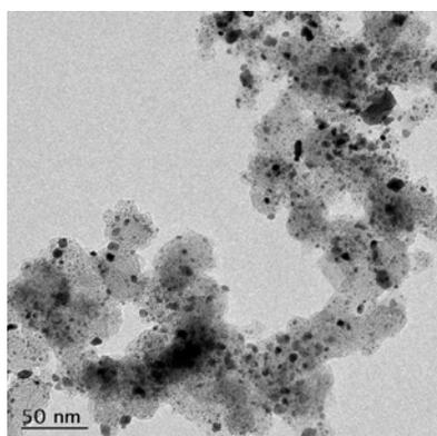
Figure 2. TEM image of core-shell PtCo<sub>3</sub>/C
