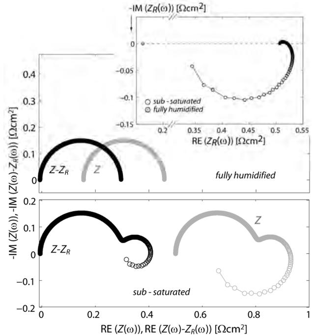
**Figure 1.** Integral cell impedance  $Z$ , membrane impedance  $Z_R$  and ' $Z_R$  -corrected' impedance  $Z - Z_R$  ( $4.2 \text{ mHz} < f < 833\text{Hz}$ ) for fully humidified and sub-saturated cell operation [1].
