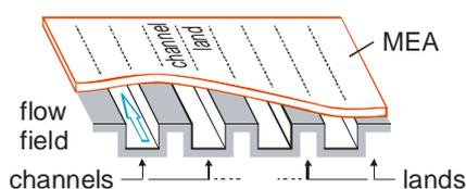
**Figure 1.** Schematic of the single cell configuration. The membrane electrode assembly (MEA) is sandwiched between two flow field plates (only bottom plate shown) for distribution of reactant gases through channels and current collection via lands.
