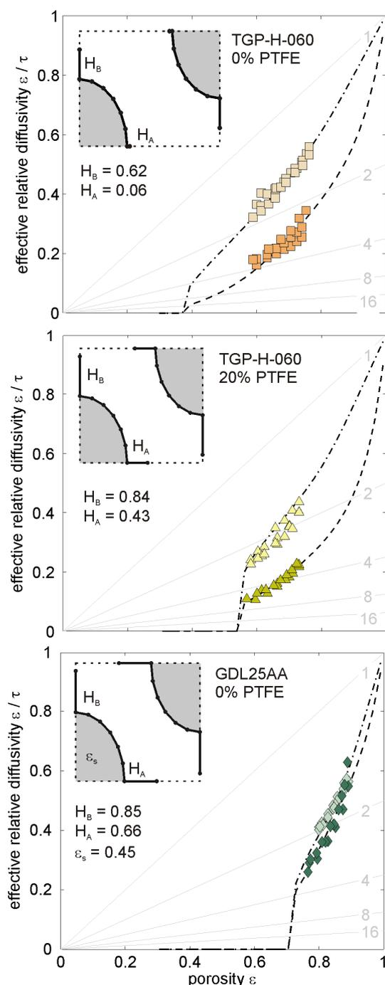
**Figure 1.** Unit cell and measured diffusivities as a function of porosity. Dashdotted lines represent *ip* and dashed lines *tp* diffusivities of the unit cell. The insets show the real, uncompressed unit cell configuration. The gray lines are isotropy levels.
