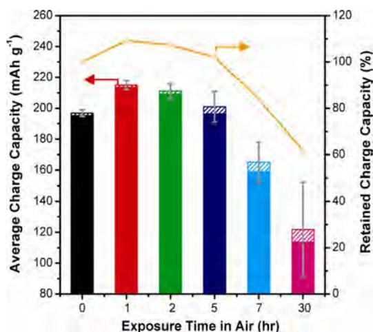
**Figure 2.** The average (over 10 cycles) and percentage of retained charge capacities of the  $\text{Li}_4\text{V}_3\text{O}_8$  electrodes after exposure to ambient air for various lengths of time, where cycling took place between 2.0 and 3.3 V at the C/3 rate. The solid columns represent the galvanostatic part of the total capacities, while the patterned columns indicate the contribution from the potentiostatic part of the total capacities.
