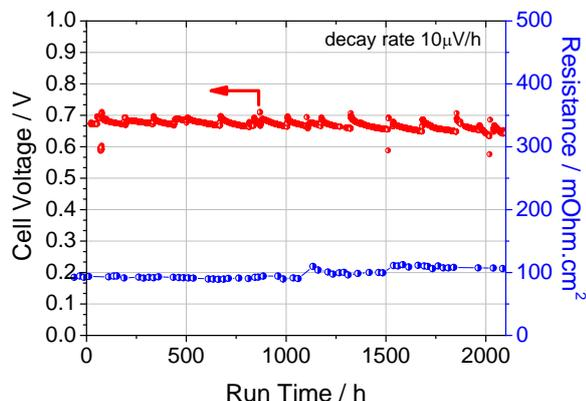
**Figure 1.** Single cell durability test using a radiation grafted membrane based on ETFE (5% DVB) @500 $\text{mA}/\text{cm}^2$ , cell temperature 80°C;  $\text{H}_2/\text{O}_2$  at a stoichiometry of 1.5/1.5.
