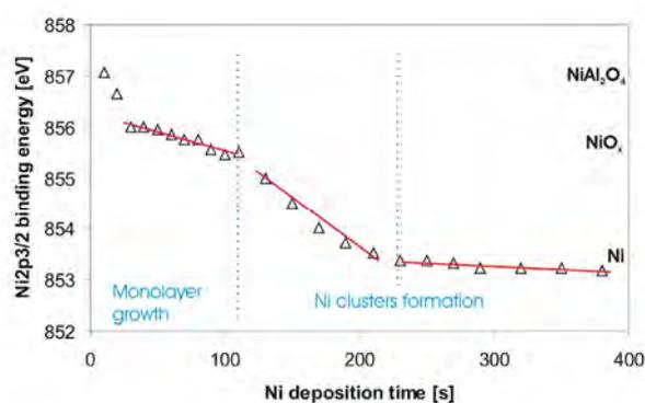
**Figure 3.** Changes of BE Ni 2p<sub>3/2</sub> during nickel deposition on Al<sub>2</sub>O<sub>3</sub> model catalysts: XPS studies.
