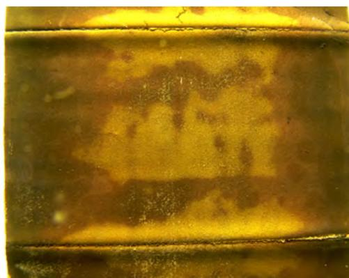
**Figure 3.** Anode of a commercial high-power cell after 1500 cycles at 6C rate.
