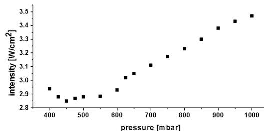
Figure 3. Lamp intensity versus xenon pressure
