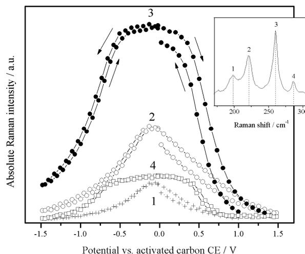
Figure 2. Intensity variation of RBM bands during cycling.
