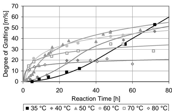
**Figure 1.** Evolution of the degree of grafting at different grafting temperatures (lines as an assistance).
