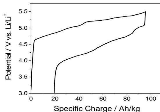
Figure 1. Electrochemical cycling of graphite in 1 M  $\text{LiPF}_6$ , EC:DMC (1:1) electrolyte.
