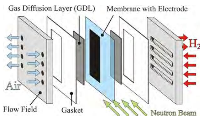
**Figure 1.** Design of the fuel cell for in plane imaging (active area is 0.5 cm<sup>2</sup>). For the sake of simplicity the cell housing is not shown here.
