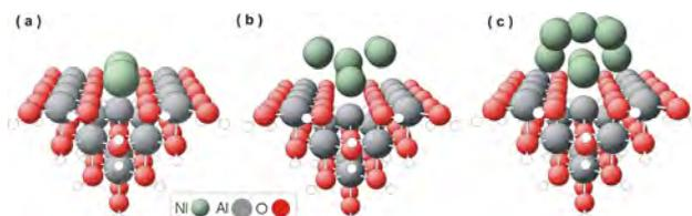
**Figure 1.** Ni<sub>x</sub> model clusters: (a) Ni<sub>2</sub>, (b) Ni<sub>7</sub>, (c) Ni<sub>9</sub> deposited at (100)  $\gamma$ -Al<sub>2</sub>O<sub>3</sub> represented by Al<sub>15</sub>O<sub>40</sub>H<sub>35</sub> cluster.
