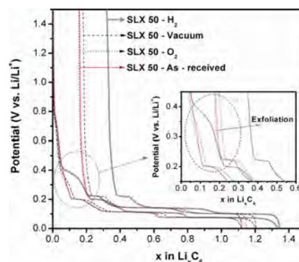
**Figure 3.** First electrochemical Li<sup>+</sup> insertion/de-insertion into TIMREX® SLX50 negative electrodes measured at 10 mA g<sup>-1</sup> in a 1 M LiPF<sub>6</sub>, EC:DMC (1:1) electrolyte. An enlarged plot of the circled dashed line is shown in the inset. Exfoliation was observed for both hydrogen- and vacuum-treated graphite samples.
