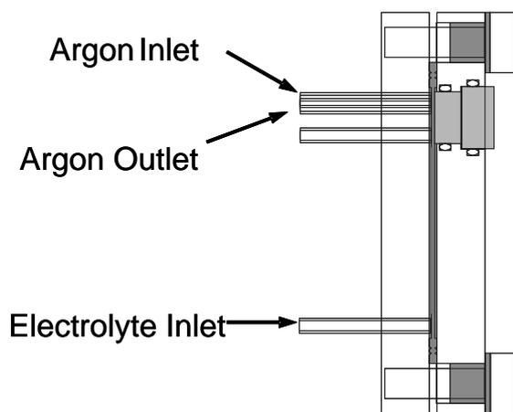
**Figure 1.** Cell design for Differential Electrochemical Mass Spectrometry experiments.
