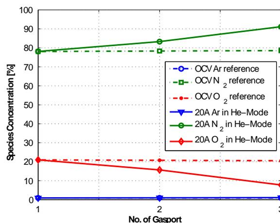
**Figure 1.** Species concentration along the cathode channel determined by *in-situ* mass spectrometry. Cathode: air,  $T_{dp}=60^{\circ}\text{C}$ ,  $\lambda=2$ ,  $p=1.5$  bar; Anode: hydrogen,  $T_{dp}=60$ ,  $\lambda=1.5$ ,  $p=1.5$ bar;  $T_{cell}=75^{\circ}\text{C}$ .
