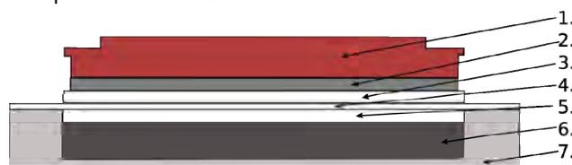
**Figure 2.** Schematic view of the electrode assembly. 1. Copper current collector, 2. Metallic lithium strip, 3. Glass fiber separator, 4. Polymeric separator, 5. Glass fiber separator, 6. Active material powder, 7. Positive current collector.
