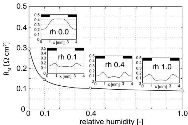
**Figure 2.** Integral ohmic resistance and local resistance distributions (insets, ribs pointed out by black bars) for different humidities of both electrodes; cell operated on  $\text{H}_2/\text{Air}$ , 70°C, 1.5  $\text{bar}_{\text{abs}}$ .
