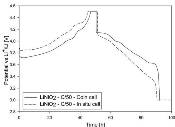
**Figure 3.** Comparison between the electrochemical performance of the neutron cell (dashed line) and a coin-like cell (solid line). Both cells were cycled at a C/50 rate against a metallic lithium counter electrode. The electrolyte was a 1:1 (wt.%) mixture of ethylene carbonate and dimethylcarbonate with 1M  $\text{LiPF}_6$ .
