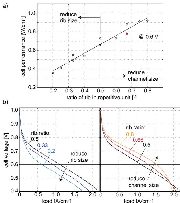
**Figure 1.** Correlation of channel-rib sizing and integral cell performance, H<sub>2</sub>/O<sub>2</sub>, rh = 0.4, 70°C, 1.5 bar<sub>abs</sub>, a) integral cell performance as a function of the rib ratio, potentiostatic operation at 600 mV; b) U-I-curves for selected flow field geometries with reduced rib sizes (left diagram) and reduced channel sizes (right diagram).
