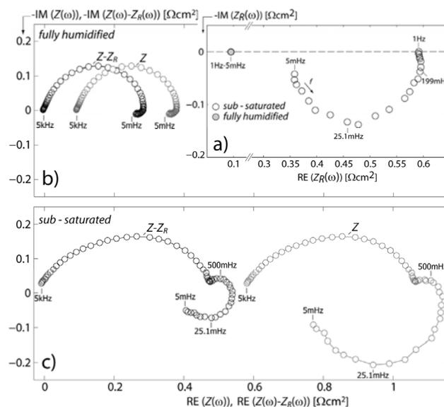
**Figure 4.** (a) Spectra for  $Z_R(\omega)$  (measure for membrane impedance) and, (b,c) original and  $Z_R(\omega)$ -corrected spectra.
