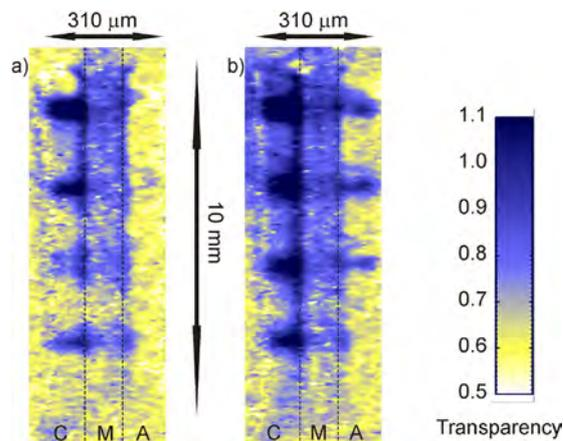
**Figure 3.** Radiograms (in plane) recorded at  $250$  (a) and  $750 \text{ mA/cm}^2$  (b). On the cathode side, a water layer is visible at the boundary of cathode flow field (C) and membrane (M).
