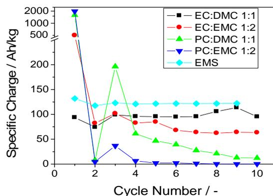
Figure 2. Cycling behavior (charging steps only) of graphite in the high potential region (3.0 – 5.5 V vs.  $\text{Li/Li}^+$ ) in different electrolytes.
