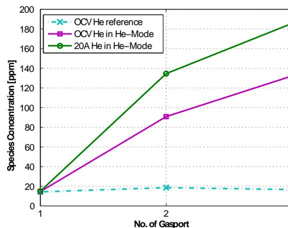
**Figure 2.** Helium concentration along the cathode channel determined by *in-situ* mass spectrometry. Anode side helium addition 5.2%. Cathode:  $T_{dp}=60^{\circ}\text{C}$ ,  $\lambda=2$ ,  $p=1.5$  bar; Anode:  $T_{dp}=60$ ,  $\lambda=1.5$ ,  $p=1.5$ bar;  $T_{cell}=75^{\circ}\text{C}$ , 5.2% dry helium addition.
