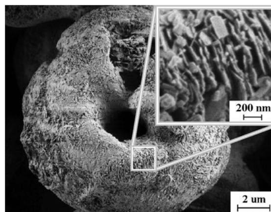
**Figure 1.** SEM image of the as-synthesized Li<sub>4</sub>V<sub>3</sub>O<sub>8</sub> material, with the inset showing the presence of rod-like nanostructures as the building block for the spherical agglomerates.
