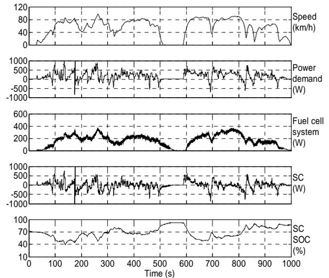
Figure 2. Simulation of light duty vehicle (1600 kg) driving outer-urban cycle. Scaled HiL powertrain: fuel cell 1 kW and 8 x 2.5V/1200F supercapacitors (SC).
