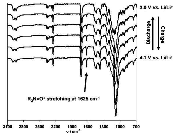
**Figure 3.** Infrared spectra of a cathode made from PTMA as a function of state of charge.
