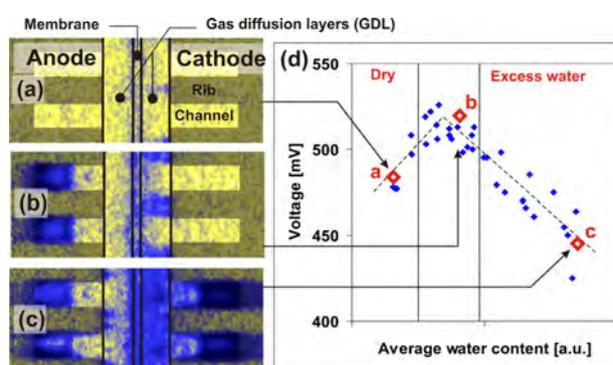
**Figure 2.** (a-c) In plane Neutron Radiograms of a PEFC showing the water distribution at 1A/cm<sup>2</sup> for different inlet relative humidities at the anode/cathode: (a) 60% / 0% (b) 110% / 40% (c) 90% / 110%; (d) relationship between average water content and cell performance.
