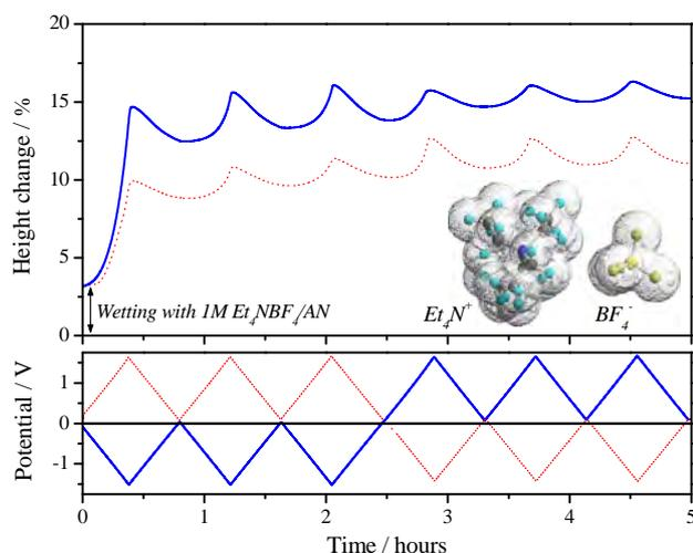
Figure 1. *In situ* dilatometry of SWCNTs during potential sweeps.
