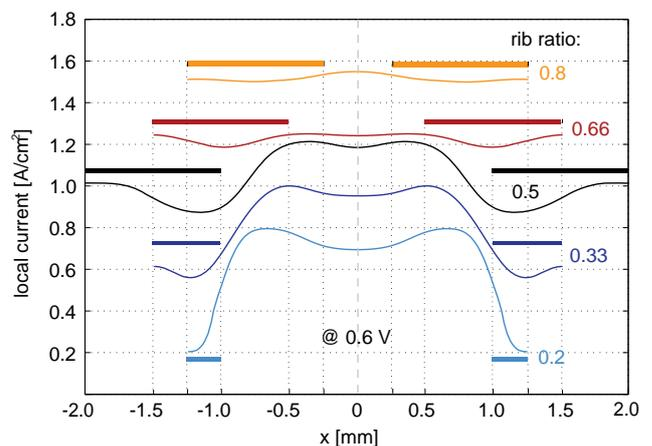
**Figure 2.** Locally resolved current distributions across two repetitive flow field units (1 channel and 2 adjacent half-ribs) for the 5 cells from Figure 1b), the rib areas are marked with bars, potentiostatic operation at 600 mV.
