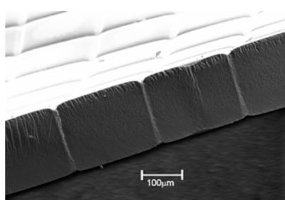
**Figure 1.** Cross-section of a structured proton-conducting membrane produced by exposing an ETFE film through a 85  $\mu\text{m}$  thick Ni-grid with 15  $\mu\text{m}$  features (90% opened area), followed by grafting of styrene and sulfonation.
