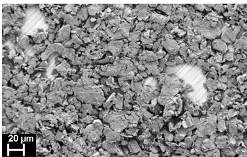
**Figure 1.** SEM picture of a typical graphite thin electrode, light gray: copper current collector, dark gray: graphite particles, SuperP has not been added for clarity
