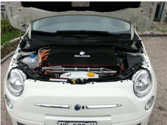
Figure 1. Top: Fiat 500 electric; bottom: integration of fuel cell system in front motor compartment.
