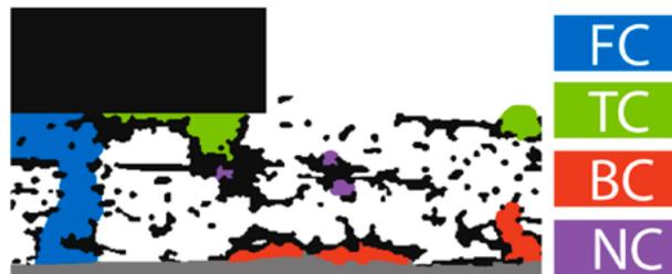
**Figure 1.** Sketch of the different cluster types that can be found in the GDL domain; blue: full connected water clusters (FC); green: top connected (TC); red: bottom connected (BC); purple: non connected (NC); rib domain and GDL fibers are shown in black, catalyst layer and membrane are shown in gray. Reproduced from [7] published under CC BY-NC-ND (<http://creativecommons.org/licenses/by/4.0/>).
