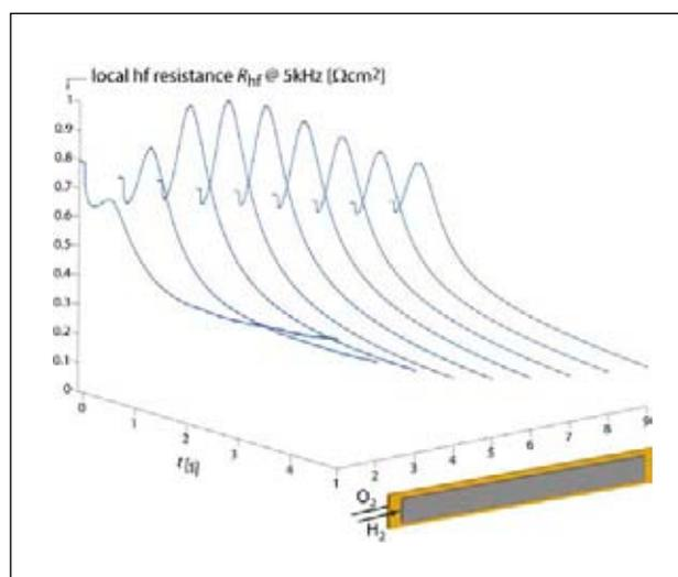
Figure 3: **Locally resolved (9 segments, 63 cm<sup>2</sup> active area) transient response of the hf resistance (5 kHz) in a nine-fold segmented PEFC with linear flow field, after a stepwise increase in current from 0.1 to 0.8 A/cm<sup>2</sup>.**
