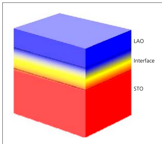
Figure 1: **Schematic of the ultrathin conducting interfacial sheet in between the insulating materials  $\text{LaAlO}_3$  and  $\text{SrTiO}_3$ .**
