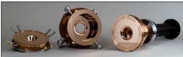
Figure 4: 1.5 GHz 2 cell cavity before assembly for low power test.
