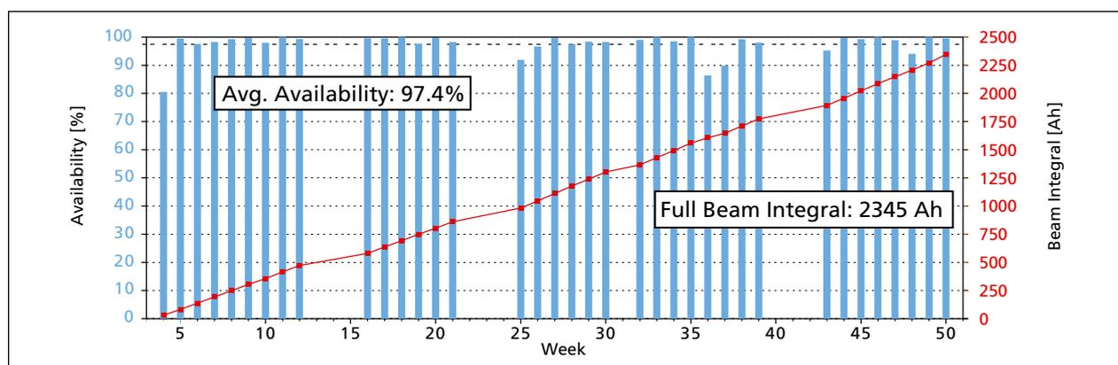
Figure 1: SLS operation statistics: weekly availability and integrated beam dose.
