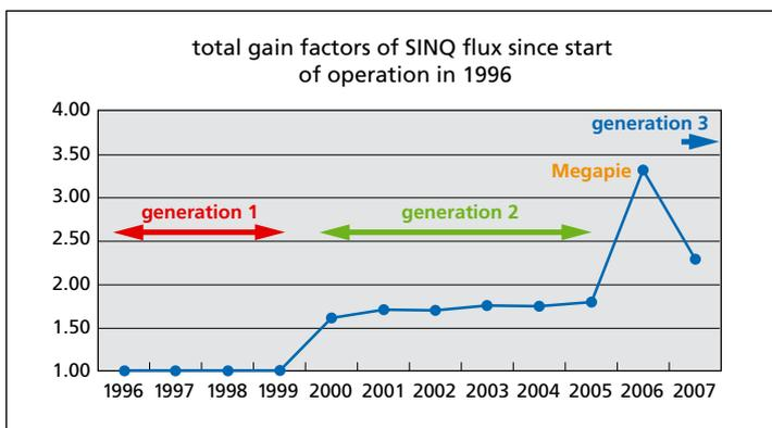
Figure 1: **Development of the neutron flux at SINQ since the start of operations. The gain is caused by both neutron target development and an increase of the accelerator's proton current.**
