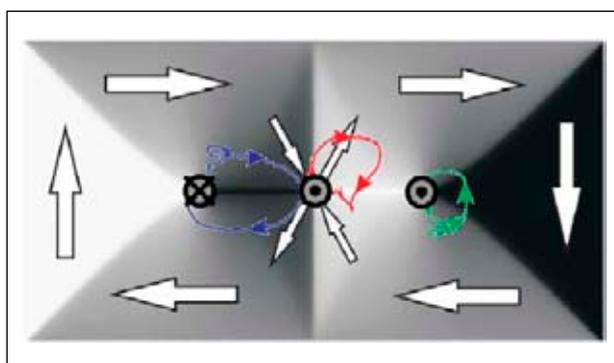
Figure 3: Domain pattern of a platelet containing a cross-tie wall taken from a simulation. The white arrows indicate the local direction of the magnetization. Coloured arrows indicate the trajectories of the three vortices following the excitation by a field pulse. The cores are oriented down – up – up ( $\otimes \odot \odot$ ).
