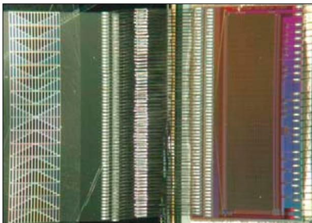
Figure 1: Pixel array of profile monitor (left) with bond wires (centre) and APC128 read-out chip.
