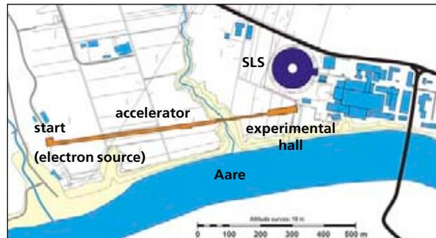
Figure 6: Planned infrastructure for the PSI-XFEL shown in Figure 5.
