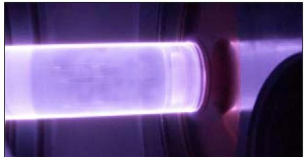
Figure 2: **Glow discharge, used for high-voltage, high-gradient commissioning of the 500 kV pulser.**
