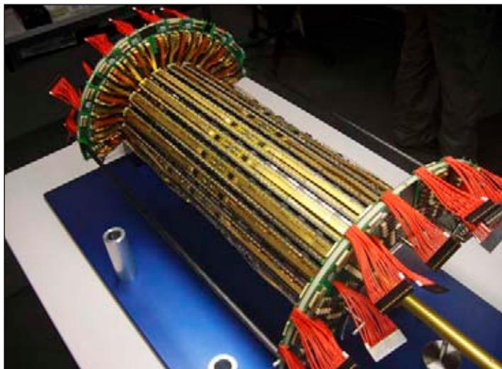
Figure 3: View of one of the two completed half barrel pixel detectors.
