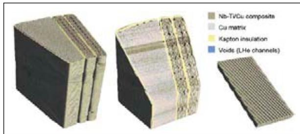
Figure 1: Tomograms of two insulated cables removed from an inner LHC magnet coil and a nude 01 LHC cable (right). The Rutherford cable with a width of 15.1 mm and a mid-thickness of 1.896 mm is composed of 28 strands with a nominal diameter of 1.065 mm.
