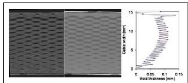
Figure 3: Plane maps of the neutron absorption contrast in a centre sagittal cable slice (left) and a stack of the 60 central cable slices (centre). The grey values were converted into a void thickness scale (right). The total void cross section is only 4 % of the entire cross section.
