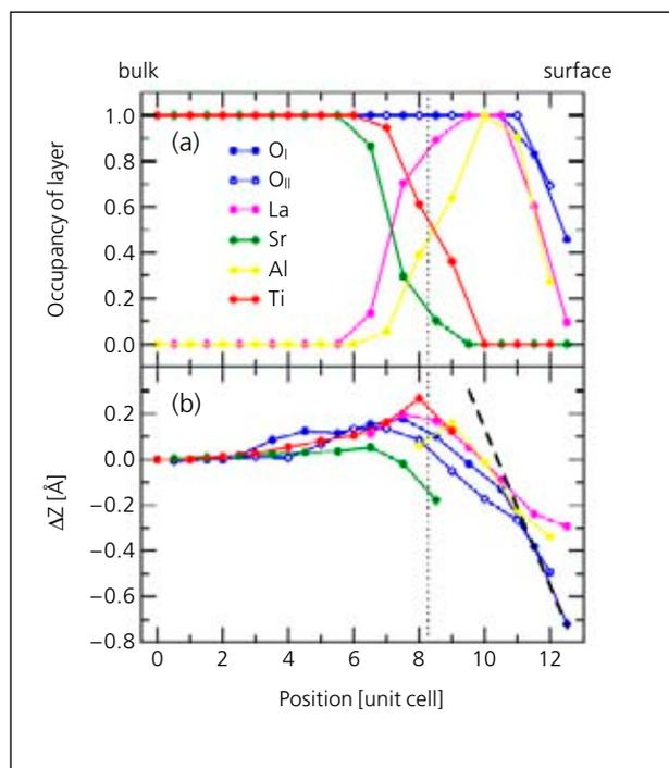
Figure 2: **(a) The chemical composition of the STO/LAO structure across the interface. The transition from STO to LAO is not abrupt, but extends over approximately three monolayers. (b) The positions of the atoms in the direction perpendicular to the interface  $z$  relative to the positions of atoms in bulk STO. Note the dilation as the nominal interface (dotted vertical line) is approached.**
