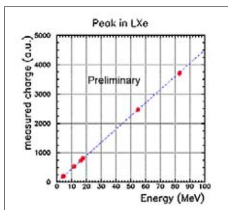
Figure 3: Calorimeter response to different  $\gamma$ -lines, e.g. C-W Li & B targets: with Li at 14.6, 17.6 MeV & B at 4.4, 11.7 & 16.1 MeV as well as CEX photons at 55, 83 MeV
