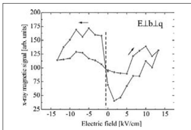
Figure 3: **X-ray difference intensity  $\Delta I$  as function of the applied electric field at  $T = 38.5 \text{ K}$ , showing its hysteretic behavior.**
