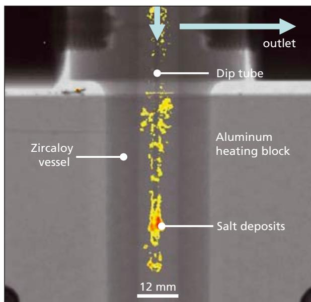
Figure 2: **Build-up of solid  $\text{Na}_2\text{SO}_4$  around the dip tube inside the separator, finally leading to a vessel blockage (405 °C, 30 MPa; Feed:  $\text{Na}_2\text{SO}_4 + \text{Na}_2\text{B}_4\text{O}_7$  in  $\text{D}_2\text{O}$ ; 15 s shutter time).**
