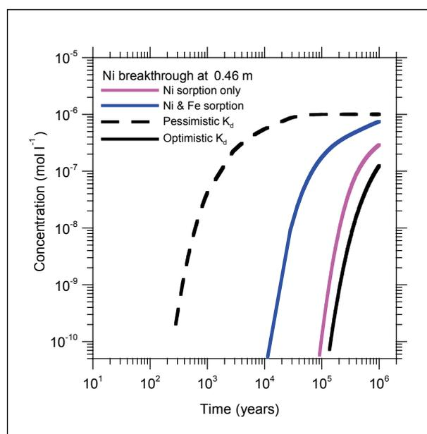
Figure 3: **Calculated  $\text{Ni}^{2+}$  concentration at the bentonite buffer/host rock interface. Sorption of Ni(II) is described by multi-species reactive transport, including mechanistic sorption models. A second calculation accounts for the effects of sorption competition between Ni and Fe. The results from calculations based on the simple  $K_d$  approach using bounding pessimistic and optimistic  $K_d$  values for Ni(II) are also shown.**
