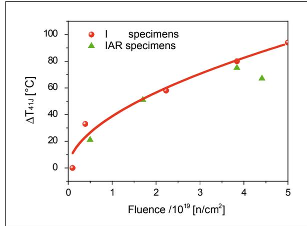
Figure 3: The shift  $\Delta T_{41j}$  of the transition temperature vs. fluence for the I and IAR specimens.
