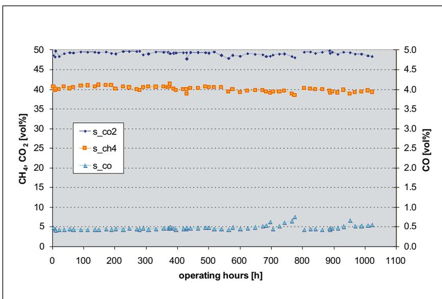
Figure 1: PSI 10 kW scale test facility (inside white container) at the industrial wood gasifier in Güssing/Austria (left), concentrations of methane and carbon oxides during the 1000h test (right)
