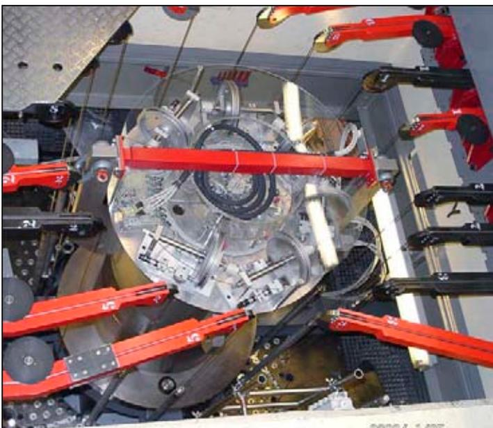
Figure 1: The shielding flask and sample changer on top of the PROTEUS reactor
