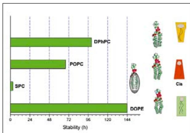
Figure 4: Stability of bilayers of different compositions on 800 nm pores. The space filling models of the lipid molecules Di-phytanyl- phosphatidylcholine (DPhPC), POPC, SPC and Di-oleoyl-PC (DOPE) and their shapes (side view) are shown. Threshold was set to 1 MΩ.
