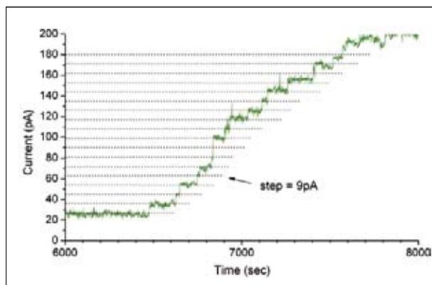
Figure 6: Insertion of hemolysin molecules results in the formation of protein pores, detected as step-wise increase of the current.
