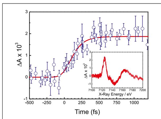
Figure 4: **Femtosecond X-ray absorption time scan performed at 7126 eV. Red line: a fit using a model taking into account the energy pathway shown in Figure 3. Inset: Transient X-ray absorption measured at 50 ps after excitation [4].**
