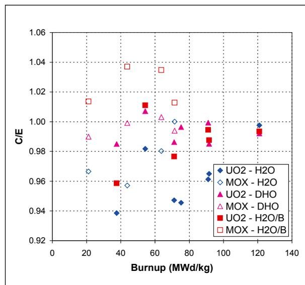
Figure 2: Calculated-to-experimental (C/E) ratios for the reactivity worths of the burnt samples vs. burnup (DHO =  $D_2O/H_2O$  mixture, H2O/B = borated  $H_2O$ )
