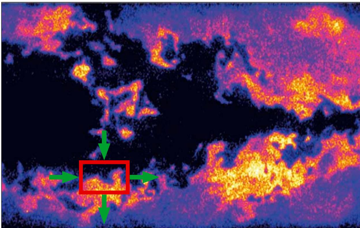
Figure 1: **The combination of laser induced fluorescence with particle induced velocimetry provides access to the local heat balance. In developing methods for the efficient, low NO<sub>x</sub> combustion of synthesis gas, this information is important to assess flame stability and to suppress thermoacoustic oscillations.**
