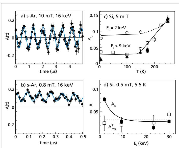
Figure 1: a) Typical LE- $\mu$ SR asymmetry  $A(t)$  of  $\text{Mu}^+$  (diamagnetic signal) in solid Argon, and b), corresponding low-field  $\text{Mu}^0$  precession which is 103 times faster. c) Undoped Si <100>,  $\text{Mu}^+$  asymmetry  $A_D$  as a function of temperature and energy. d)  $\text{Mu}^+$  and  $\text{Mu}^0_T$  asymmetries versus energy. The lines in a) and b) are fits, and in c) and d) guides to the eye.
