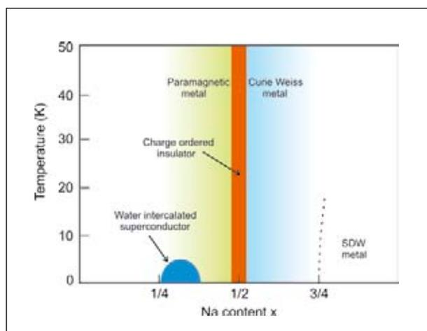
Figure 1:  $\text{Na}_x\text{CoO}_2$  phase diagram (after Foo et al. [4])
