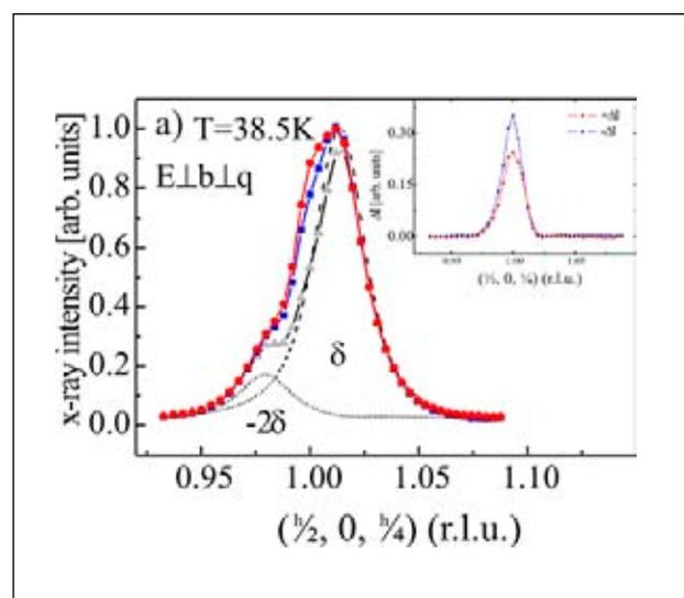
Figure 1: The  $(\frac{1}{2} 0 \frac{1}{4})$ -reflection of  $\text{ErMn}_2\text{O}_5$  taken at the Mn  $L_3$ -edge above  $T_{CM}$ .  $\delta$  corresponds to a magnetic reflection,  $-2\delta$  to an induced aspheric charge reflection. The inset shows the intensity difference  $\Delta$ .
