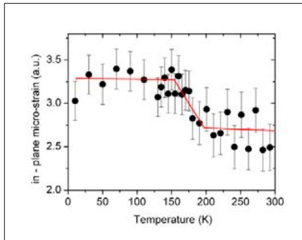
Figure 3: **Temperature dependence of the in-plane micro strain in  $\text{Na}_{0.8}\text{CoO}_2$  as determined by high resolution neutron diffraction experiments. The increase below 200 K can be related to the sodium ordering.**
