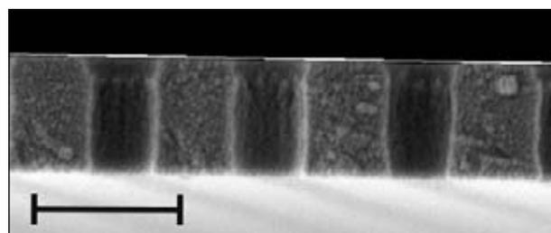
Figure 2: **Silicon nitride nanopore membrane as support for lipid bilayers (white line), shown in detail in Fig. 1. Side view, scale bar is 400 nm.**
