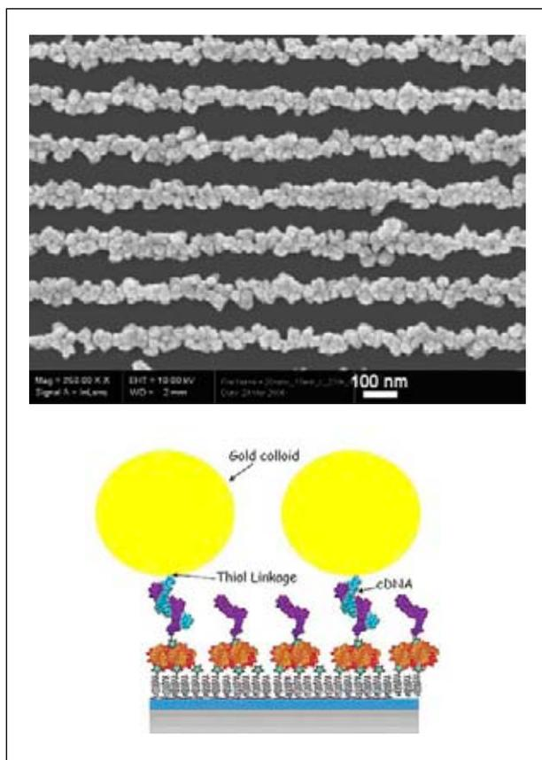
Figure 2: **Gold colloid nanowires were formed on a Nb<sub>2</sub>O<sub>5</sub> substrate: DNA-tagged gold particles were linked to the PLL-g-PEG/PEG biotin surface by neutravidin/biotin linkage.**
