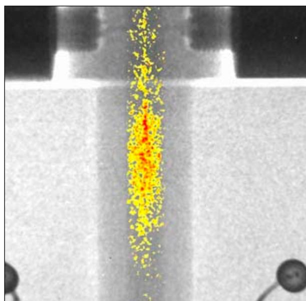
Figure 3: **Snapshot of the distribution of  $\text{H}_2\text{O}$  injected as a tracer pulse into the high pressure separator filled with  $\text{D}_2\text{O}$  (400 °C, 30 MPa; 1 s shutter time).**
