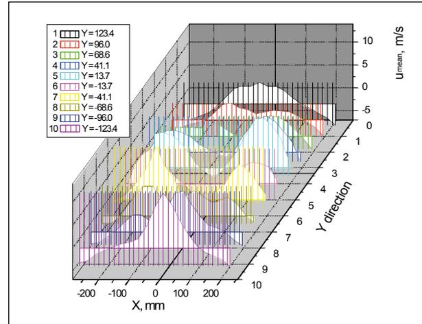
Figure 3: Vertical velocity profiles in the tube bundle.
