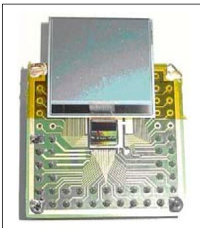
Figure 1: **Test structure with the Si-microstrip detector bonded to the MYTHEN readout ASIC.**
