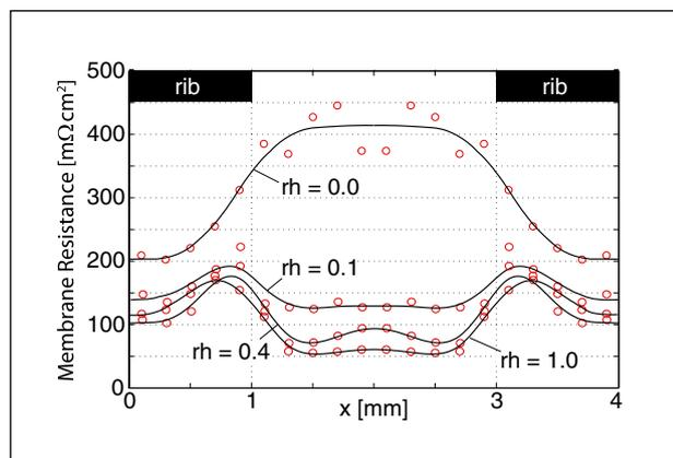
Figure 2: **Sub-mm resolved resistance measurements of membrane under channel and rib at different relative humidity (rh). Current density 400 mA/cm<sup>2</sup>; T<sub>cell</sub> = 70 °C; p = 1.5 bar<sub>a</sub>.**
