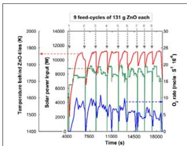
Figure 3: **Radiative power input, cavity temperature, and O<sub>2</sub> molar flow rate measured during a solar run with 9 feed cycles of 131 g ZnO each.**
