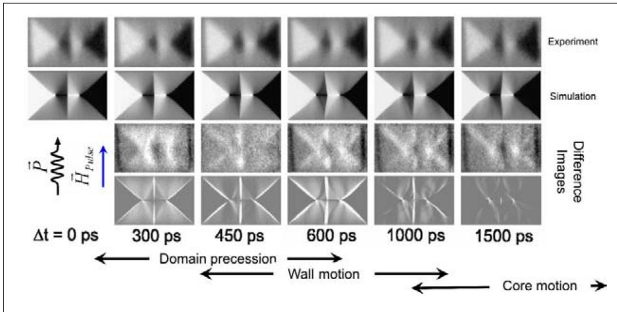
Figure 2: Magnetization  $M_y(r, \Delta t)$  of a cross-tie wall at characteristic delay times.
