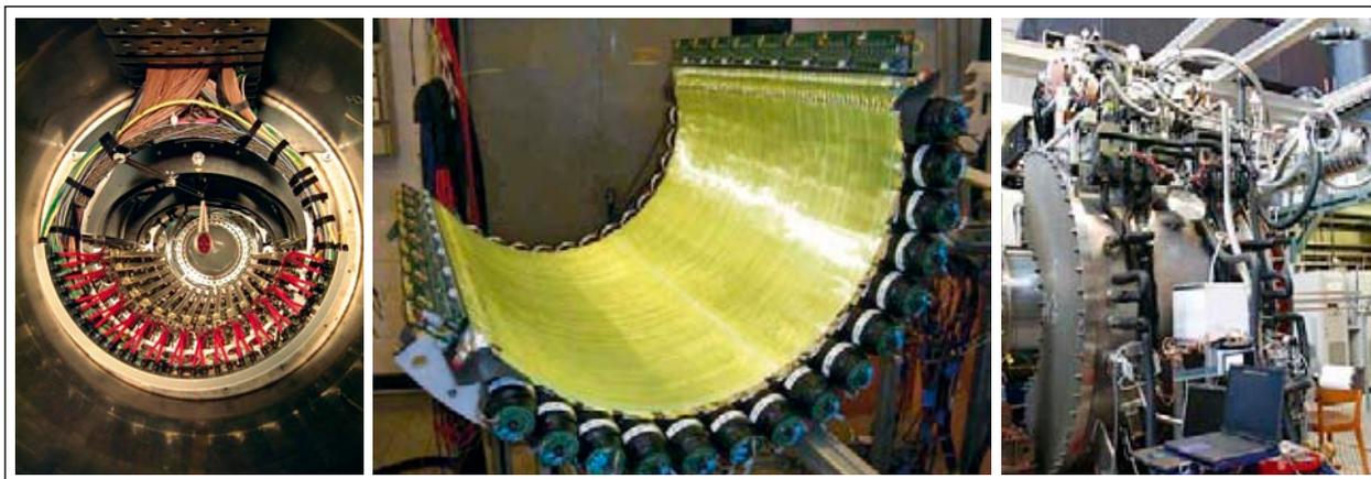
Figures 2 (Left): – COBRA central He-volume, with the Drift Chamber Assembly including the mounted target. The beam entrance window can be seen at the far end (Centre): – Timing Counter assembly with scintillating fibres and APD readout exposed (Right): – Liquid Xenon (LXe) Calorimeter installed in the  $\pi$ E5 area
