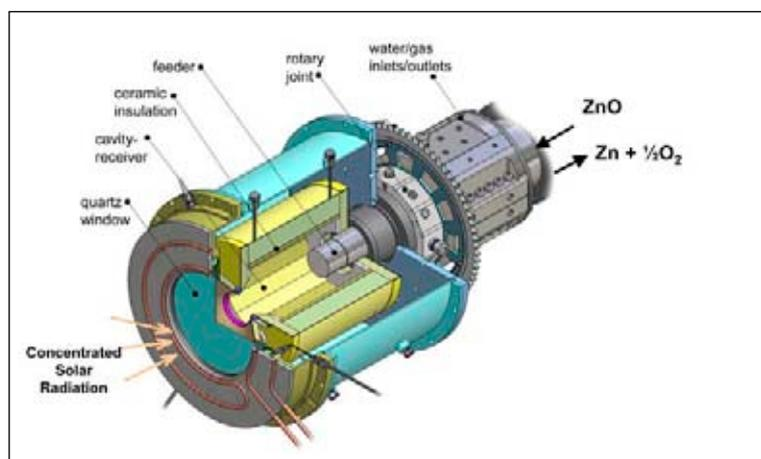
Figure 1: Schematic of the solar chemical reactor configuration.
