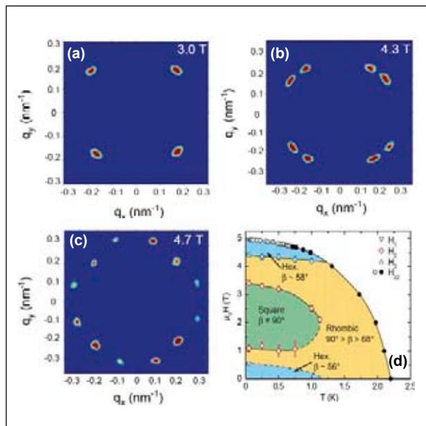
Figure 1: (a-c) Superconducting vortices as a function of field, measured using SANS-I at PSI and an 11-Tesla horizontal field dilution cryo-magnet. (d) Field-temperature phase diagram of the vortex lattice.
