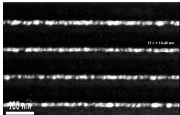
Figure 1: SEM image of 10 nm wide Au lines obtained with EUV-IL and novel lift-off processes.
