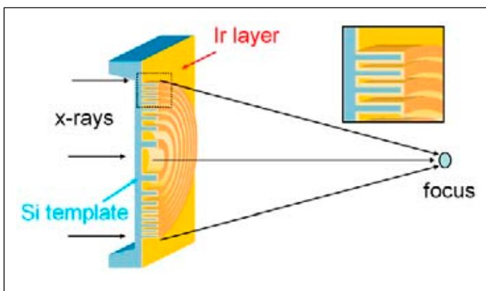
Figure 1: Zone doubling technique to obtain ultra-high resolution X-ray lenses. A silicon template is covered with a thin layer of iridium by atomic layer deposition. The cross section through the structure reveals the 20 nm wide Ir zone plate structures.
