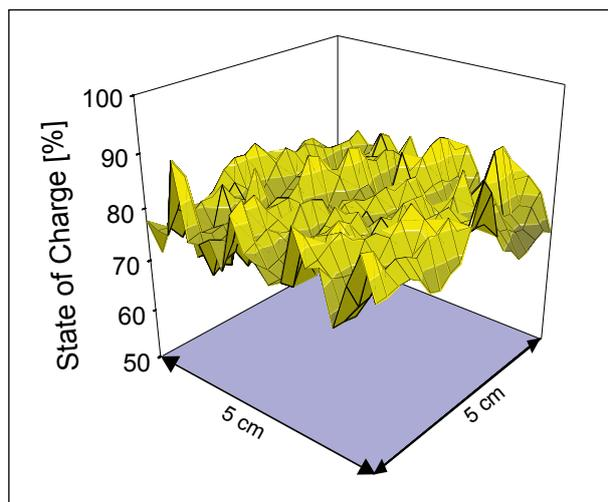
Figure 4: **Locally resolved state of charge of a carbon-based anode.**
