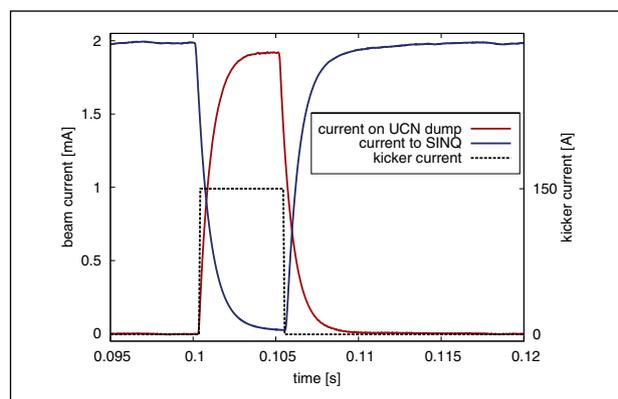
Figure 3: **Beam current measured during fast switching of the beam into the new UCN beamline. The UCN beam pulse is 5 ms long in this experiment and it will have a duration of 8 s later.**
