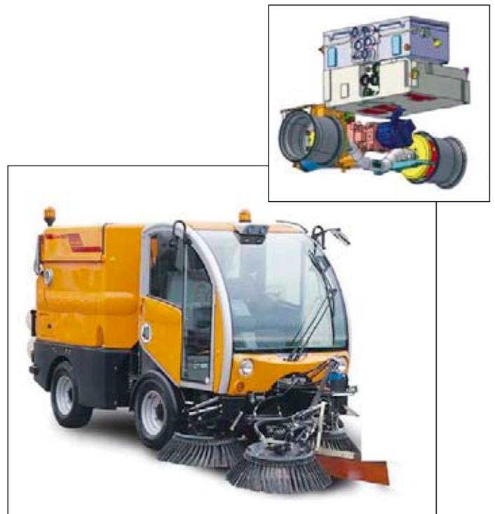
Figure 1: **Municipal vehicle to be converted and the fuel cell powertrain for enabling local emission-free operation.**
