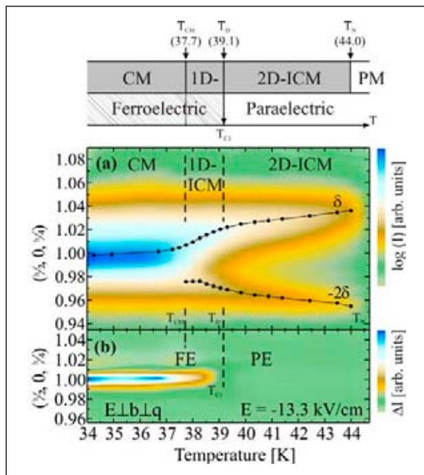
Figure 2: **top: Phase diagram of  $\text{ErMn}_2\text{O}_5$ .**
