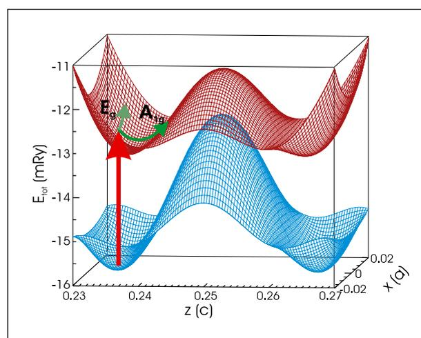
Figure 1: **Computed potential energy surface for the ground (blue) and for the excited electronic state (red) [2]. The arrows indicate the optical excitation and the  $A_{1g}$  and  $E_g$  optical phonon modes.**
