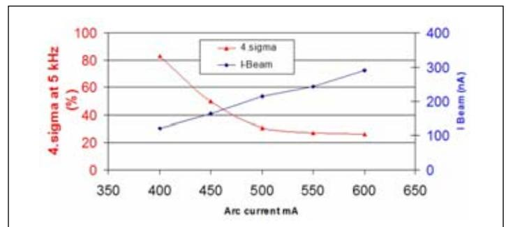
Figure 5: Extracted beam intensity and stability as a function of arc current.
