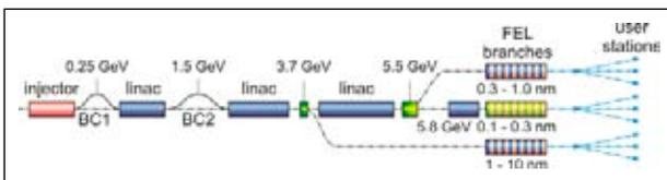
Figure 5: Schematic layout of the PSI-XFEL. A single linac feeds three FEL branches, that together cover the wavelength range from 10 nm (120 eV) to 0.1 nm (12.4 keV).
