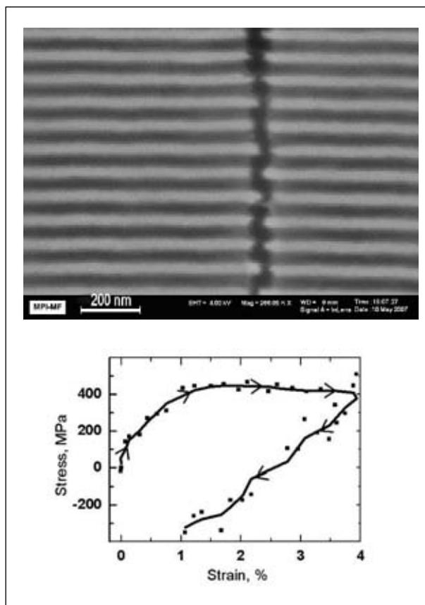
Figure 3: **a) SEM image of Au nanowires on polyimide substrate. First cracks perpendicular to the loading direction appear at a strain of 2.4%. b) Stress/strain curve of Au nanowires with 20 nm height and 50 nm width in loading direction. The arrows show the strain change direction. The yield stress averages approximately 400 MPa which is one order of magnitude higher compared to the yield stress of bulk gold and the same as in a corresponding thin film.**
