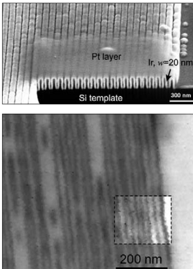
Figure 2: **Scanning X-ray microscope image of a test object consisting of lines and spaces down to 15 nm in width. Photon energy: 1 keV.**
