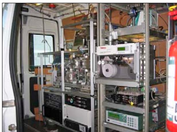
Figure 1: **Aerosol mass spectrometer and other instrumentation in the PSI mobile laboratory.**
