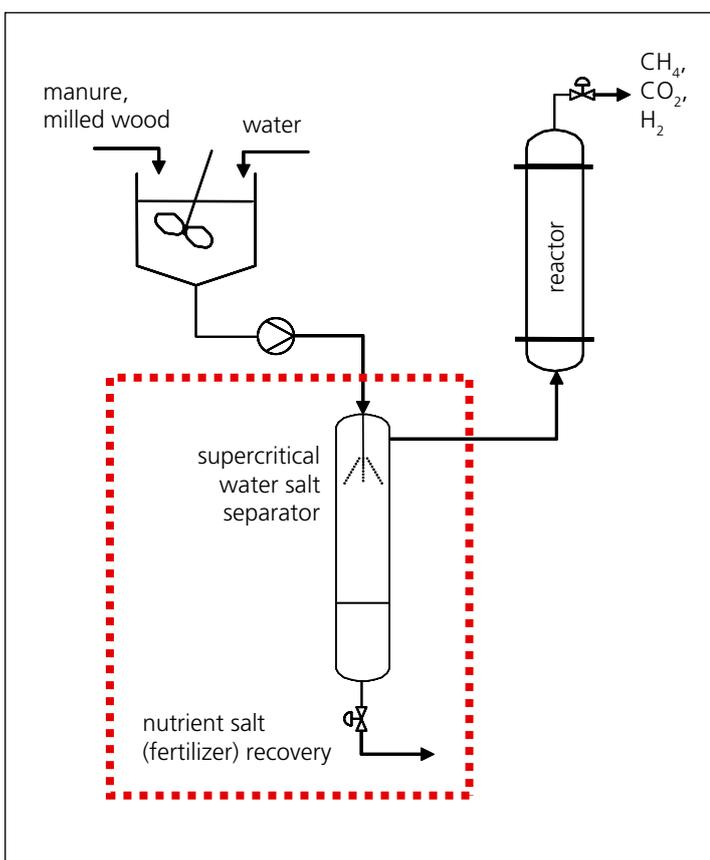
Figure 1: Schematic representation of PSI's catalytic hydrothermal gasification process (excluding heat exchangers and gas/water separation).
