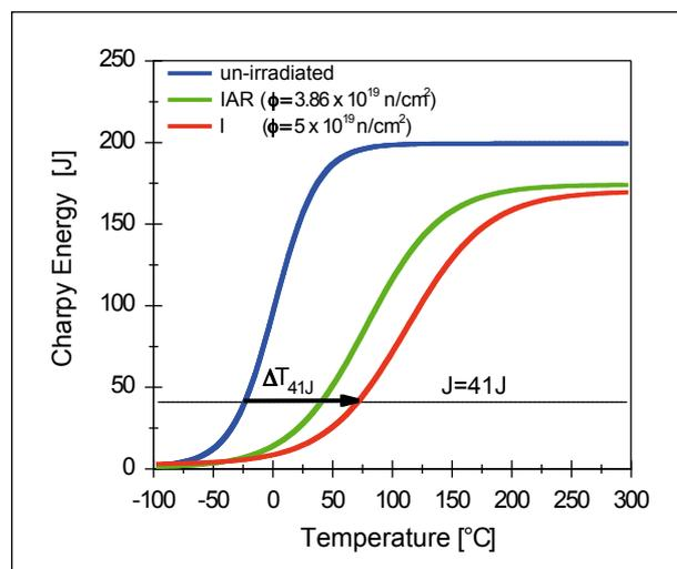
Figure 1: Charpy energy vs. temperature for un-irradiated, irradiated (I), and irradiated-annealed-re-irradiated (IAR) specimens [2].
