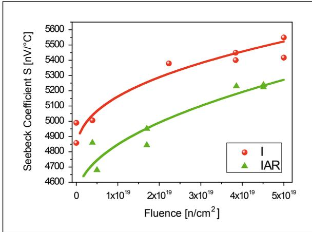
Figure 2: Measured Seebeck coefficients for irradiated (I) and irradiated, annealed and re-irradiated (IAR) specimens.
