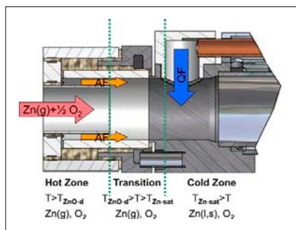
Figure 4: **Schematic of the quench apparatus illustrating the three temperature zones (AF: annular flow; QF: quench flow).**
