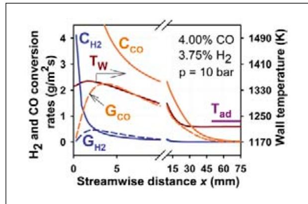
Figure 2: Computed profiles of catalytic (C) and gas phase (G) conversion rates of  $\text{H}_2$  and  $\text{CO}$ , and surface temperature ( $T_w$ ). Inlet temperature: 600 K.  $T_{ad}$ : adiabatic equilibrium temperature.
