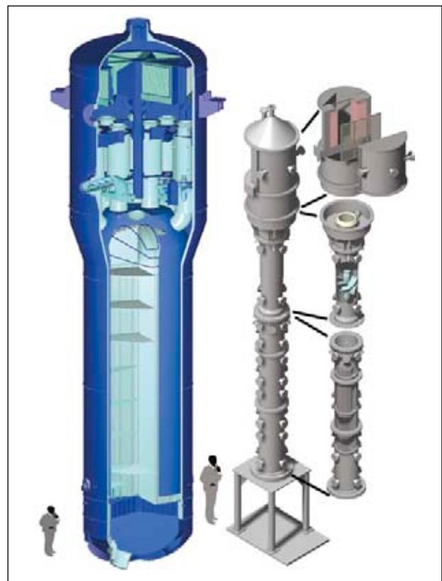
Figure 1: Schematic of the KKB SG alongside the ARTIST facility showing the relative proportions.
