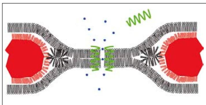
Figure 1: **Side view of a nanopore in the silicon nitride membrane (red) used as a support for stable and functional lipid bilayers, self-assembled from lipid molecules (black). Insertion of peptide and protein (green) can result in pore formation and allows diffusion of ions (blue) across the bilayers.**
