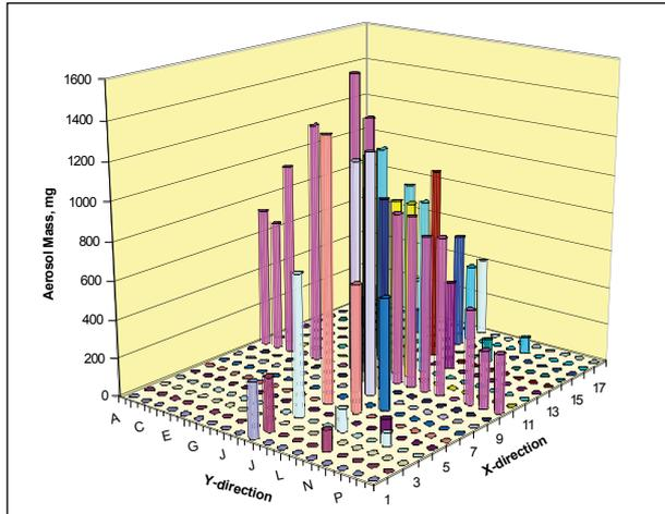
Figure 2: Aerosol deposition profile in the tube bundle.
