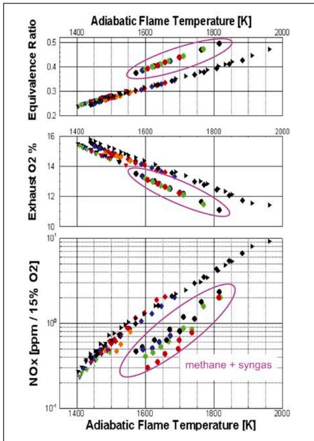
Figure 1:  $\text{NO}_x$  emission and operational range for all investigated syngas mixtures at several conditions.
