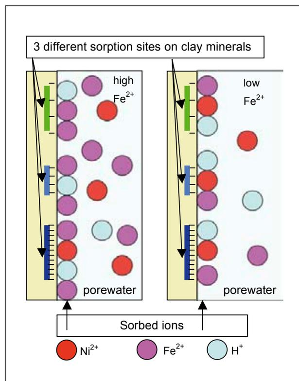
Figure 2: **Competition between  $\text{Fe}^{2+}$  and  $\text{Ni}^{2+}$  on three different sorption sites. Lower  $\text{Fe}^{2+}$  in solution results in an increased sorption of  $\text{Ni}^{2+}$  (right), and vice versa.**
