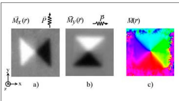
Figure 1: **Magnetization of a permalloy square. The intensity is proportional to the projection of the magnetization  $M$  onto the polarization  $P$ . The two in-plane components  $M_x(r)$  a) and  $M_y(r)$  b) are measured by rotating the sample around the surface normal ( $z$ ) in the PEEM. The vector of the in-plane magnetization is shown in c) using colour coding.**
