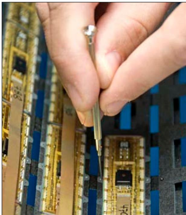
Figure 2: A pixel module is mounted onto the carbon fibre mechanics with integrated cooling by use of tiny swiss watch screws.
