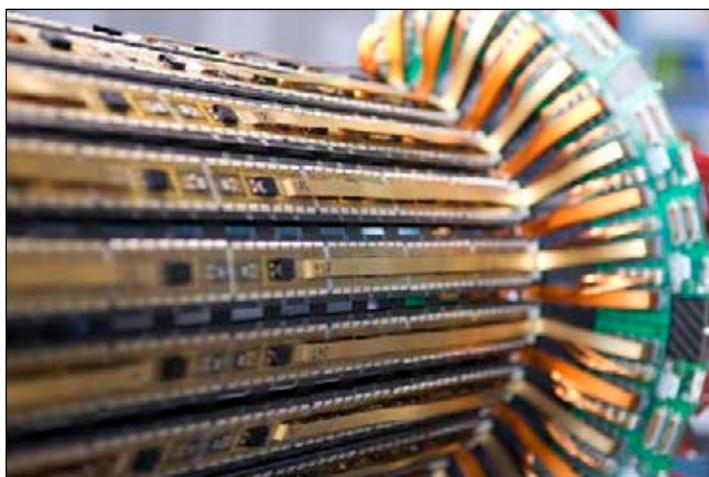
Figure 4: Details of the mounted pixel modules with the high density cabling.
