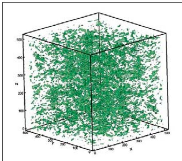
Figure 2: **Entropic Lattice Boltzmann simulation of the three-dimensional Kida-vortex flow at  $Re=20000$ . Iso-vorticity surfaces at the peak of enstrophy are presented on a  $512 \times 512 \times 512$  grid.**
