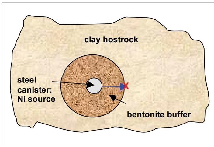
Figure 1: **Schematic cross-section through the nearfield of a high-level nuclear waste repository. The migration path is indicated by the blue arrow; X indicates the interface for which the Ni arrival time is calculated.**
