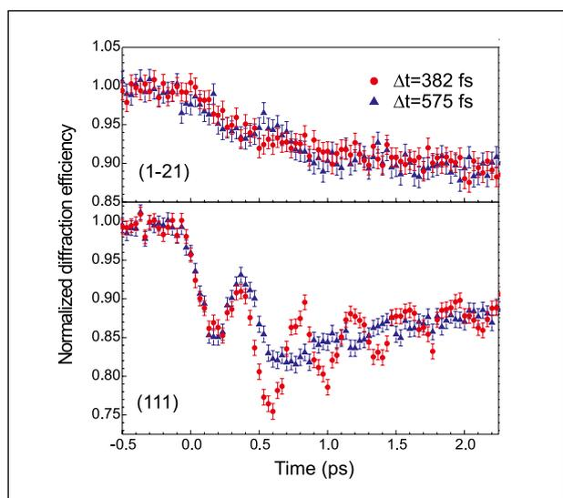
Figure 2: **Measured response of the (111) and (1-21) diffraction signals at 7.15 keV controlled by a 2-pulse excitation scheme for two delay settings of the pump pulse pair. The absorbed energy density was 1.09 mJ/cm<sup>2</sup> for the first and 0.77 mJ/cm<sup>2</sup> for the second pulse, respectively.**
