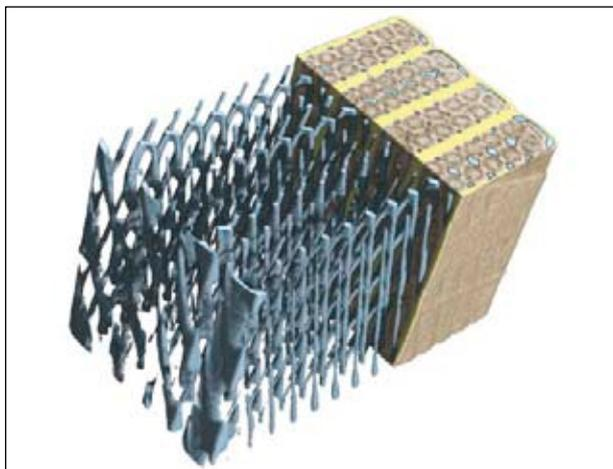
Figure 2: Tomogram of a stack of four 01B cables with partly removed structure for the visualization of the free space volume for the He cooling liquid (indicated in blue).
