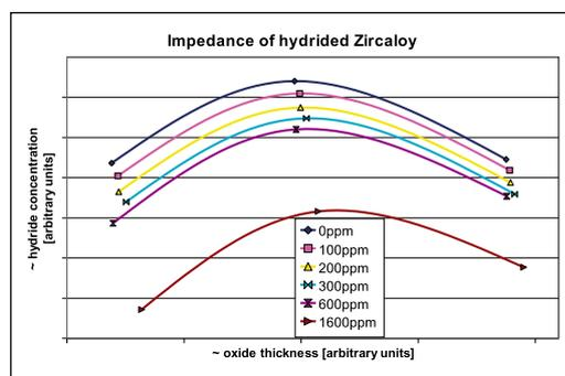
Figure 1: Non-destructive determinations of hydride concentration in fuel claddings: Impedance curves of differently hydrided zircaloy samples.
