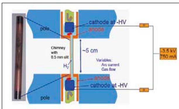
Figure 3: Schematic view of the proton source in the cyclotron center. Free electrons, created in arcs between cathodes and anodes, are trapped in the chimney and ionize gas that is flushed into the source. The protons can leave the chimney through a slit and are pulled towards the first HF electrode.
