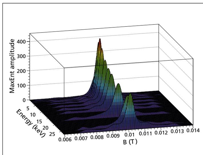
Figure 2: **Undoped ZnO, <0001> oriented, energy scan at 10 K, 10 mT applied parallel to <0001>. Maximum Entropy analysis.**
