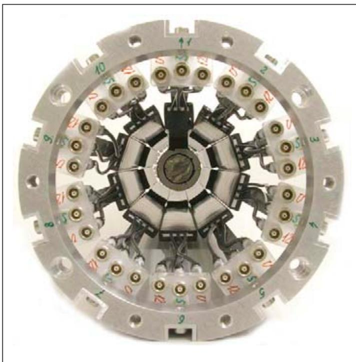
Figure 1: Prototype detector assembly for ALC  $\mu$ SR, equipped with Avalanche Microchannel Photodiodes (AMPD's) tested in magnetic fields up to 5 Tesla.
