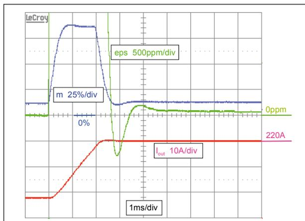
Figure 1: U-sweeper closed loop control performance.
