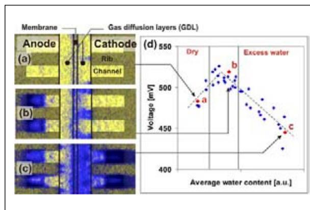
Figure 1: *In plane* Neutron Radiograms ( $2.5 \mu\text{m}$  per pixel perpendicular to membrane) of a PEFC showing the water distribution at  $1\text{A}/\text{cm}^2$  for different inlet relative humidities at the anode/cathode: (a) 60%/0% (b) 110%/40% (c) 90%/110%.
