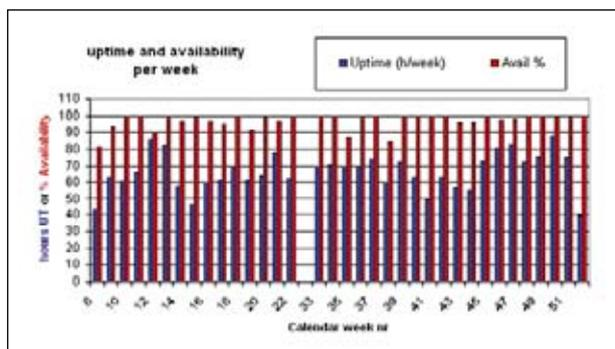
Figure 1: **Uptime and availability of cyclotron and beam lines in 2007.**
