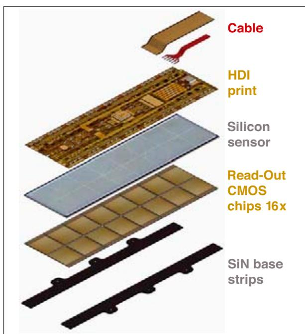
Figure 1: Exploded view of a barrel pixel module. The silicon sensor has an approximate length of 65 mm and is 16 mm wide.
