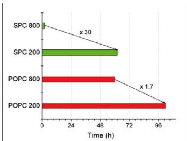
Figure 3: Time of soy phosphatidylcholine (SPC) and palmitoyl-oleoyl-PC (POPC) bilayers in 200 nm and 800 nm pores evincing a membrane resistance >1GΩ.
