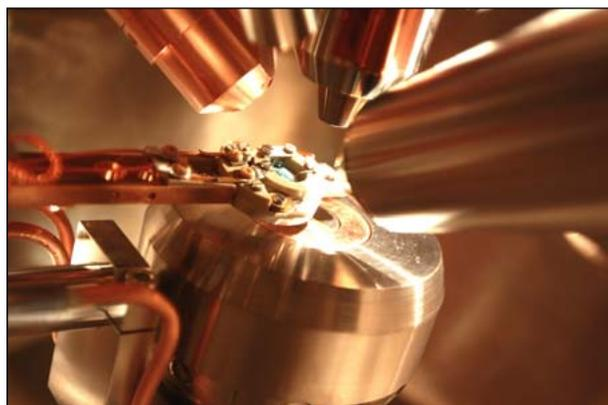
Figure 5: **View into the UHV chamber of the XPS showing the electrochemical cell with IL electrolyte.**
