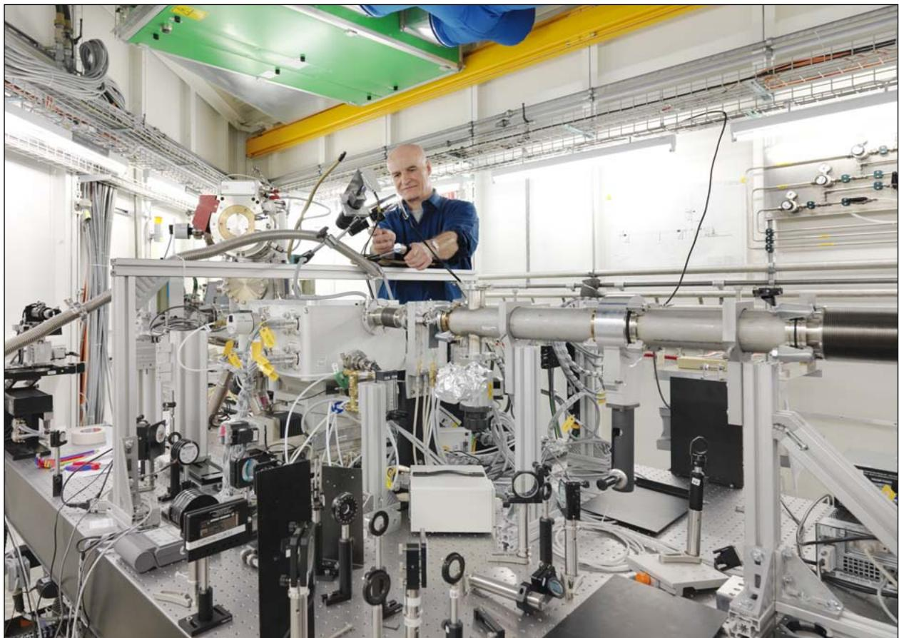
Figure 1: PSI scientist Gerhard Ingold at the FEMTO beamline at the SLS. Here, experiments with very short pulses are performed – partly as a preparation for investigations at the LCLS and SwissFEL X-ray lasers. (Photo: Scanderbeg Sauer Photography)
