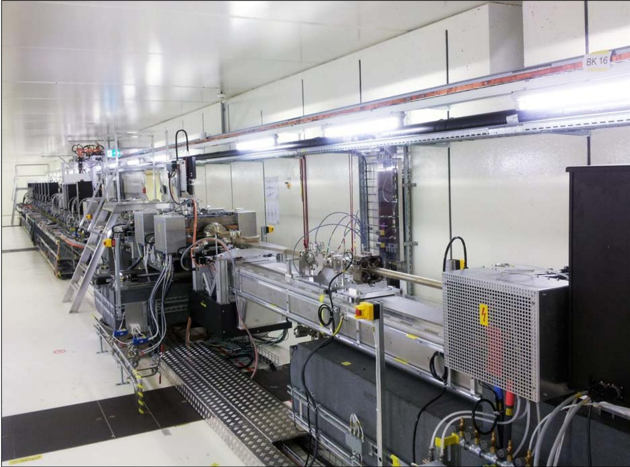
Figure 2: **Bunch compressor section installed in the tunnel of the SwissFEL Injector Test Facility.**
