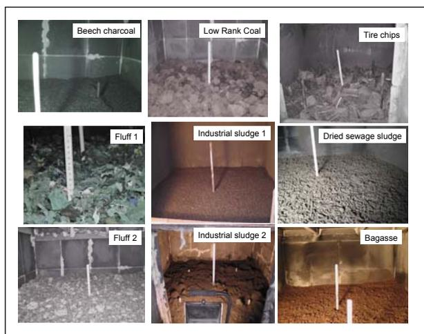
Figure 4: Packed bed of the 200 kW solar gasification reactor with different feedstocks prior to solar tests.
