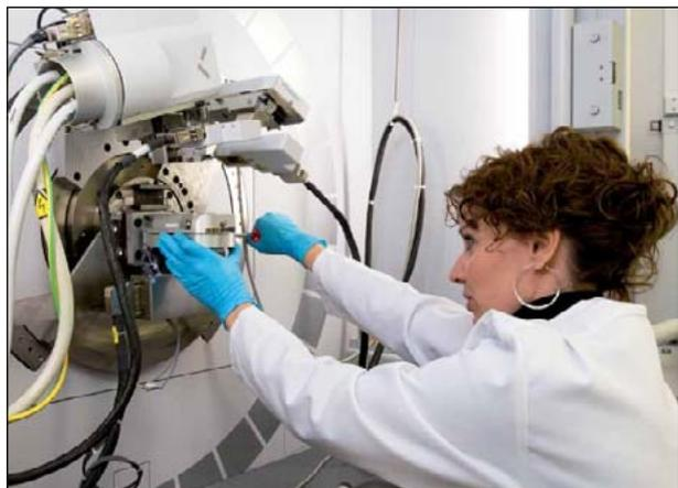
Figure 2: **Newly installed X-ray diffractometer for the structural analysis of battery materials.** (Photo: Stefan Rötheli, Appenzell)
