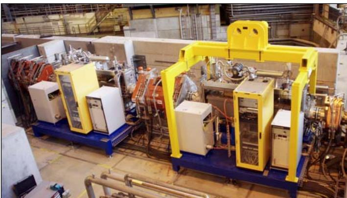
Figure 1: During the autumn of 2011, the PiE3 beam area was extended to deliver a fully polarized muon beam to the High-Field  $\mu$ SR facility. The picture shows the two spin rotators, with a refocusing element in between.
