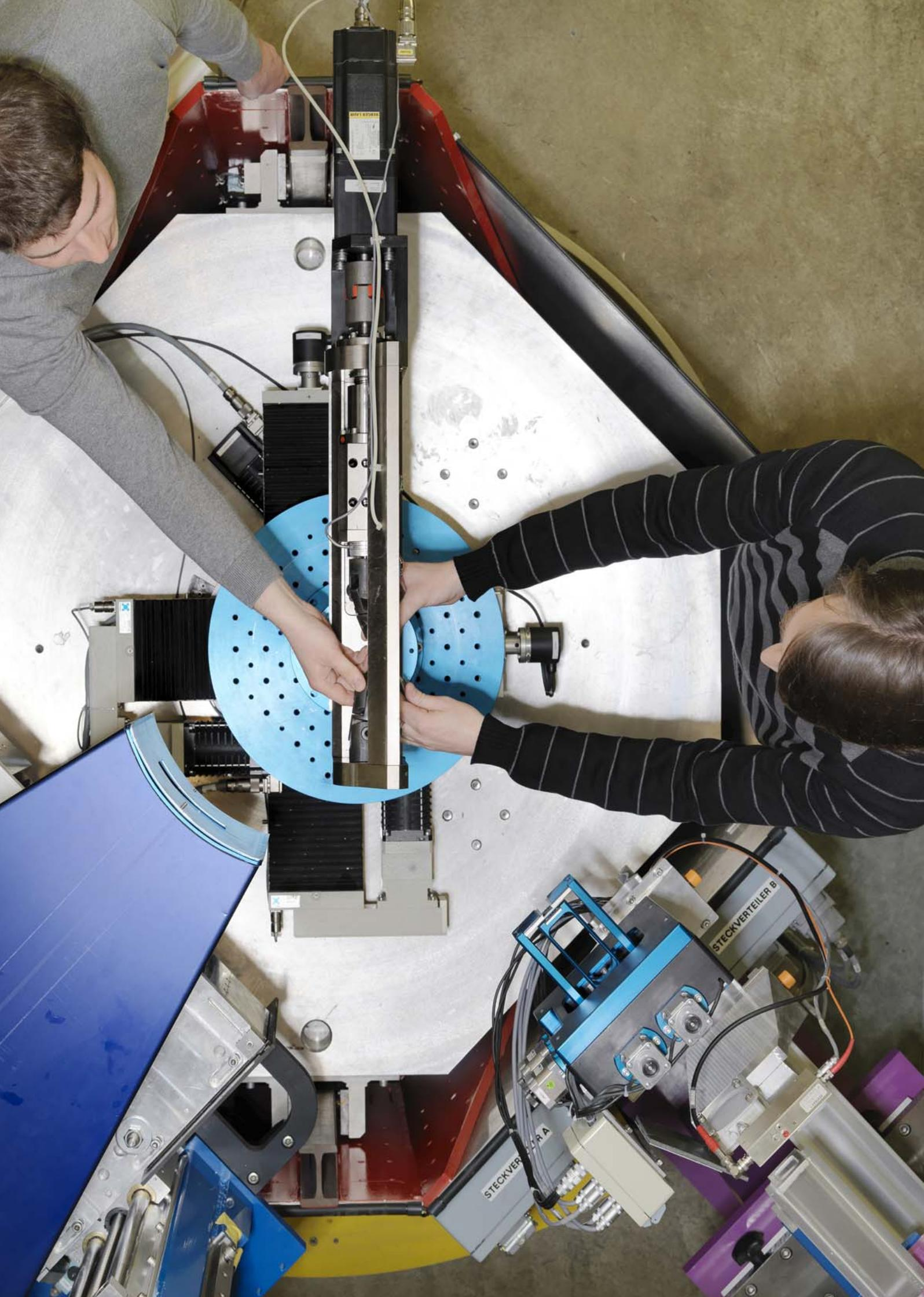
◀ **PhD students Vadim Davydov und Steven Van Petegem at the neutron instrument POLDI at SINQ. This instrument allows the non-destructive determination of residual stresses in machine components.**
