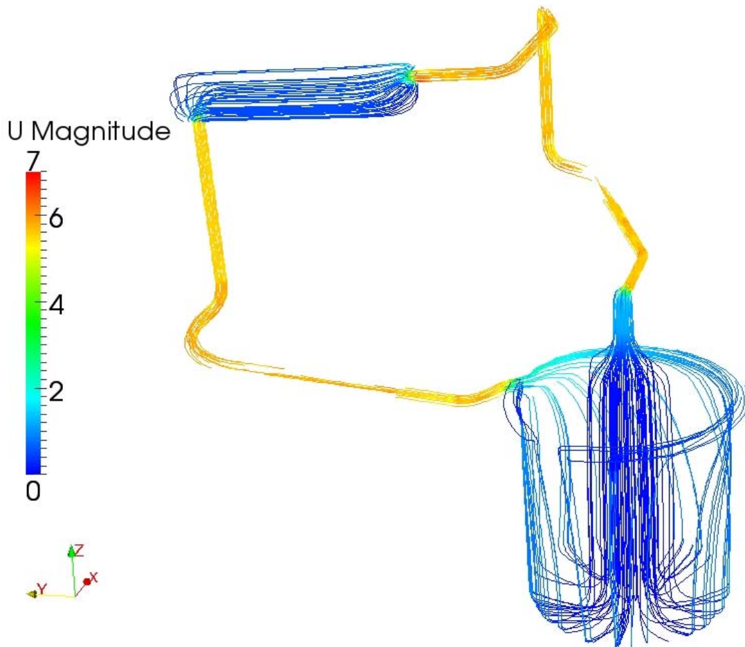
Figure 333: The streamlines along the primary circuit.
