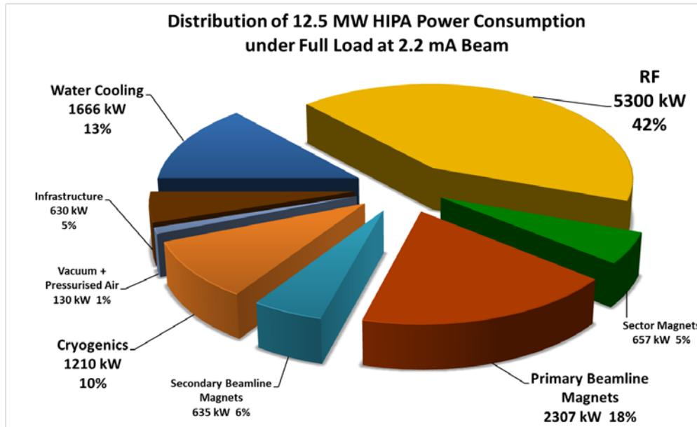
Figure 11: Distribution of HIPA power under full load at 2.2 mA beam
