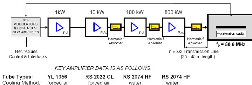
Figure 16: Tetrode Tube Amplifier Chain. Courtesy of M. Schneider.
