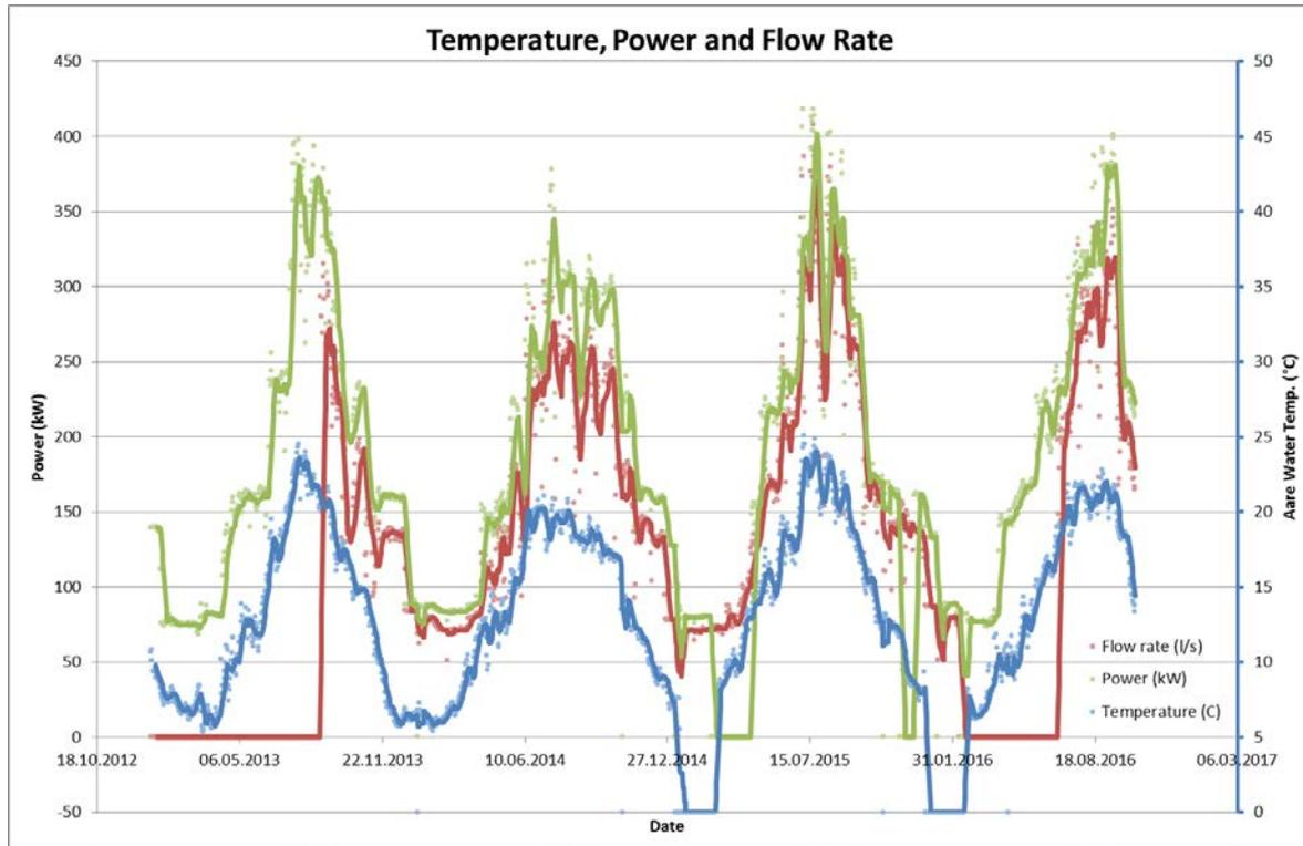
Figure 30: Water Temperature, flow rate and power consumption of OPHB pumps
