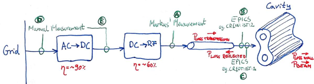
Figure 15: RF system energy flow
