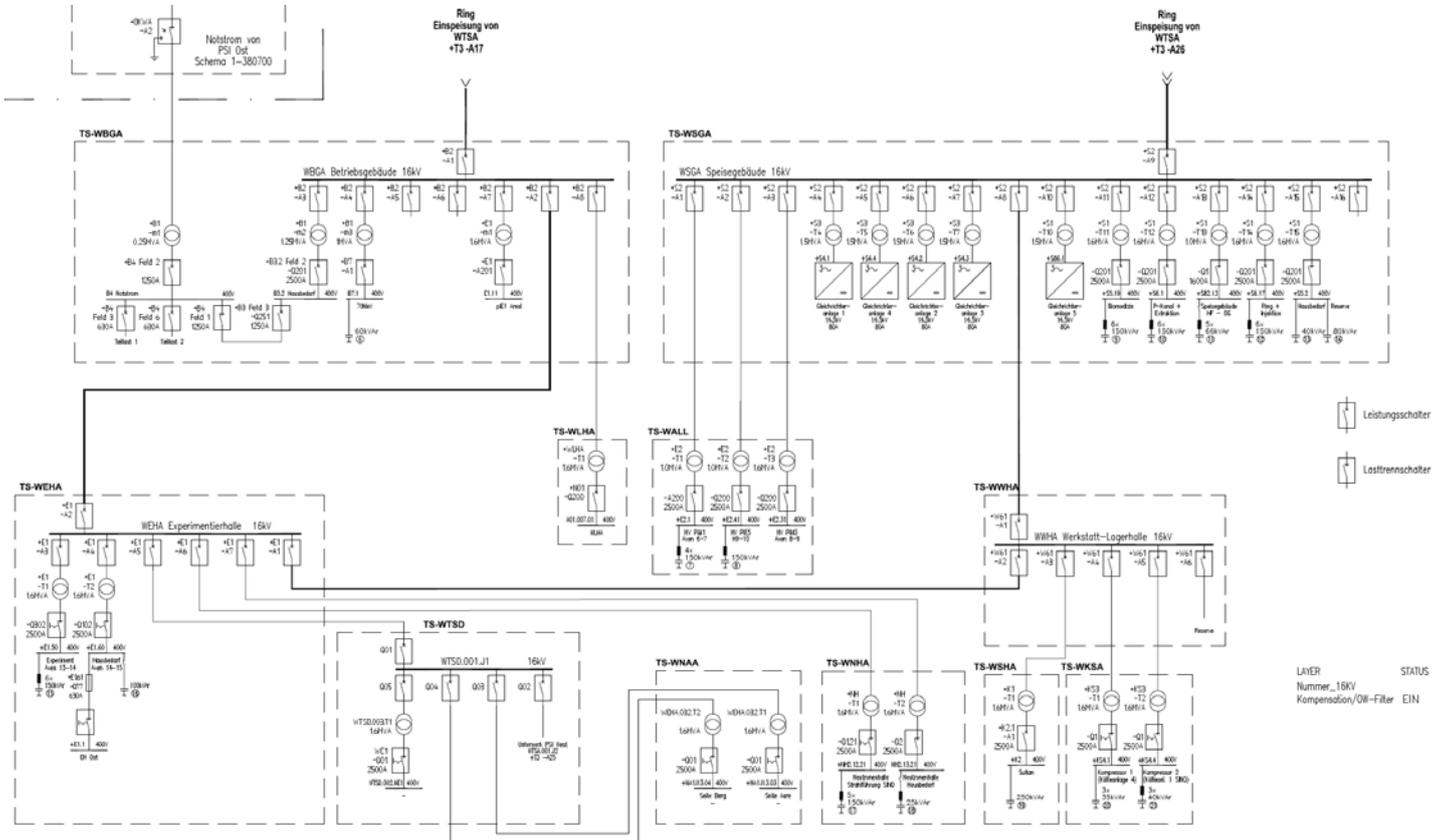
Figure 2: The layout of HIPA supply ring ‘Ring WBGA’. See source document in Appendix XXX.
