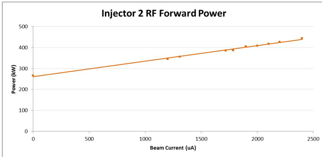
Figure 19: Injector 2 RF forward power against beam current
