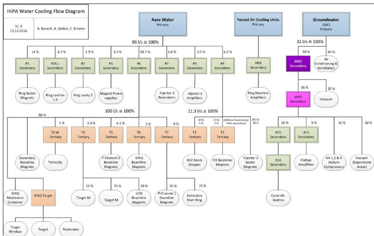
Figure 28: HIPA Water Cooling Flow diagram
