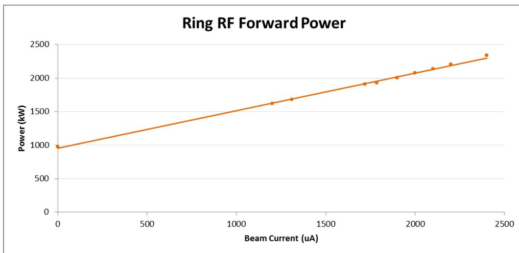
Figure 18: Ring RF forward power against beam current
