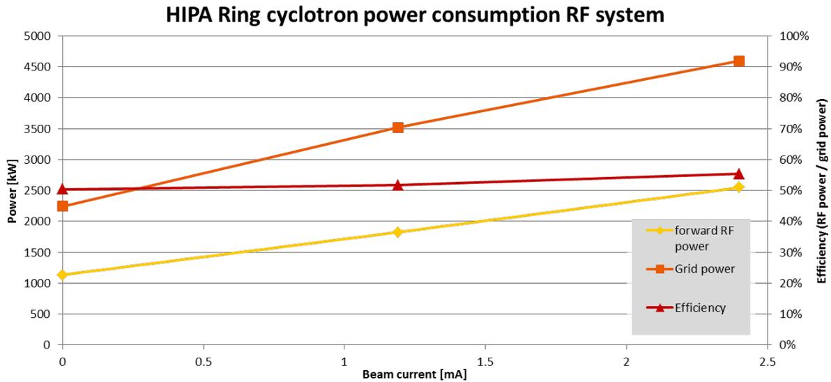
Figure 17: Ring cyclotron RF system power consumption. Data courtesy of M. Schneider
