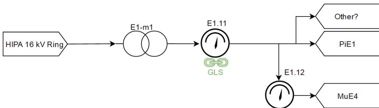
Figure 9: Simplified schematic drawing for E1-m1 transformer energy flow.
