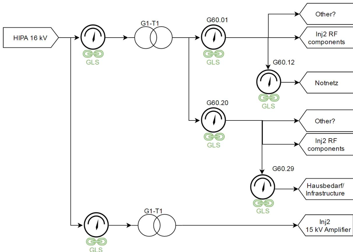
Figure 10: Simplified schematic drawing for transformers G1-T1 and G1-T2 energy flow.
