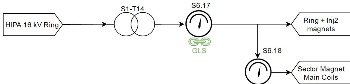
Figure 6: Simplified schematic drawing for S1-T14 transformer energy flow.
