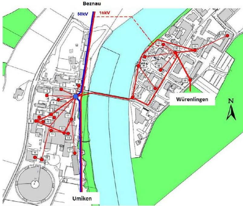
Figure 1: Layout of electrical grid at PSI. (source: PSI, 2010)
