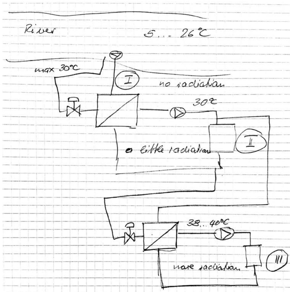
Figure 27: Schematic system overview of water cooling
