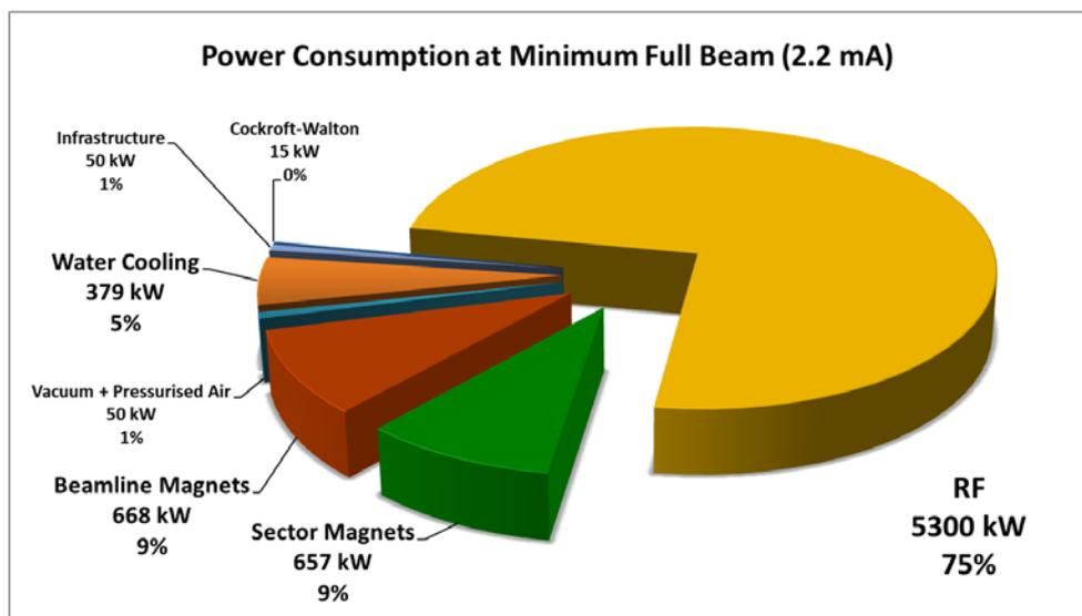
Figure 12: Distribution of power at a minimum full beam.
