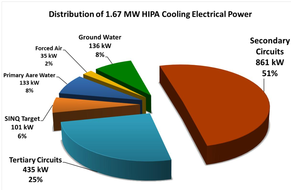
Figure 29: Distribution of HIPA Cooling Electrical Power
