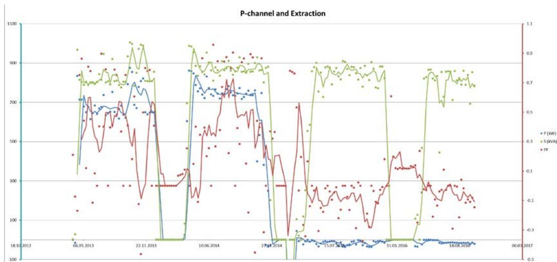
Figure 7: Plot of archived data (from January 2013 to October 2016) for real power, apparent power and Power Factor for meter S6.1.
