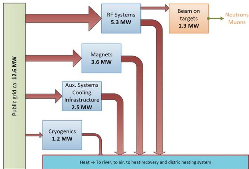
Figure 13: HIPA energy flow diagram
