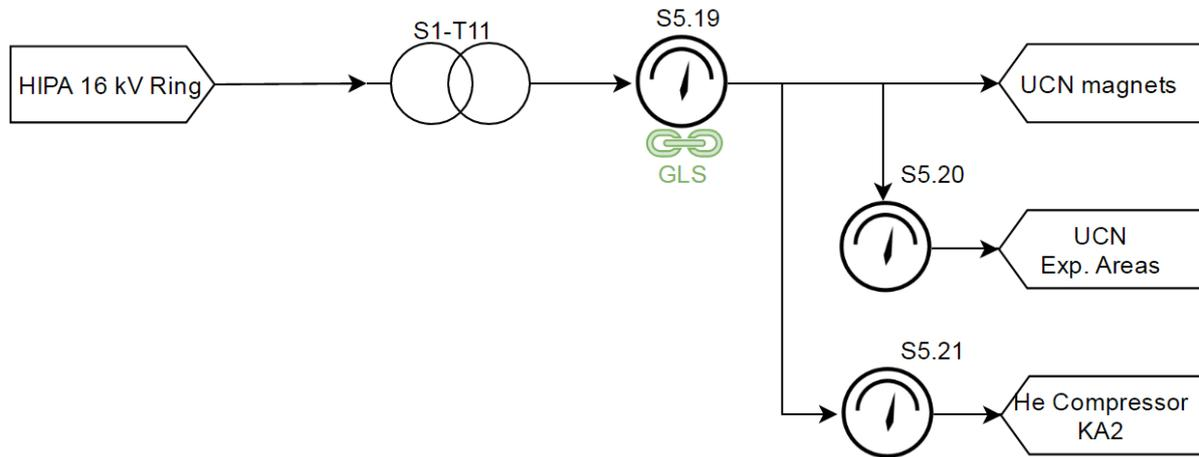
Figure 8: Simplified schematic drawing for S1-T11 transformer energy flow.
