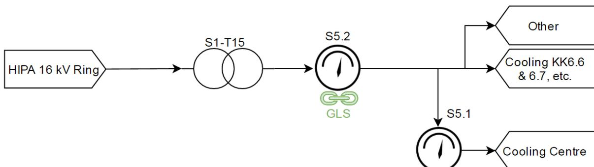
Figure 5: Simplified schematic drawing for S1-T15 transformer energy flow.
