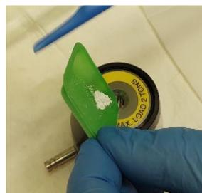
Figure 2: Filling of powder into pressing chamber.
