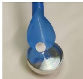
Figure 4: Pressed oxide disk.
