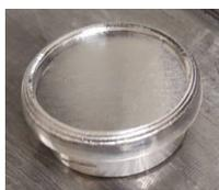
Figure 1: Aluminium capsule with irradiation target inside.
