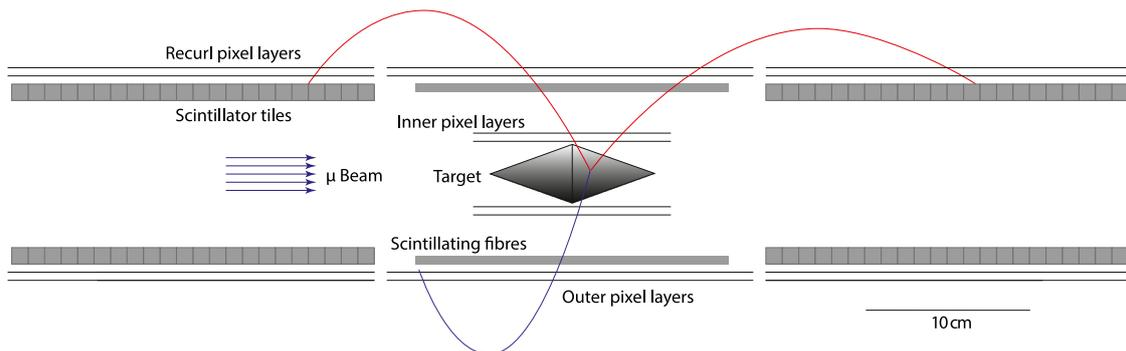
**Figure 2.** Sketch of the Mu3e detector. The central station surrounds the target and consists of four tracking layers and one layer of scintillating fibers for precision timing. The outer stations upstream and downstream have two tracking layers and one layer of scintillating tiles for complementary timing. Reprinted from [1], Copyright (2021), with permission from Elsevier.
