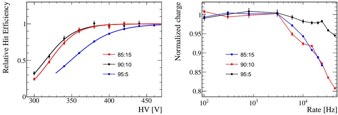
Figure 66: (Left) Efficiency of the GridPix hit reconstruction as a function of the mesh voltage, fitted with a sigmoid function and normalized to its maximum value. (Right) GridPix efficiency drop produced by the charge buildup in the mesh at high ionization rates. Efficiency is normalized to the average of the first three points. Three different Helium:Isobutane gas mixtures are considered.
