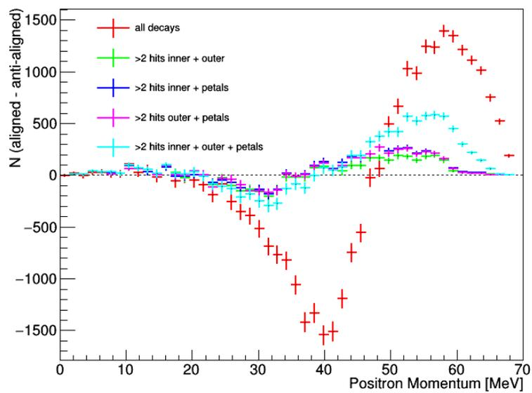
Figure 38: The sensitivity to an AMM measurement for different tracker configurations. The inner and outer layers refer to the original design and the petals are the additional layers.
