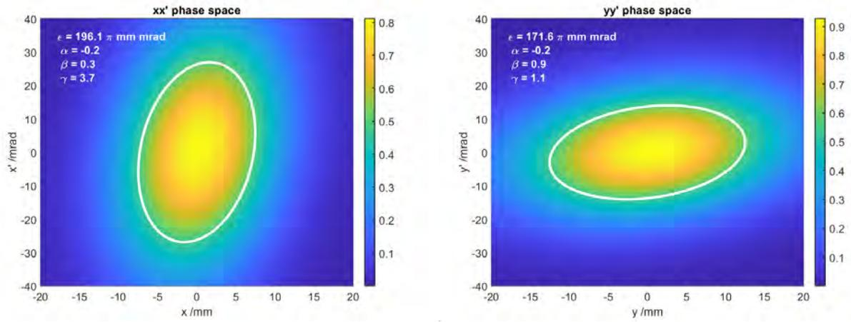
Figure 26: The Monte Carlo-generated  $x$  and  $y$ -phase space of  $\pi E1$  was used as input with the  $5 \times 10^6$  events for a simulation of transmission through the collimation channel.
