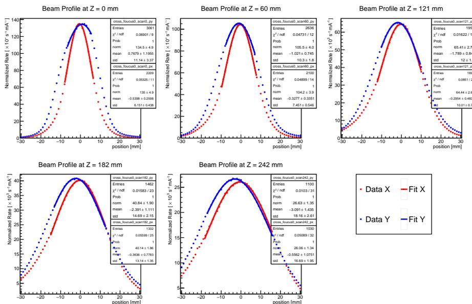
Figure 69: Fitted transverse beam profiles for the case of entrance ( $z = 0$ ) focus. The trigger rate is normalized to the proton current.
