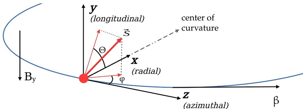
Figure 2: The local reference coordinate system used to derive the motion of the spin in the EM fields of the experiment. The vector  $z$  follows the momentum of the muon and  $y$  always points along the longitudinal direction defined by the main solenoid magnetic field  $B_y$ .
