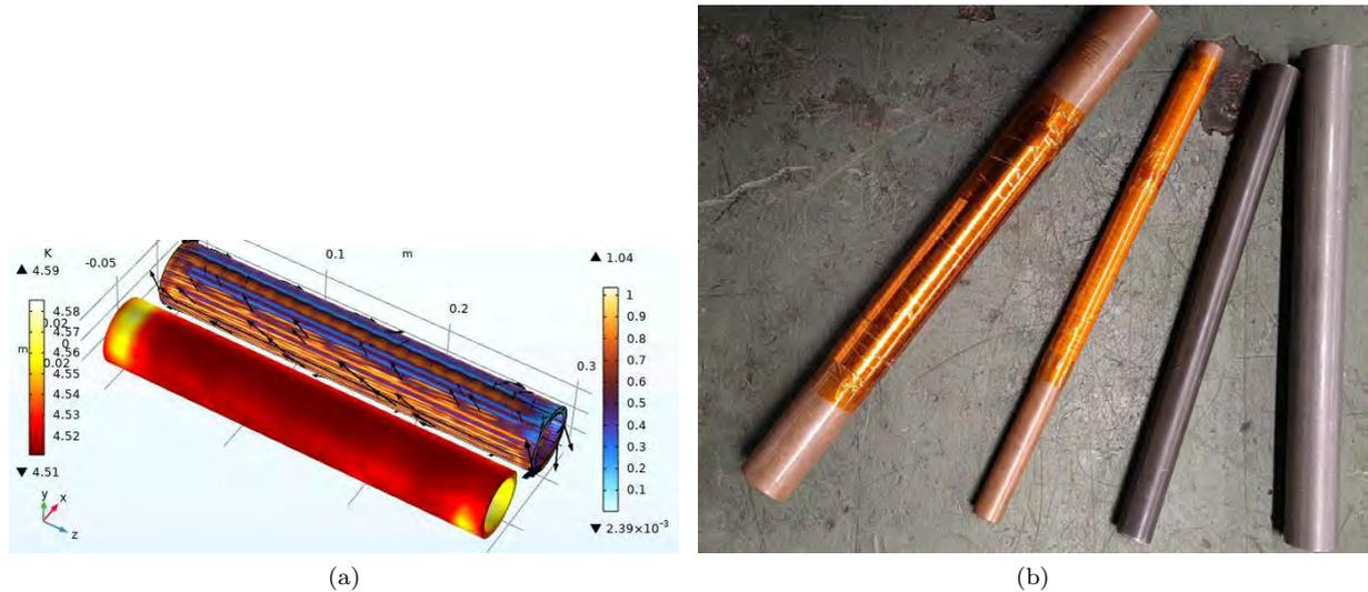
Figure 22: (a) Finite element calculation of an injection tube made of a superconducting sheet. (b) First prototype magnetic shields for the injection channel. On the left, two versions made of high temperature superconducting tape wound onto a copper tube. On the right, two standard iron tubes that might be used in the region with fields below 1 T.
