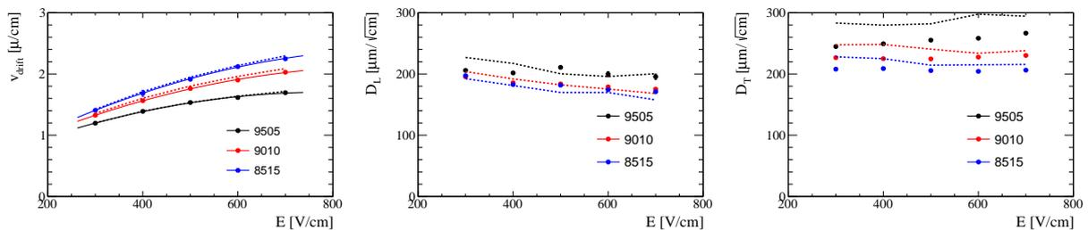
Figure 67: Electron drift velocity (left), longitudinal diffusion (center), and transverse diffusion (right) as a function of the drift field for three different Helium:Isobutane gas mixtures. The drift velocity is fitted with a second-order polynomial (continuous line). The results of GARFIELD simulations are shown with dashed lines.
