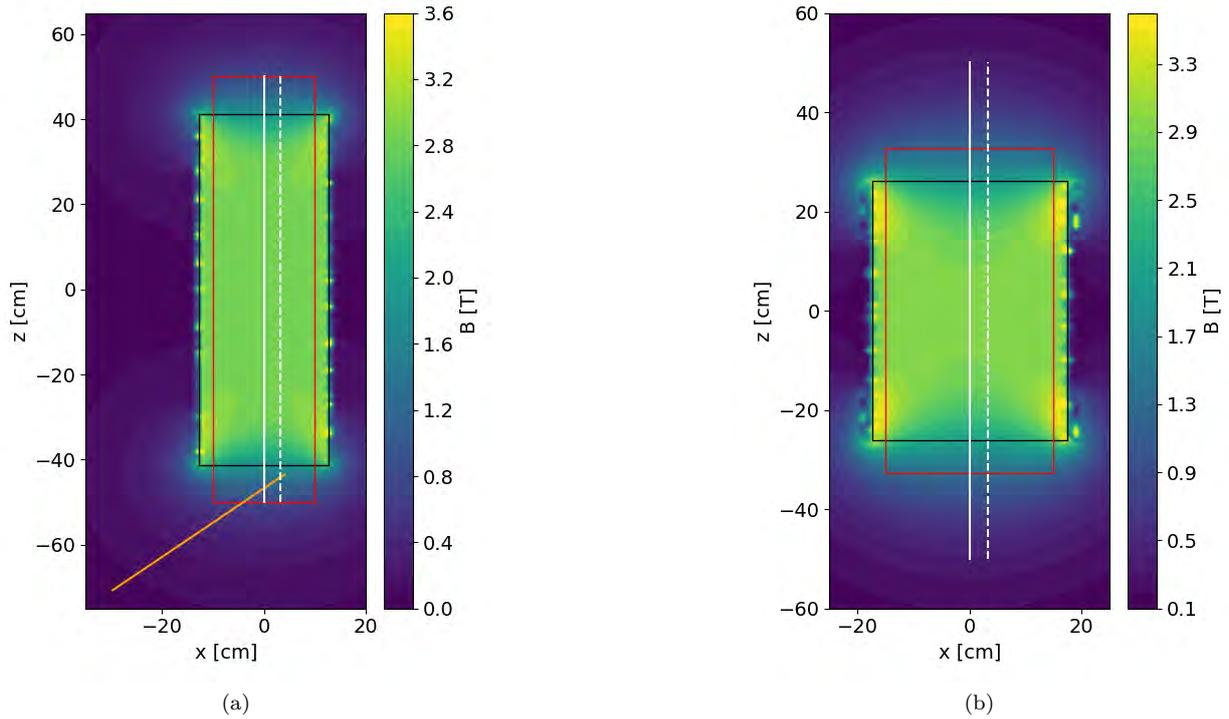
Figure 18: Contour plots of the magnetic field component  $B_z$  of PSC (a) and Ben (b) solenoid magnets. The bores are indicated as red rectangles. The magnetic field along the solid and dashed white lines is shown in Fig. 19a. The field along the orange line, indicating the position of the injection tube, is shown in Fig. 19b.
