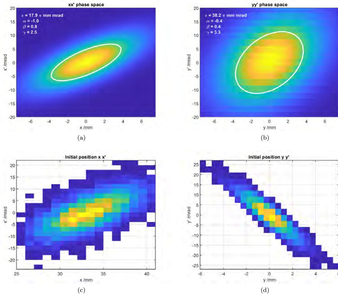
Figure 27: (a-b) Monte Carlo-simulated  $x$ - and  $y$ -phase space after transmission through a collimation tube with  $d_{inj} = 15$  mm with a total transmission of 3%. (c-d) Fraction of the phase space shown in (a-b) that is stored in the central plane 240 ns after creation. Only 1.7% of the muons that reach the exit of the collimation channel can be stored.
