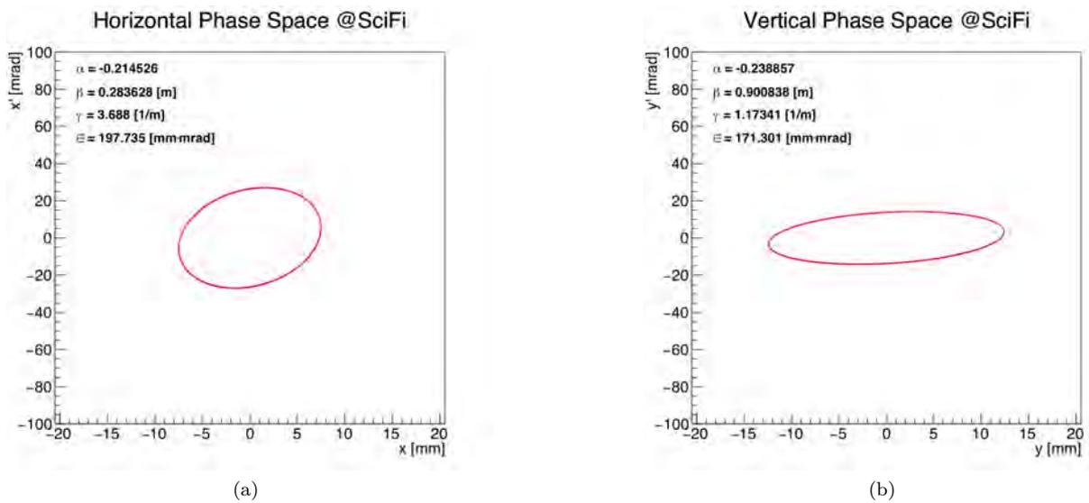
Figure 14: Measured horizontal (a) and vertical (b) phase space Twiss parameters for 28 MeV/c muons for  $\pi E1\_2$
