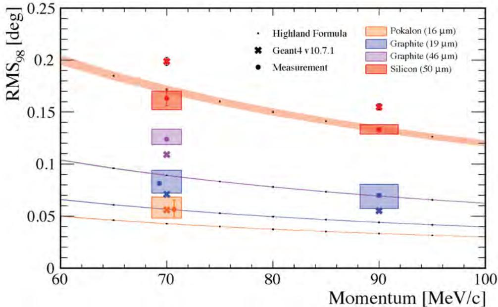
Figure 64: Experimental results are shown by the RMS of the central 98% of the sample distributions extracted by deconvolution. Statistical uncertainty is shown by the error bars, and the total error by the shaded rectangles. The  $\text{RMS}_{98}$  predicted by the Highland Formula and the GEANT4 Urbán model are also plotted, where the uncertainties on these points reflect the uncertainty in the determination of the sample thicknesses.
