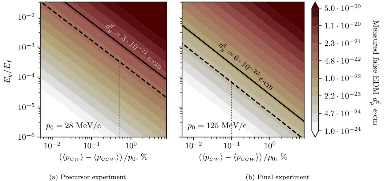
Figure 4: Limit on the difference of the average momentum between CW and CCW injection for the precursor and final experiments. The dashed lines show the level of control on the average momentum that is targeted, 0.5% and 0.1%, respectively.
