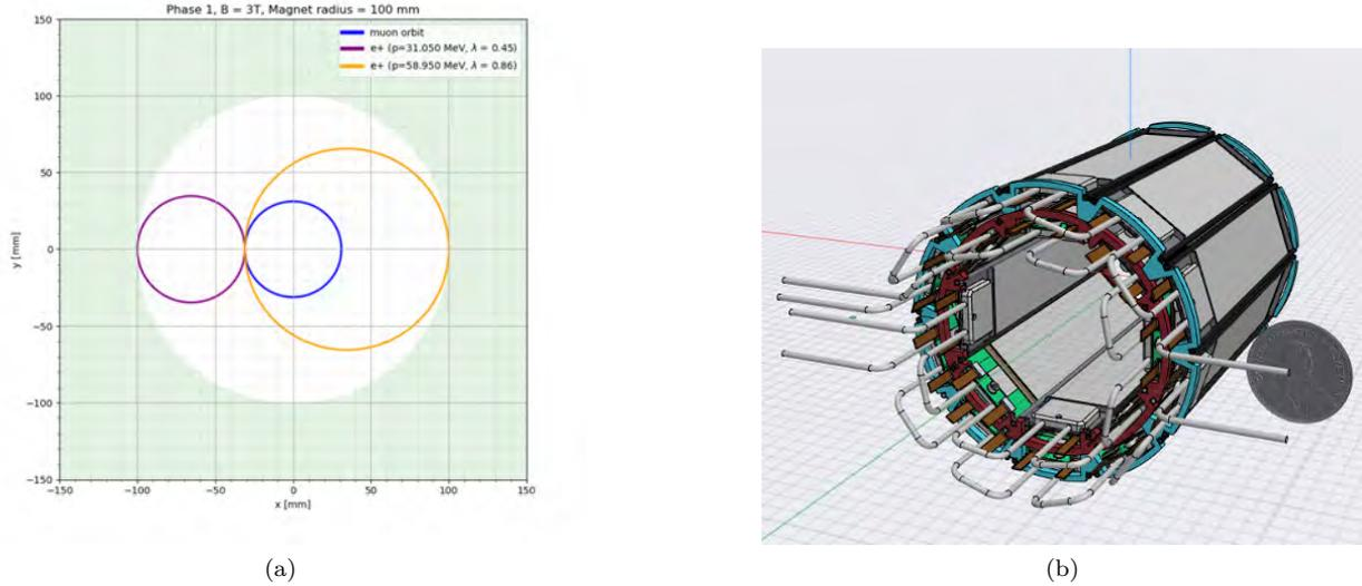
Figure 32: (a) Outward and inward positron decays that are contained with a radius of 100 mm in a 3 T magnetic field. A reference muon orbit is also shown. This simple model does not account for variation in the decay radius. (b) An example of 2 tracking detectors in place, surrounding the stored muons. Here they are placed at  $r = 35$  mm and  $r = 47.5$  mm. Note the size of the 5 CHF coin.
