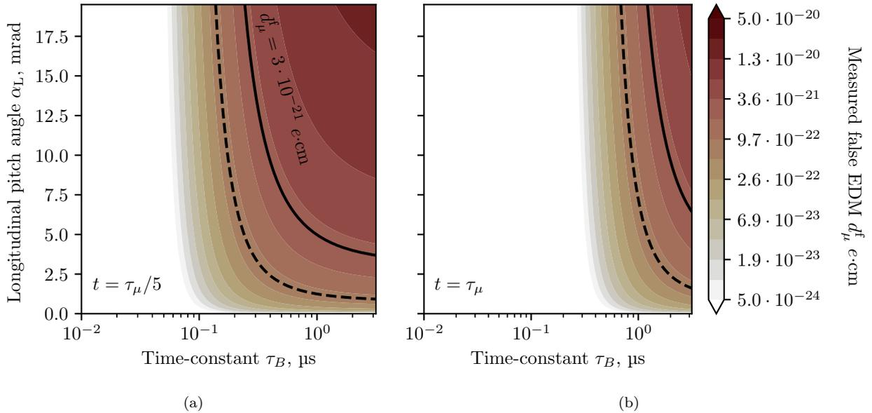
Figure 5: Measured false EDM due to an exponentially decaying residual radial magnetic field. (a) Systematic effect at time  $t = 450$  ns and (b) at time  $t = 2197$  ns, after one muon lifetime. The black line represents the target sensitivity level of  $d_\mu^f = 3.0 \times 10^{-21}$  e.cm and the dashed line is one quarter of that value. The figures show a snapshot of the limit at two different moments in time.
