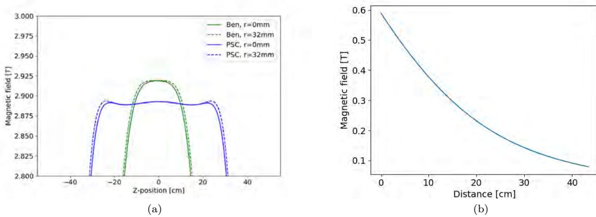
Figure 19: (a) Magnitude of the magnetic field component  $B_z$  for  $x = 0$  (solid) and  $x = 32$  mm (dashed) for PSC (blue) and Ben (green) solenoid. (b) Magnitude,  $|B|$ , of the magnetic field along the injection tube without magnetic shield.
