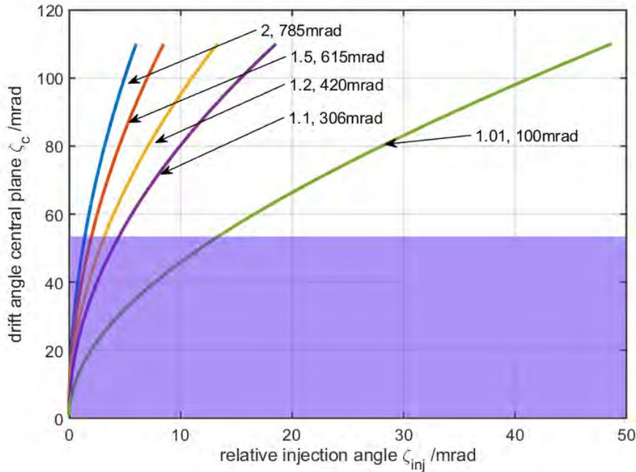
Figure 23: Injection angle offset  $\Delta\zeta_{inj}$  versus drift angle  $\zeta_c$  in the center of the magnet. Each data pair indicates the ratio  $B_c/B_{inj}$ , and the nominal injection angle  $\zeta_{inj}$ , which results in  $\zeta_c = 0$ . Note that a nominal injection angle  $\zeta_{inj} = 0$  is a lateral injection.
