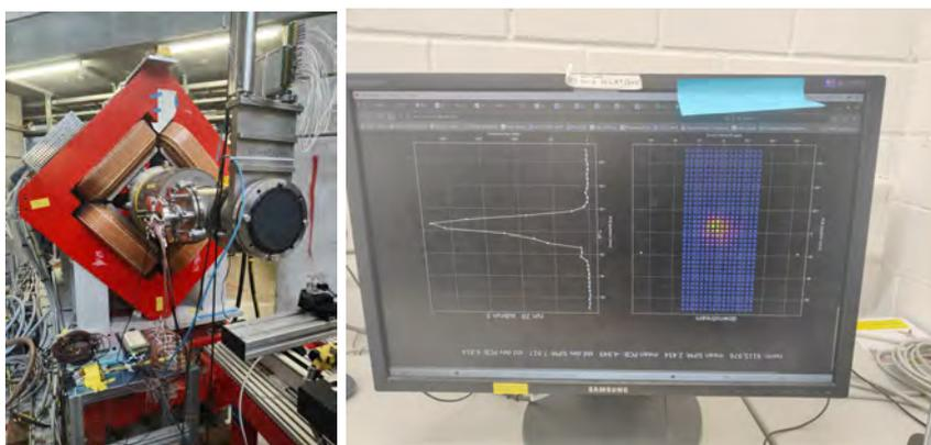
Figure 71: (Left) SiMon detector at the end of the beamline. (Right) A typical beam profile measured during the beam test.
