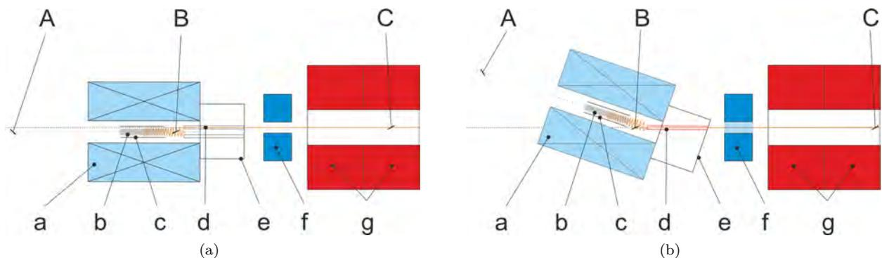
Figure 15: View of the last section of the injection beamline: side view (left) and top view (right) along the line A-B-C. From left to right: (a) SC solenoid, (b) inner high-voltage electrode, (c) outer ground electrode, (d) magnetically shielded injection channel, (e) vacuum tube, (f) horizontal dipole, (g) quadrupoles QSN55 and QSN56. (Orange) nominal muon trajectory, (black dashed) beam axis, (dark gray dotted) SC solenoid axis.
