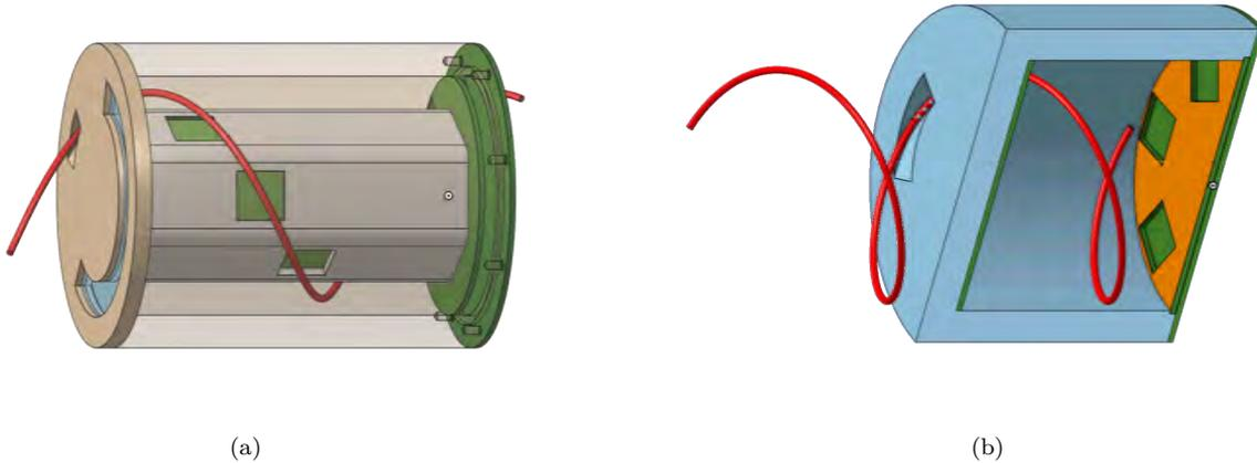
Figure 16: Sketches of possible geometries for the TPCs to measure the muon injection angle (a) and momentum (b, section view). The green squares in the electrodes correspond to the position of the GridPix sensors. The red helix represents a hypothetical muon trajectory.
