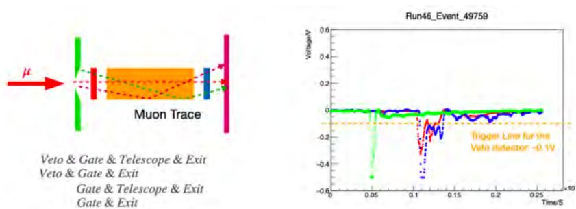
Figure 74: (Left) Classification of event types. (Right) A typical event recorded during the test beam. In this event, the muon hit the Veto (green), the Gate (red) and the Exit (blue) detectors.
