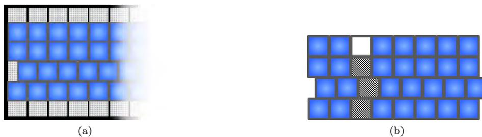
Figure 49: Illustration of a column-wise readout of fiber tracker using SiPM arrays, rather than reading out every fiber individually. Fiber tracker (blue) coupled to a SiPM array (gray/b). Emulation of the column-wise read-out by SiPM arrays, combining offline the SiPM read out (b).
