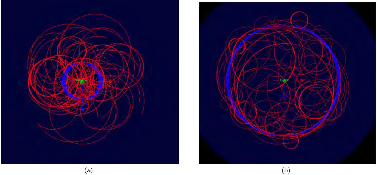
Figure 61: Plots from G4BEAMLIN simulations with muons in a 3 T uniform magnetic field, at (a) 28 MeV/ $c$  and (b) 125 MeV/ $c$  momenta, view along the solenoid axis. While in the low-momentum case most positrons tracks (red) have radii larger than the muon orbit (blue),  $r = 31$  mm, in the high-momentum case the positron track radii are smaller than the muon orbit,  $r = 139$  mm, and the positrons curl inward.
