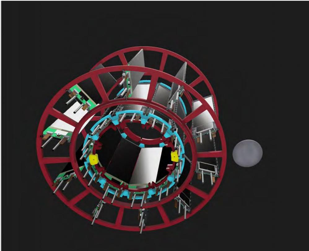
Figure 37: An extension to the original proposal, where the additional layers (here 10) are orientated in a petal formation around the muon orbit.
