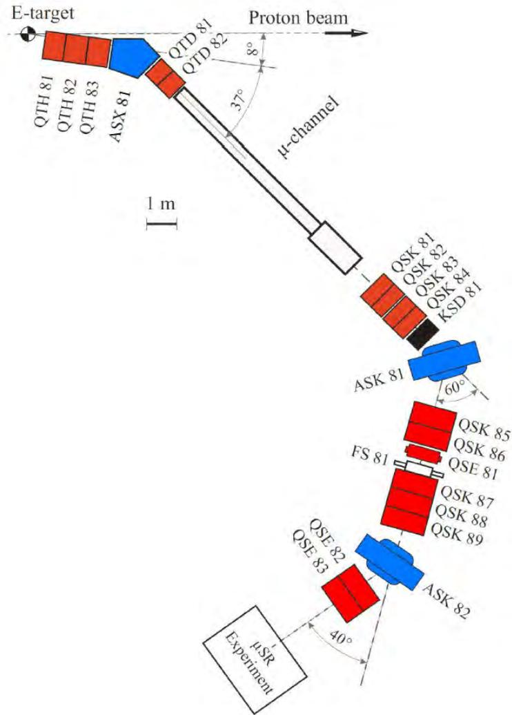
Figure 56: Layout of the  $\mu$ E1 beam line.
