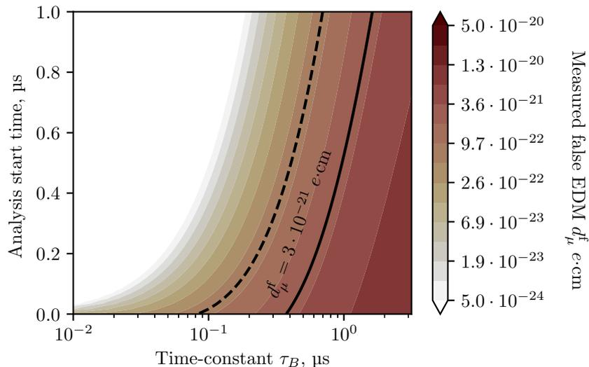
Figure 6: Phase accumulation due to exponentially decaying radial magnetic field from the analysis start time to infinity. The longitudinal pitch angle is 10 mrad.
