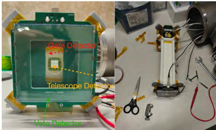
Figure 73: (Left) A muon beam view of the entrance trigger. (Right) A top view of the entrance trigger.
