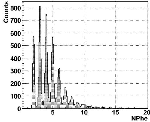
Figure 50: Typical light spectrum (threshold 0.5 phe) measured by a single 250  $\mu\text{m}$  square multiclاد fiber ( $\approx 50$  cm length) read out by a SiPM on each end (SiPMs combined in logic AND) upon the passage of a mip.
