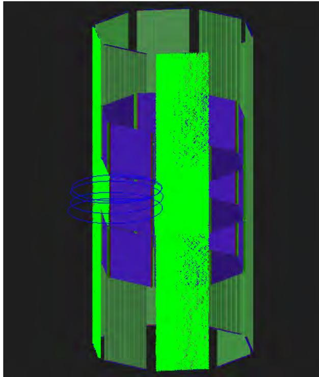
Figure 44: An example of GEANT4 simulated event. In green the optical photons reflecting inside the fiber ribbons; in blue the trajectory of the positron. Keeping the same colour scheme, the longitudinal SciFi is green while the transverse one is blue.
