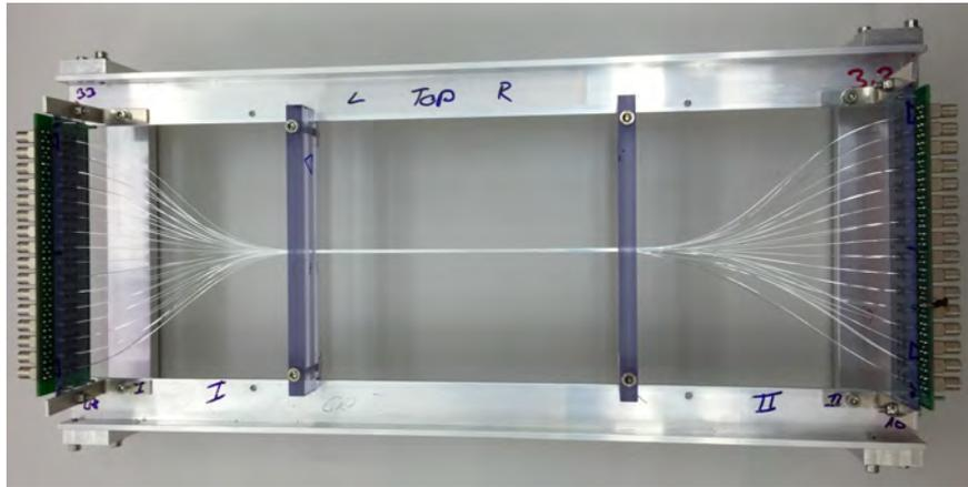
Figure 48: The Large Prototype, made of 32 squared, multicladd BCF-12 fibers of 250  $\mu\text{m}$  thickness. Each individual fiber is coated with  $\sim 100\text{nm}$  of aluminum and read out by a SiPM at each end.
