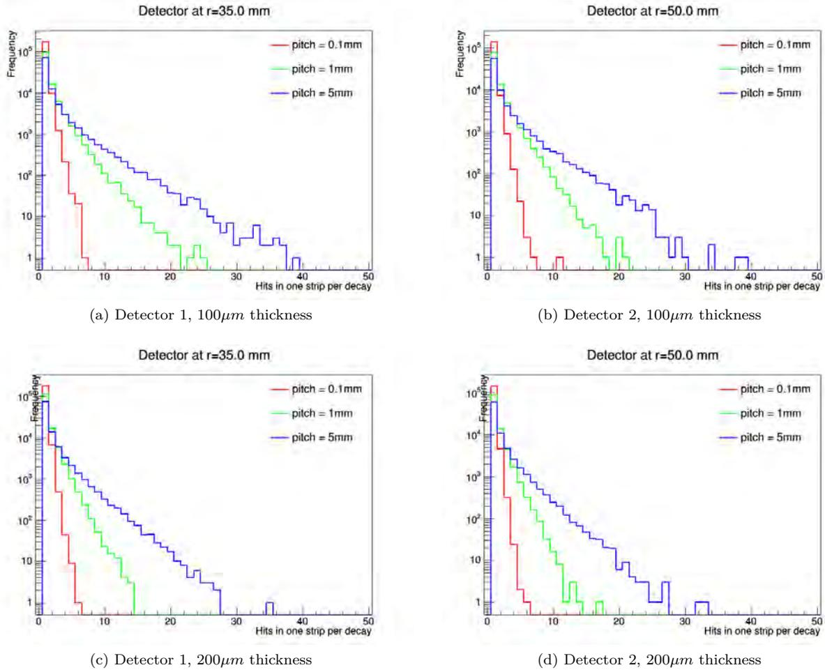
Figure 40: Hit multiplicity in a single strip for 3 different pitches. Each detector is made of Silicon with the quoted thickness.
