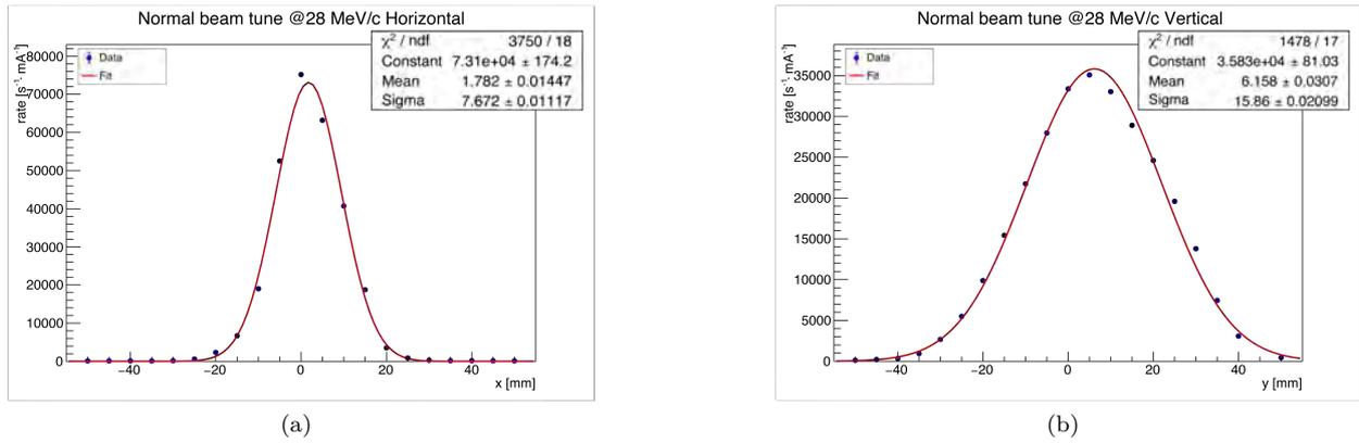
Figure 13: Measured horizontal (a) and vertical (b) muon beam distribution at 28 MeV/c for  $\pi E1\_2$
