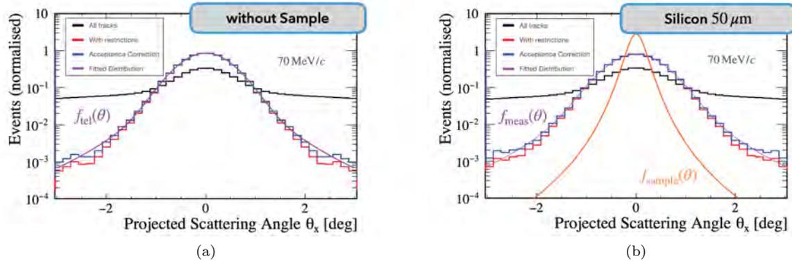
Figure 63: The angular distributions of the experimental data measured without sample (a) and with  $50\ \mu\text{m}$  Si (b) are shown, along with fitted functions. The raw distribution (black) is restricted to tracks that meet criteria on the fit and intersection at the sample plane. A correction is applied to account for the geometric acceptance of the telescope. The orange curve in (b) shows the sample distribution extracted from deconvolution of the two fitted distributions.
