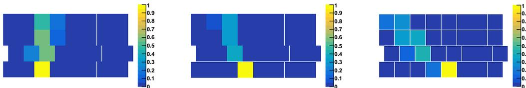
Figure 52: Particle tracks observed in the Large Prototype as a function of the inclination angle  $\phi$ . From left to right, the impinging angle is  $\phi = 0^\circ$ ,  $\phi = 22^\circ$ , and  $\phi = 60^\circ$ . The color scale indicates the number of events involving the corresponding fiber relative to the number of triggered events.
