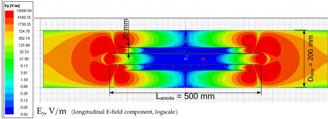
Figure 7: Longitudinal E-field component for a 500 mm long coaxial electrode structure simulated using ANSYS finite element simulations. The color scale is logarithmic and the values are in units V/m. The radial component  $E_r$  is 270 kV/m. The potential difference between the anode and cathode is 6.2 kV.
