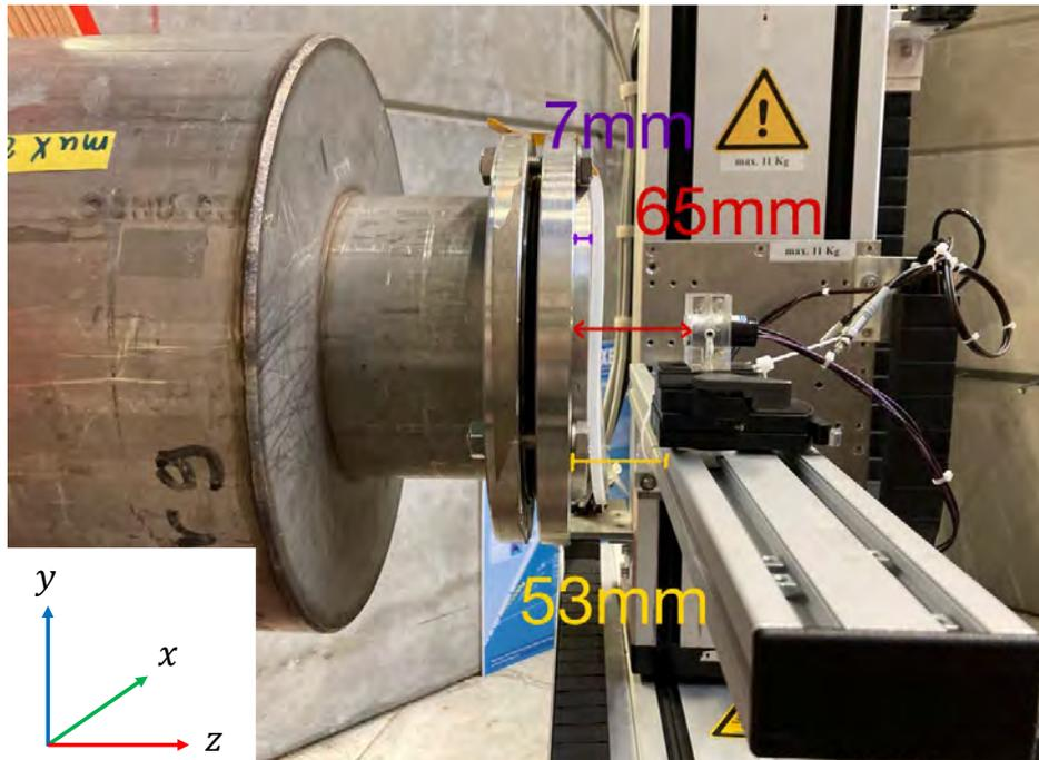
Figure 68: Setup of the beam scanner. The PMT on the plastic holder (the pill scintillator is covered at the front of the PMT and is not shown) is at the  $z = 0$  position. The muon beam direction is taken as the  $z$ -direction. The last flange will be housing for the entrance detector's vacuum tube. Part of the last quadrupole magnet in the beamline is also shown.
