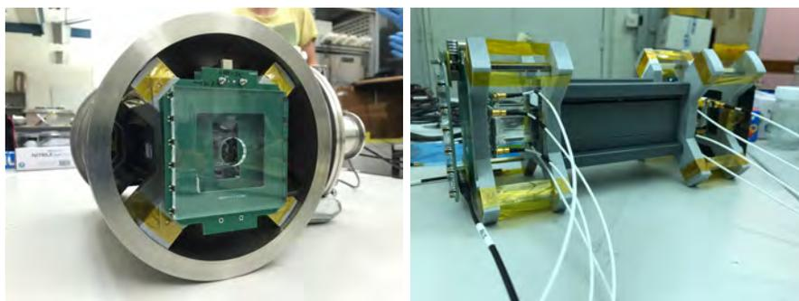
Figure 75: (Left) the entrance detector installed into the vacuum tube. (Right) A side view of the entrance trigger.
