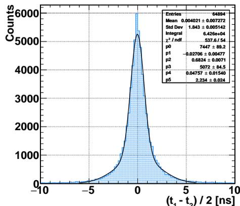
Figure 51: Timing distribution of a single fiber with a double Gaussian fit (solid line).
