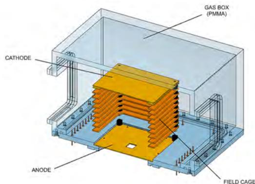
Figure 65: A schematic of the TPC prototype used for the characterization of the GridPix (section view).
