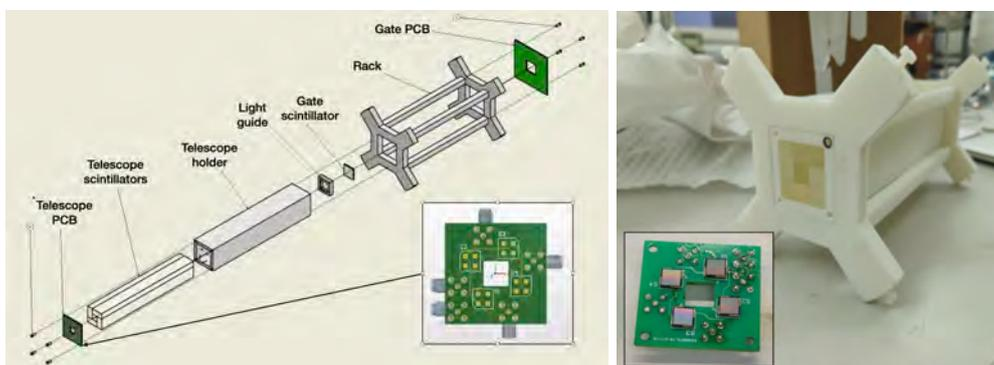
Figure 72: (Left) A 3D CAD drawing of the muon entrance detector. (Right) A prototype entrance detector developed for the test beam at PSI. Insets are SiPM read out boards for the telescope scintillators.
