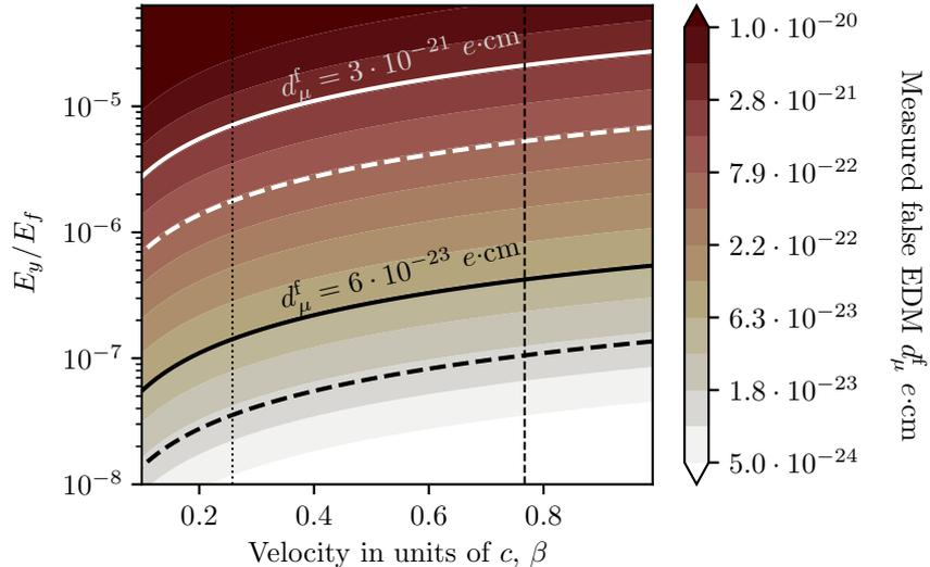
Figure 3: The measured false EDM due to non-zero average electric field in the vertical direction. The solid horizontal line shows the target sensitivity for the true EDM and the dashed horizontal line is one quarter of that value. The vertical dotted line is at  $\beta = 0.258$  as for the precursor experiment and the vertical dashed line is at  $\beta = 0.767$  as for the final experiment.
