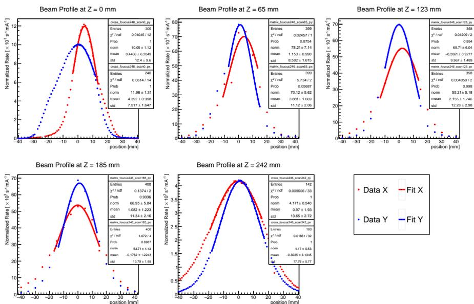
Figure 70: Fitted transverse beam profiles for the case of exit ( $z = 246 \text{ mm}$ ) focus.
