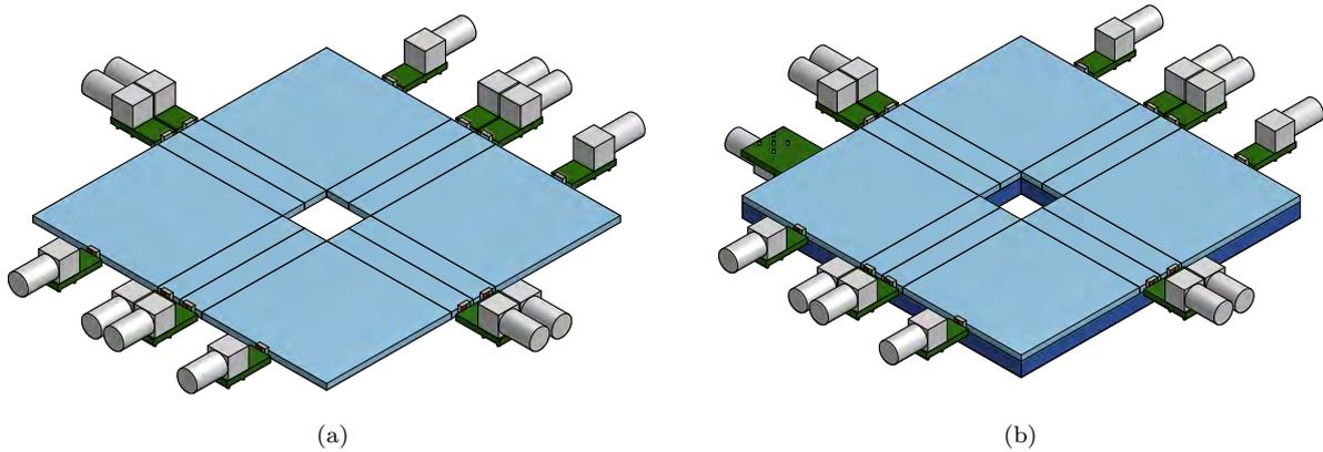
Figure 20: A sketch of the two possible realizations of the muon entrance monitor. (a) A single layer of  $\sim 2$  mm thick scintillators adding up to twelve channels. (b) Additional thicker ( $\sim 5$  mm) 1-channel layer is placed behind the thinner 12-channel layer to improve muon vs. positron discrimination.
