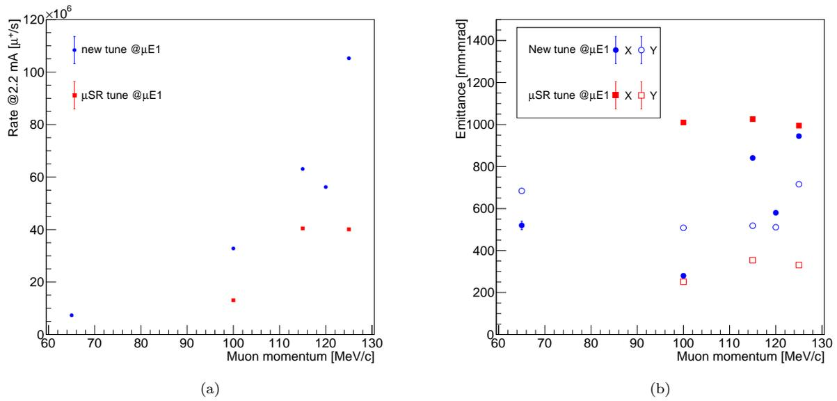
Figure 57: Muon-beam rate (a) and emittance (b) at the  $\mu E1$  beam line for two beam line settings as a function of the muon-beam momentum.
