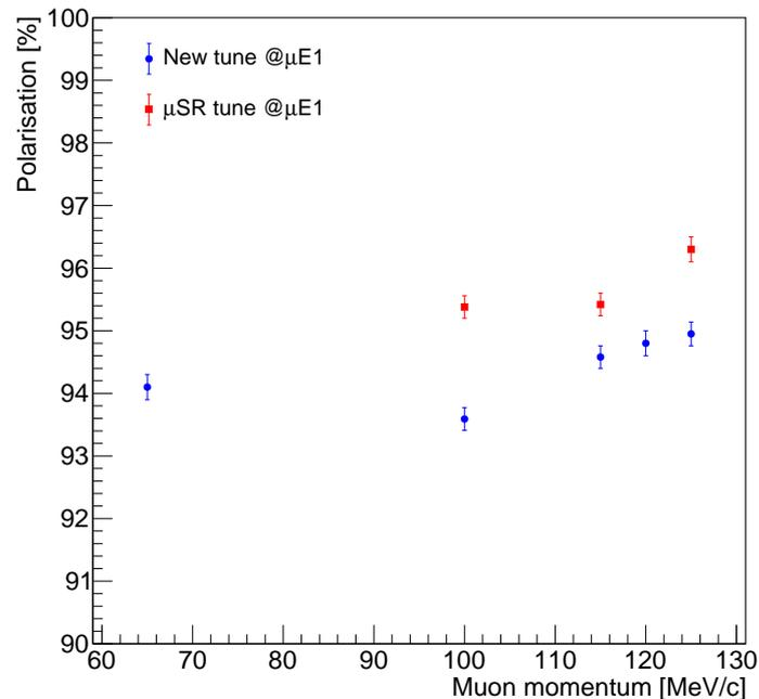
Figure 60: Muon polarization of the  $\mu$ E1 beam line for two beam tunes as a function of the muon-beam momentum.
