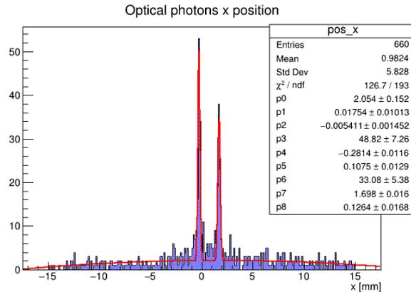
Figure 42: Two particles impinging 2 mm apart on the same ribbon. Using 250  $\mu\text{m}$  fibers and having no pixelation on the readout, the spatial resolution is  $\sigma \approx 100 \mu\text{m}$  (p5 and p8). This value was obtained with a fit to  $pl02+gaus+gaus$  and with a bin width of 125  $\mu\text{m}$  (half a fiber width).
