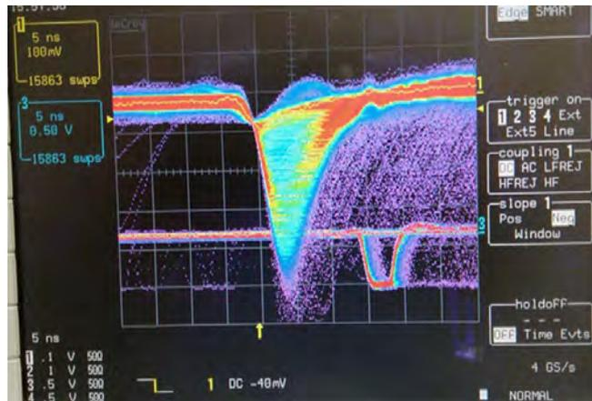
Figure 21: An image demonstrating the discrimination power between muons and positrons. A 2 mm thick plastic scintillator is placed in the beam containing particles with the momentum of 28 MeV/c. Positrons, being minimum-ionizing particles, deposit much less energy than muons, resulting in lower-amplitude pulses.
