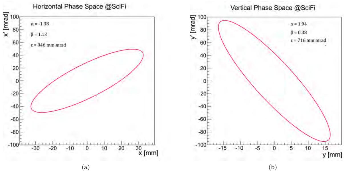
Figure 58: Horizontal (a) and vertical (b)  $1\sigma$  phase space ellipses of 125 MeV/c muon beam at the SciFi beam monitor position at the PSI  $\mu E1$  beamline.
