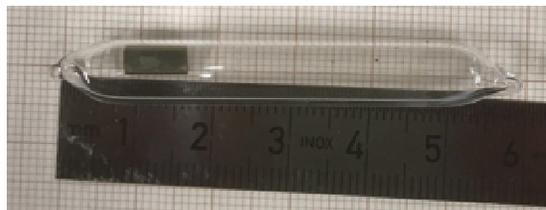
**Figure 3:** Photo of sample No. 4 (irradiated Ti), sealed in a quartz ampoule.
