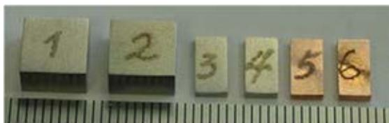
**Figure 1:** Photos of six samples (1-4: Ti; 5&6: Cu) before irradiation in the SINQ at PSI in the frame of the STIP IV material investigation program. Sample No. 4 was used for the half-life determination of  $^{42}\text{Ar}$
