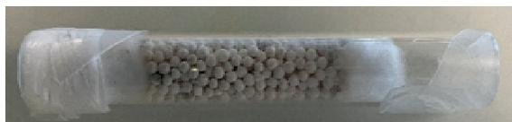
**Figure 2:** The Ag-zeolite trap containing 3 g of Ag-zeolite
