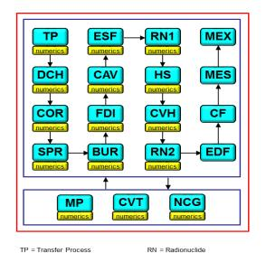
DCH = Decay Heat COR = Core SPR = Containment Spray BUR = Gas Combustion FDI = Fuel Dispersal Interaction CAV = Cavity (MCCI) ESF = Engineered Safety Features
