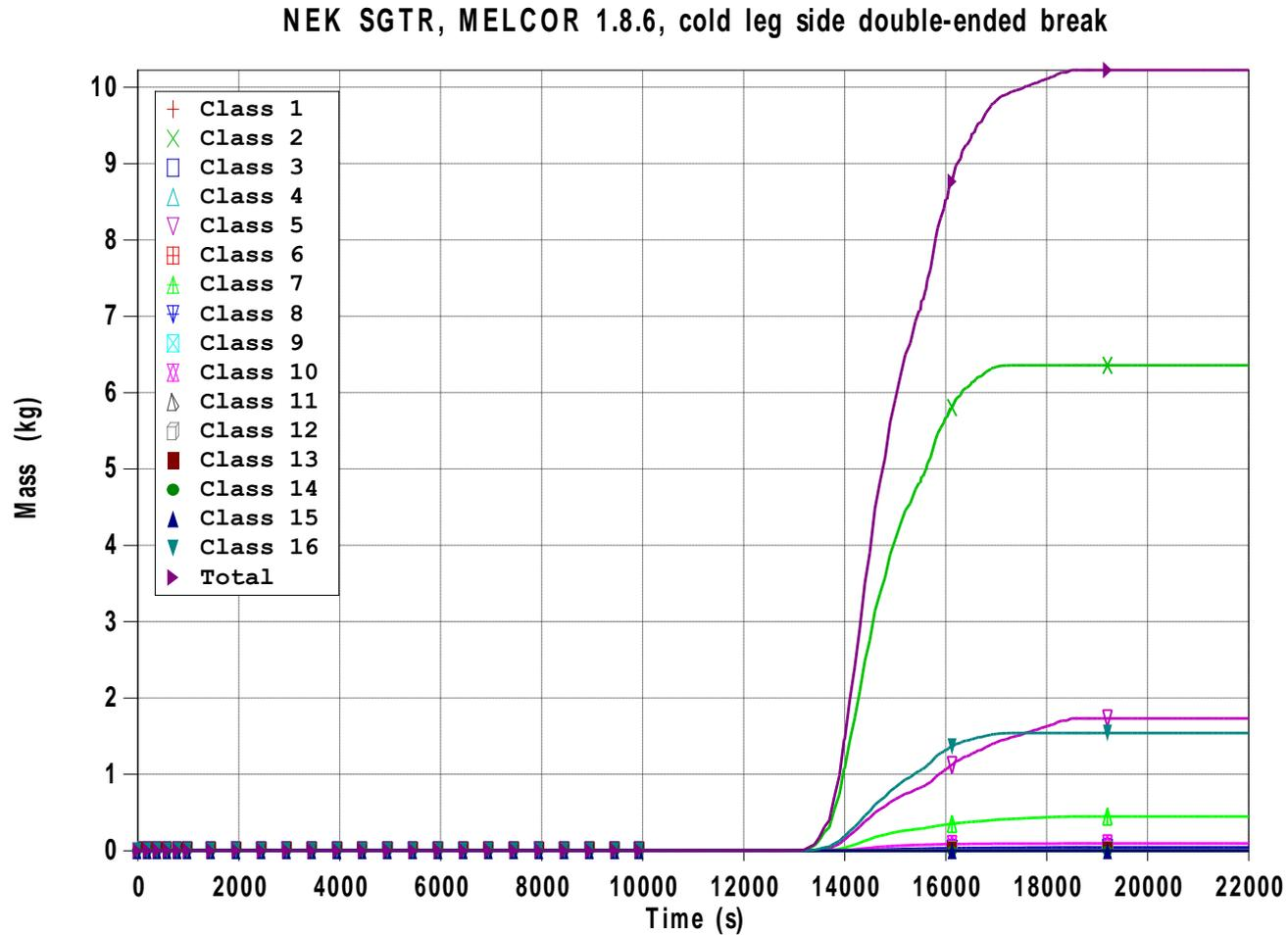
Figure 15: Released radioactive aerosol mass
