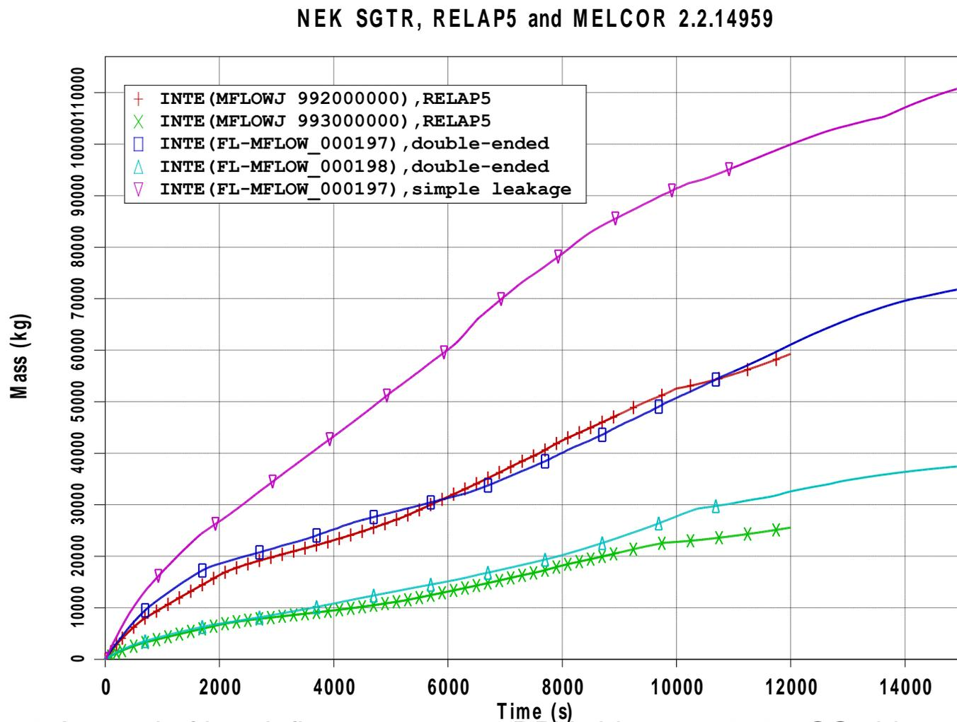
Figure 8: Integral of break flow; 197, 992 – RPV side, 198, 993 – SG side
