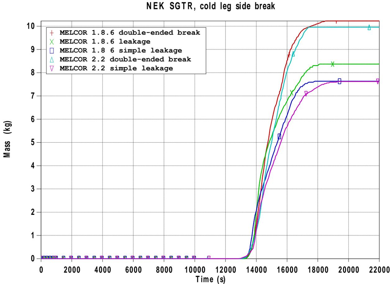
Figure 24: Released radioactive aerosol mass through SG 1 safety valve
