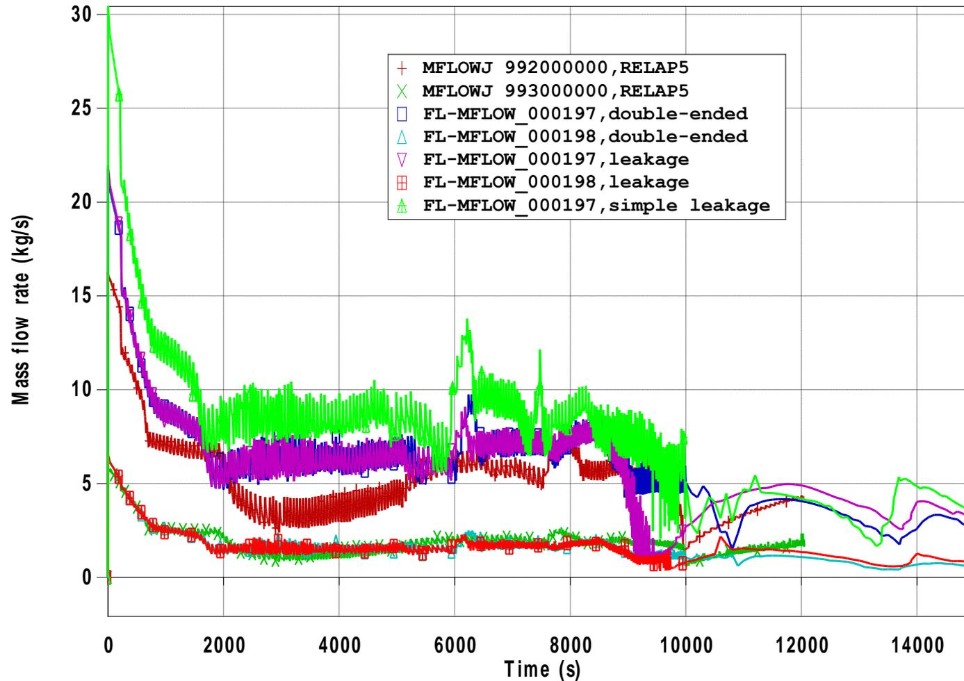
Figure 1: Break mass flow rate; 197, 992 – RC pump side, 198, 993 – hot leg side
