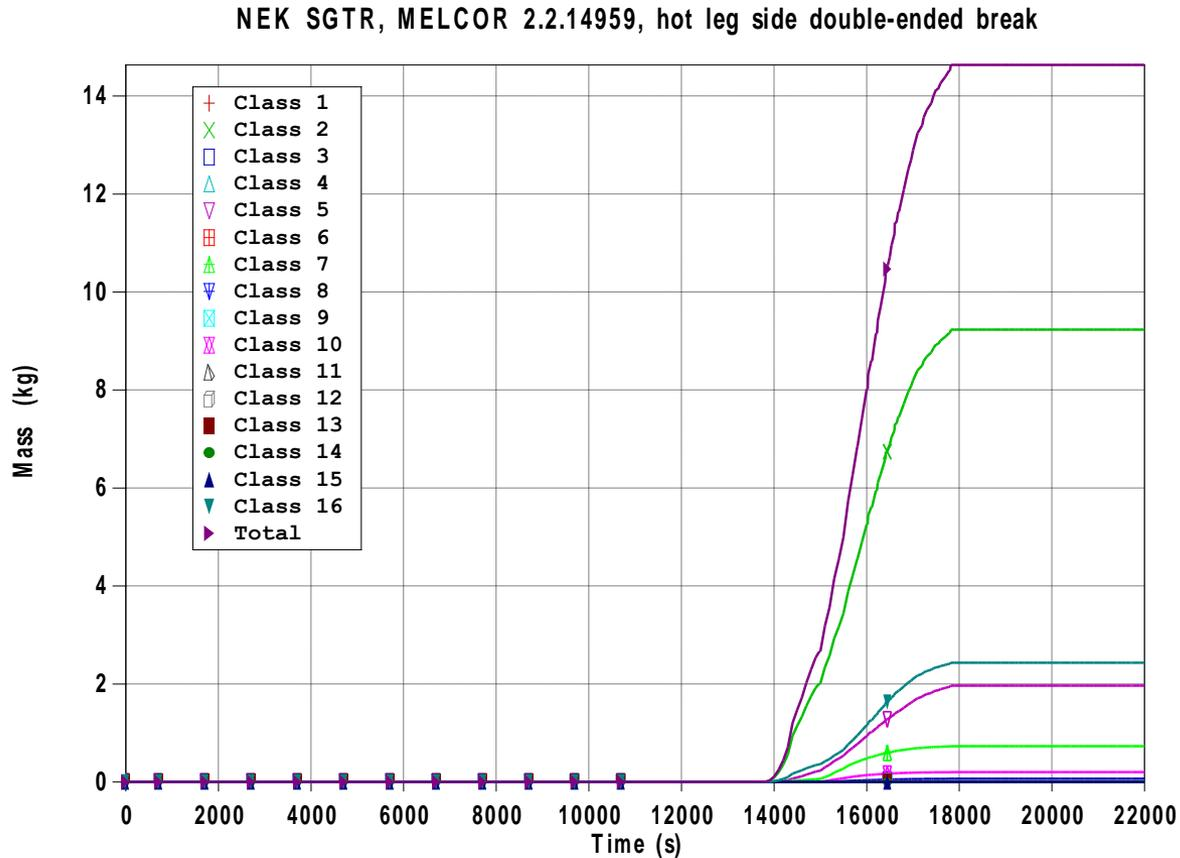
Figure 21: Released radioactive aerosol mass
