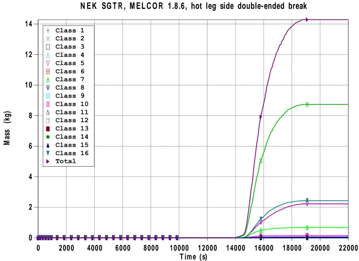
Figure 19: Released radioactive aerosol mass
