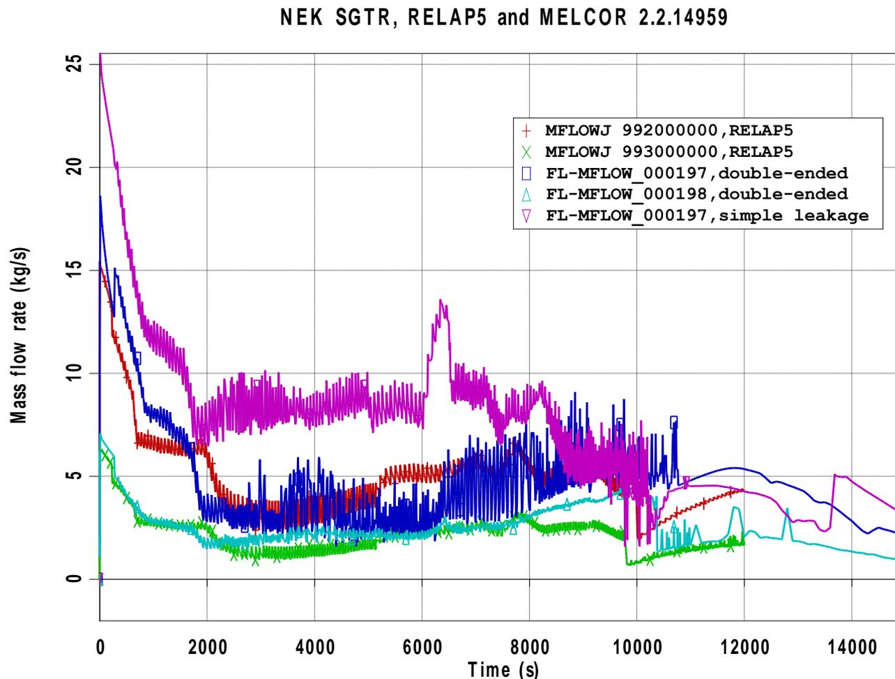
Figure 7: Break mass flow rate; 197, 992 – RPV side, 198, 993 – SG side
