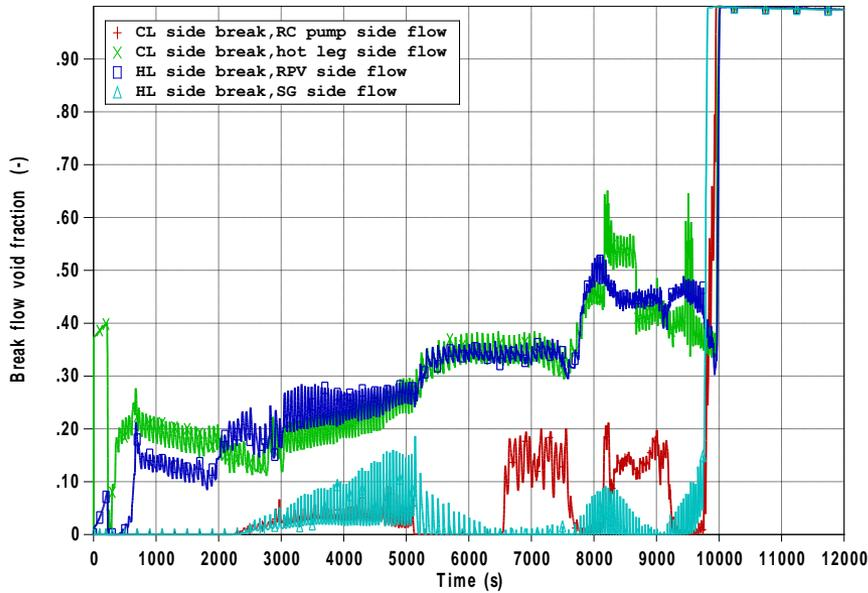
Figure 13: Break flow void fraction, RELAP5
