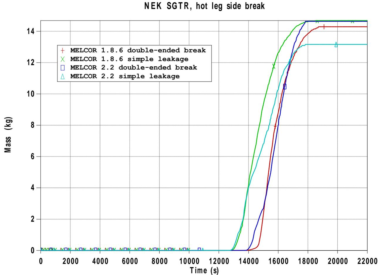
Figure 26: Released radioactive aerosol mass through SG 1 safety valve
