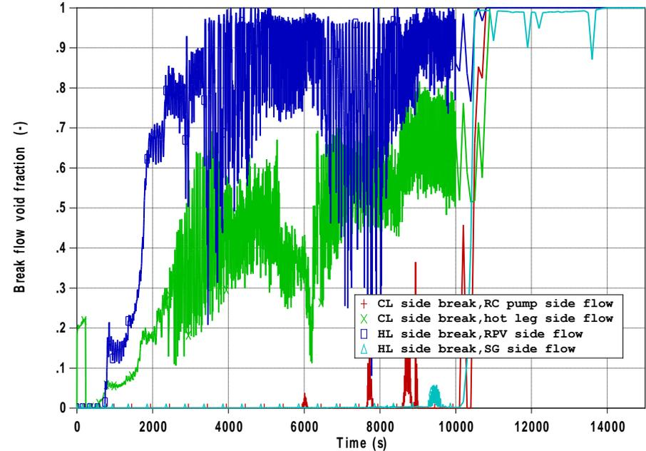
Figure 14: Break flow void fraction, MELCOR 1.8.6
