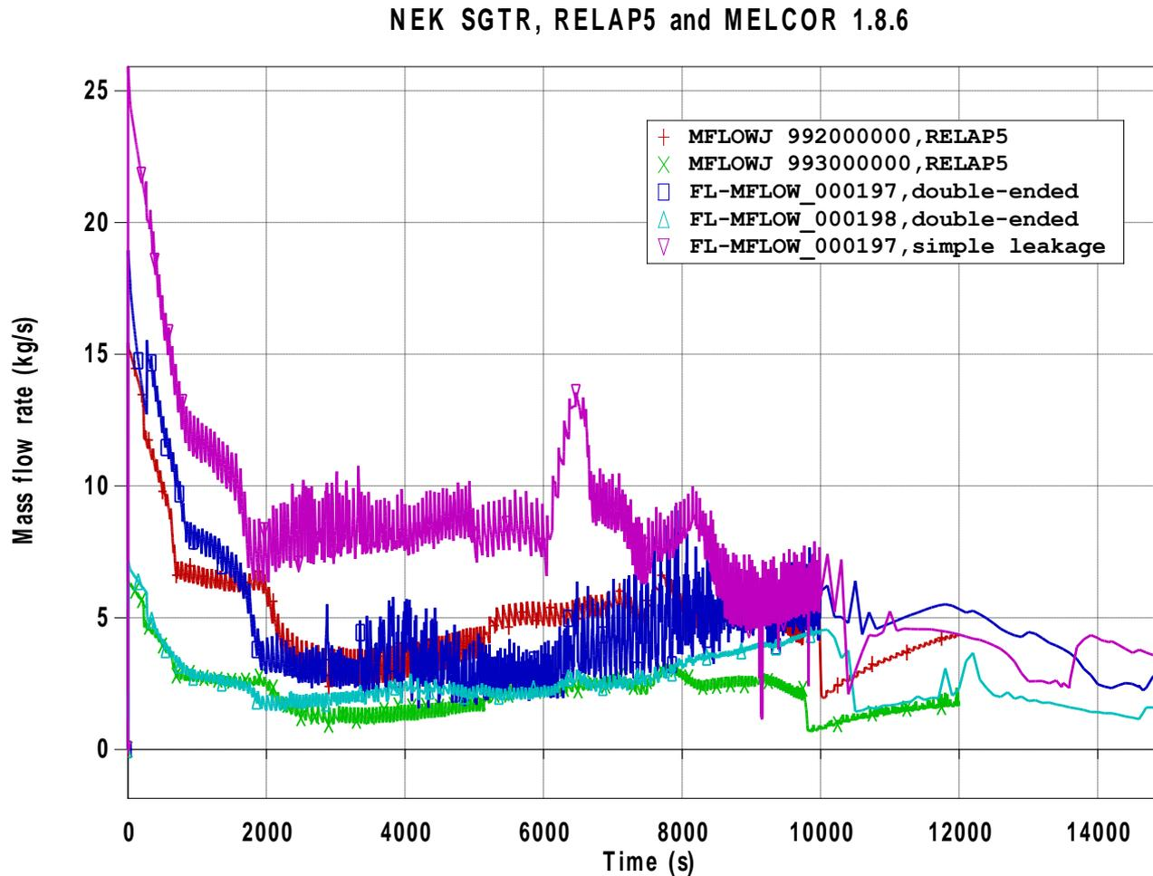
Figure 5: Break mass flow rate; 197, 992 – RPV side, 198, 993 – SG side
