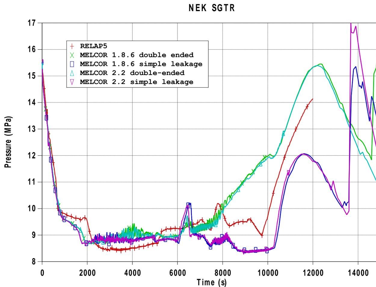
Figure 12: Pressurizer pressure
