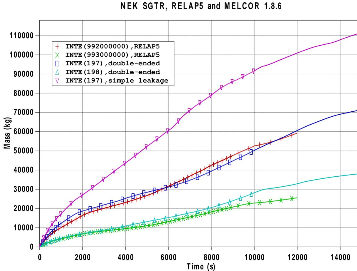
Figure 6: Integral of break flow; 197, 992 – RPV side, 198, 993 – SG side
