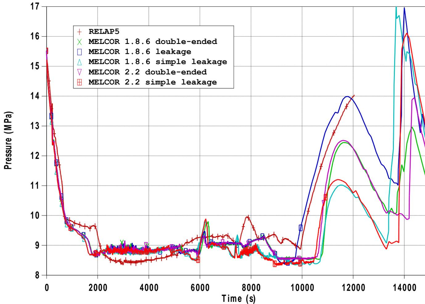
Figure 9: Pressurizer pressure
