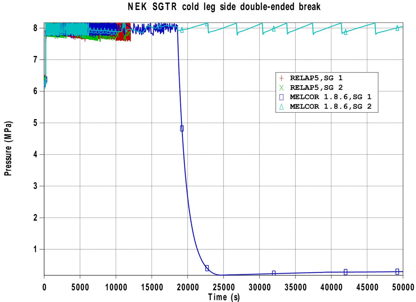
Figure 10: Steam generator pressure
