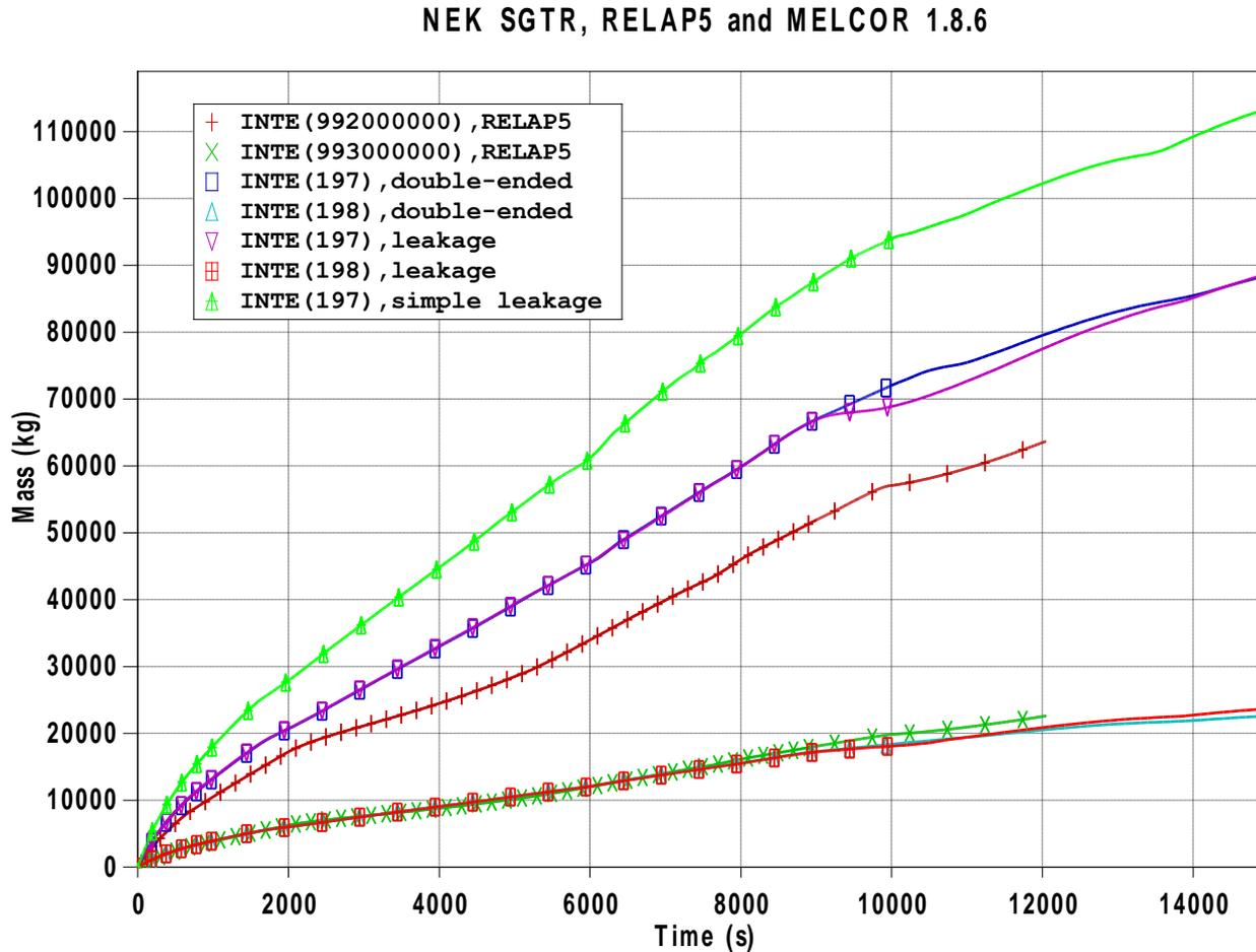
Figure 2: Integral of break flow; 197, 992 – RC pump side, 198, 993 – hot leg side
