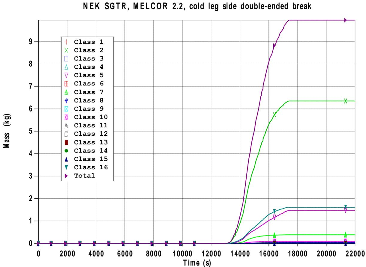
Figure 17: Released radioactive aerosol mass
