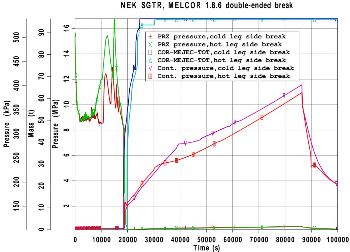
Figure 28: Pressurizer pressure, ejected mass to cavity and containment pressure
