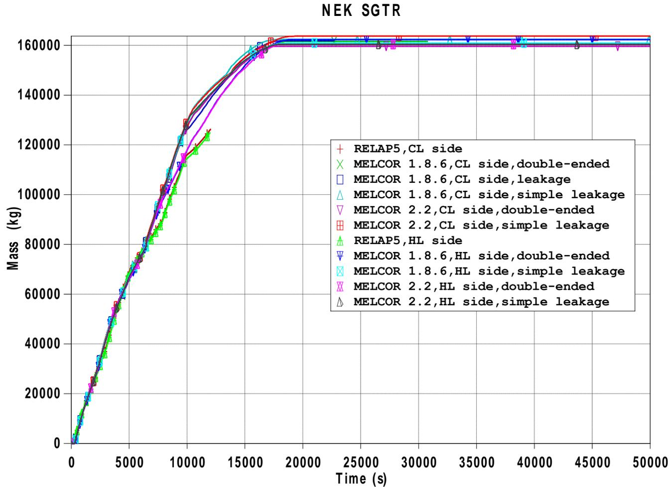
Figure 23: Discharged mass through SG 1 safety valve
