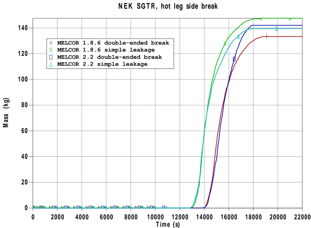
Figure 27: Released radioactive mass through SG 1 safety valve
