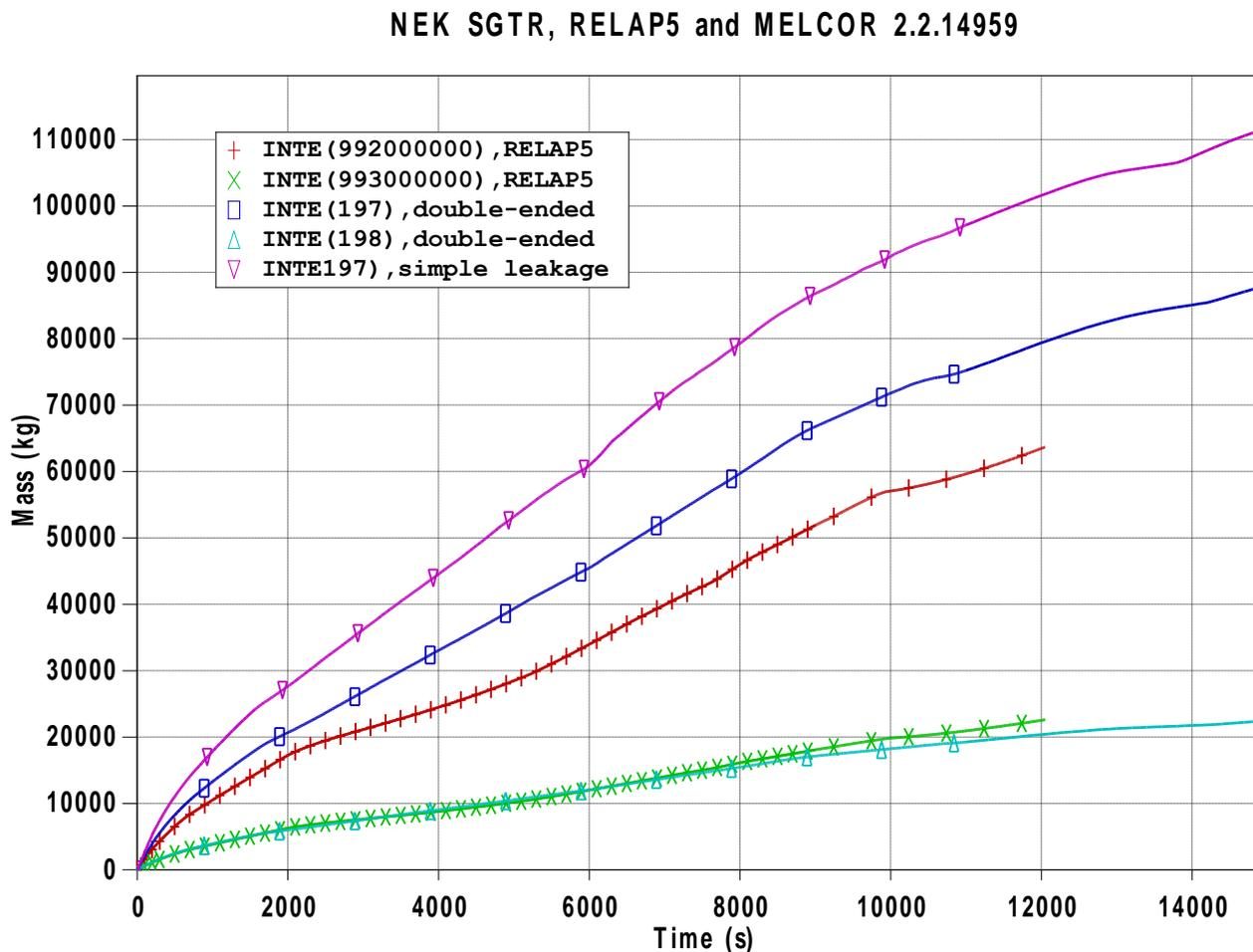
Figure 4: Integral of break flow; 197, 992 – RC pump side, 198, 993 – hot leg side
