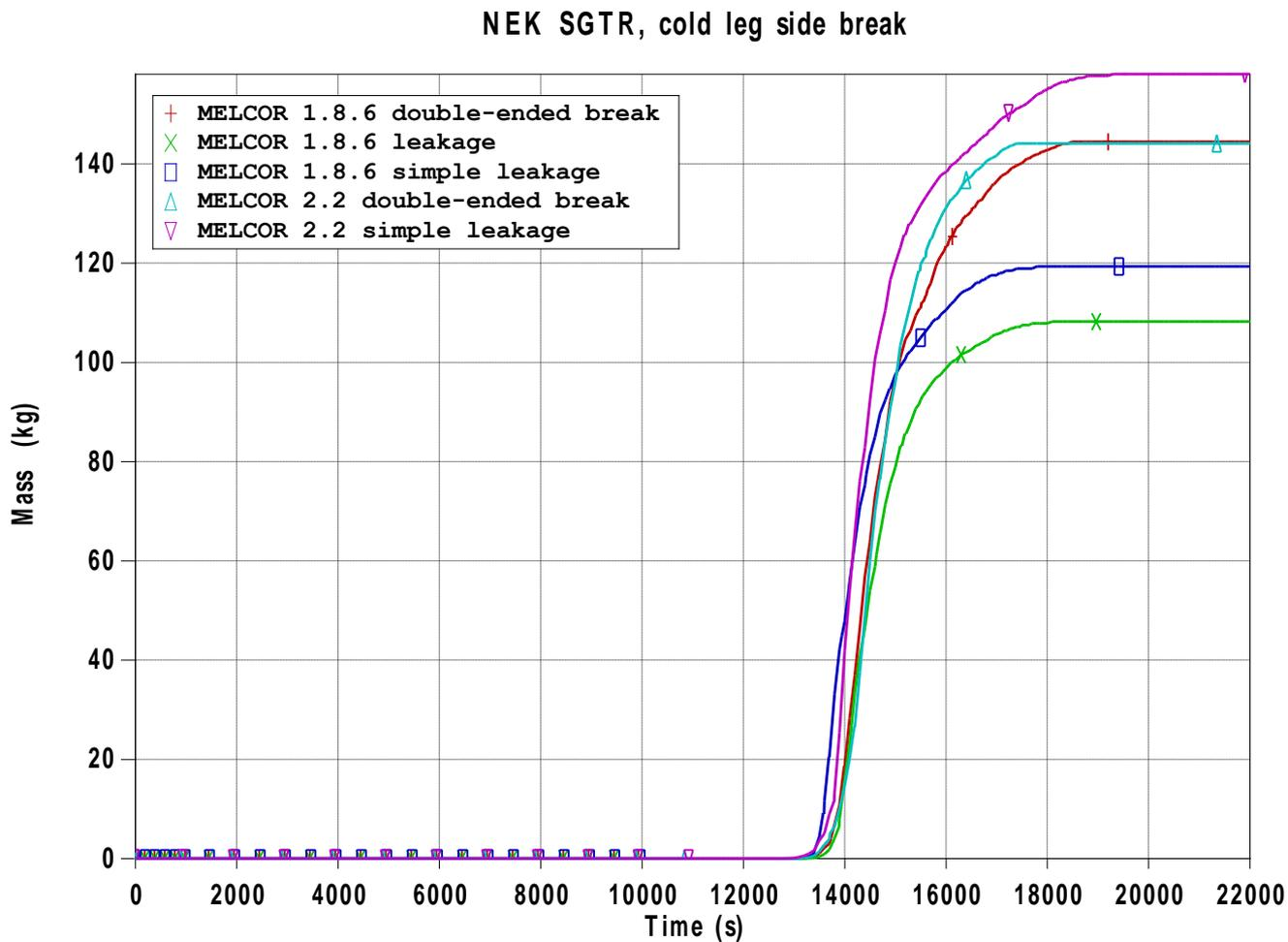
Figure 25: Released radioactive mass through SG 1 safety valve
