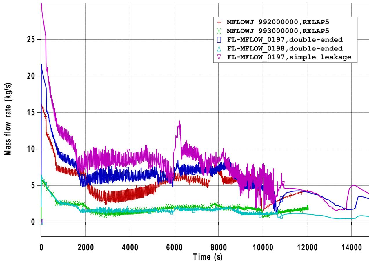
Figure 3: Break mass flow rate; 197, 992 – RC pump side, 198, 993 – hot leg side
