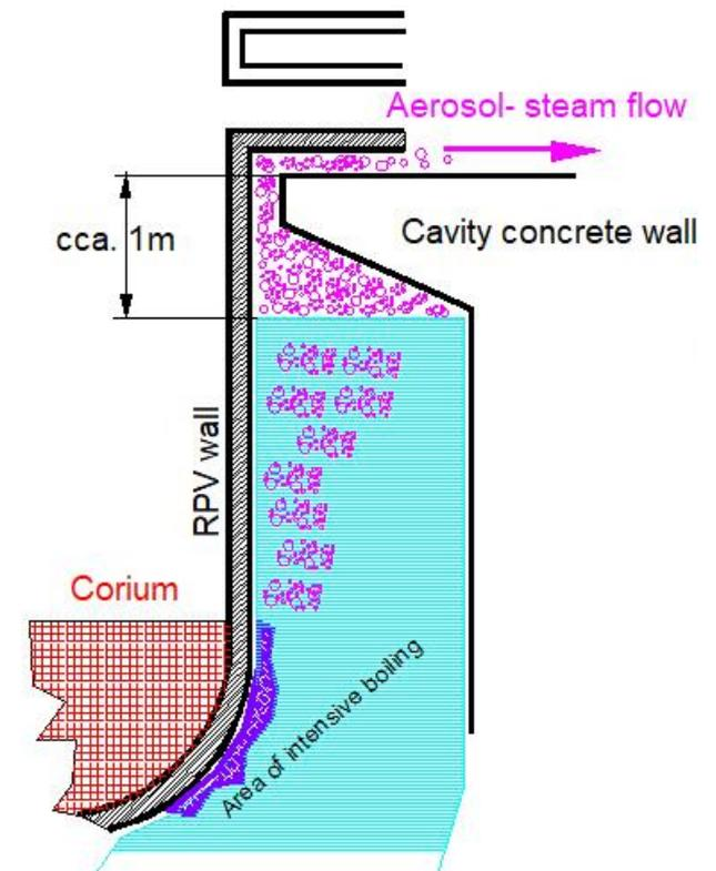
Coolant flowing into the cavity also contains soluble radionuclide chemical compounds – therefore the resuspension of the radionuclides should be expected
