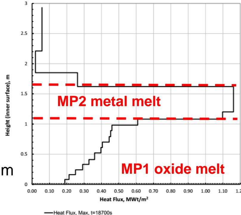
LH external heat flux at maximal value (t=18700s)
