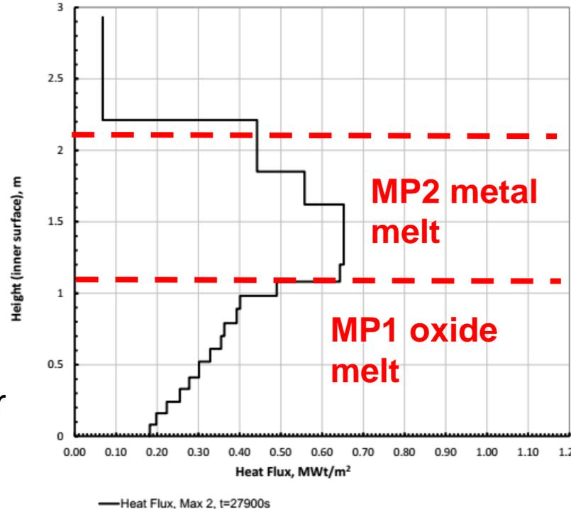
LH external heat flux at maximal value (t=27900s)
