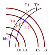
$\begin{array}{l} {\bf T1} \mbox{ - first recurl of particle} \\ {\bf T2} \mbox{ - second recurl of same} \\ {\rm particle} \end{array}$
